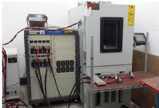
Fig. 1. The devices for battery test and temperature control
