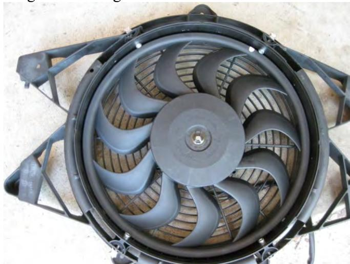
I cut the pig tail off of the OEM fan motor and soldered the connections onto the Hayden fan wires. I used liquid tape for insulation. I pulled the high and low speed relays, shorted the high speed relay then connected the ground wire (center wire on the CRD plug) and touched the high speed wire from the Hayden fan to the two wires. When the fan ran I knew I had the high speed lead from the CRD so I completed my connections.
