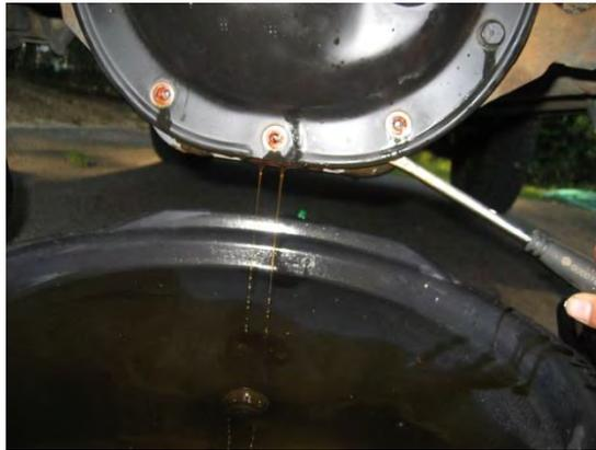
I untightened the screws and used a flat head screw driver to pry open the pan.
