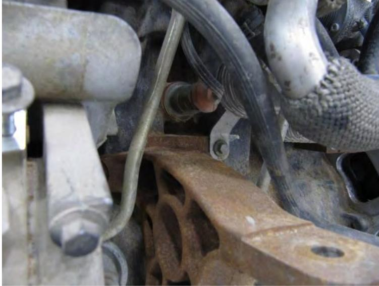
Cam notches aligned - engine in time
