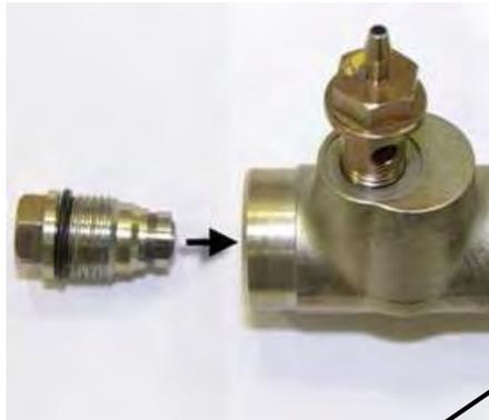
If excessive fuel pressure is generated, the valve opens a fuel return port.
