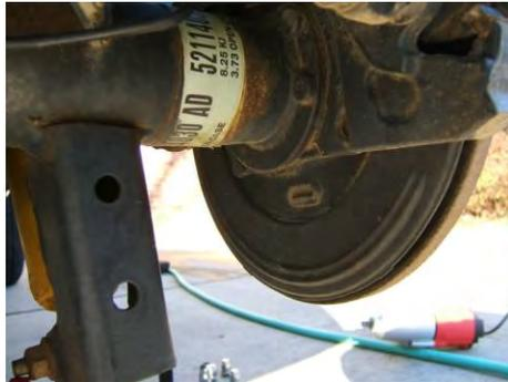
On BOTH sides, the wheel needs to be turned up.. Pull the E-brake handle up 3 clicks. Turn the star wheel until you feel some drag on the rotor but do not tighten it until the rotor will not turn..
