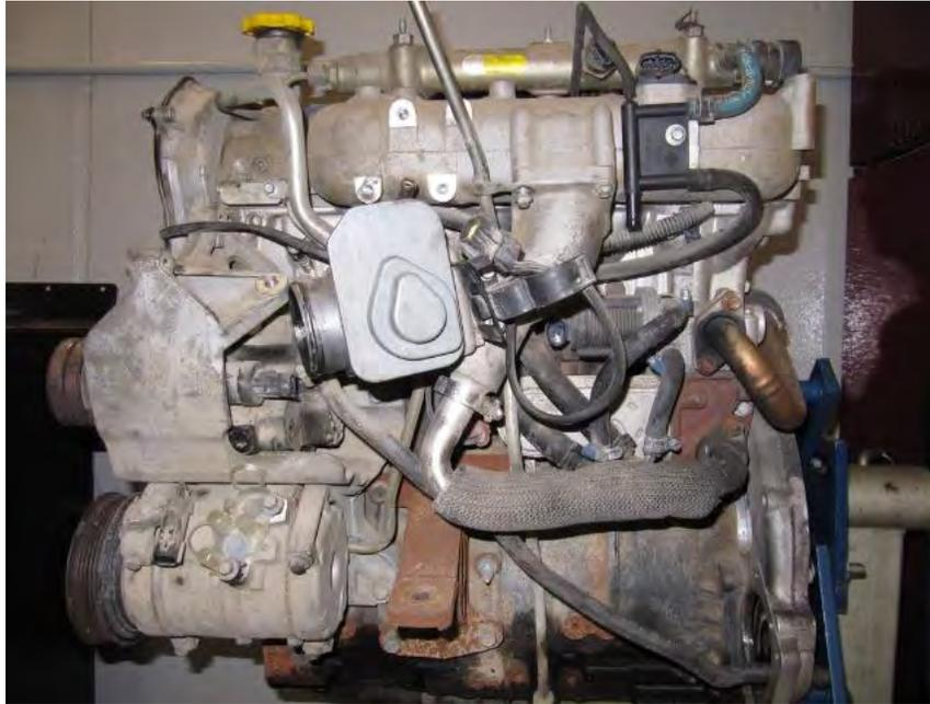
Front view minus alternator and power steering pump
