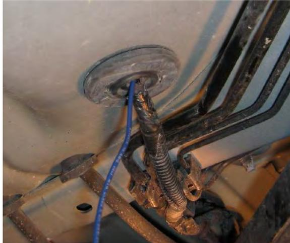
I spliced into the wire and ran the wire to the lift pump through the grommet under the left rear seat. It can be fairly easily accessed by reaching under the carpet and running your hand 'uphill' under the seat.
