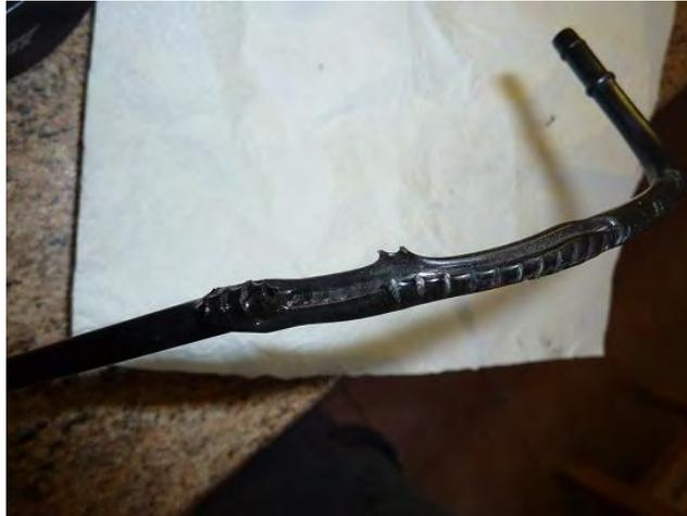
and here is an attempt to show the exact location of where the line was passing and where it was broken. on this pics the coolant tank is unhooked and slightly lifted up:
