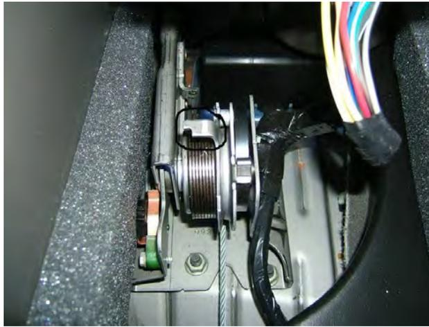
When you pull the ebrake up, that entire thing will move with it. When you hold the tab and let the handle back down, it will stay in place. Max time: 15min
