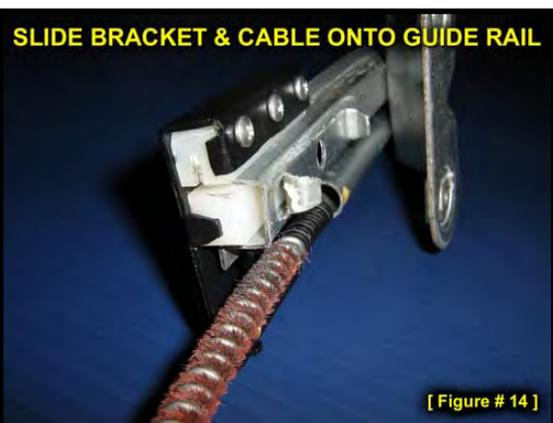
Slide the broken plastic bracket off the guide rail and install the new one as shown in Figure 14. The cable rides in the round channel, the nylon block in the middle of the bracket rides in the square channel and the nylon slot rides on the edge of the guide rail.
