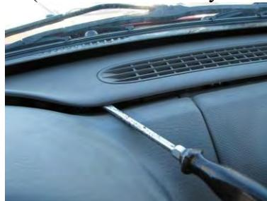
(3) Remove the seven screws and remove the cluster bezel.
