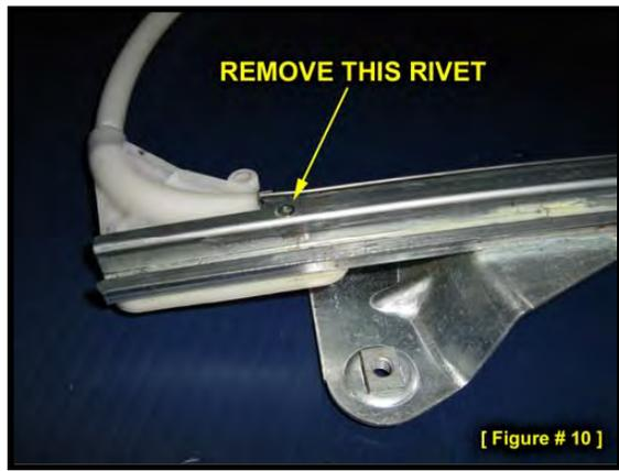
At the top of the guide rail (where the main tube attaches) you will find a small rivet. (Figure 10) Remove the head of this rivet. You can use a drill, grinder, cutoff wheel, Dremel® tool or even a hand file if you have the elbow grease to spare, but whatever method you use, be careful to only remove the head of the rivet itself; do not damage the underlying metal guide rail.
