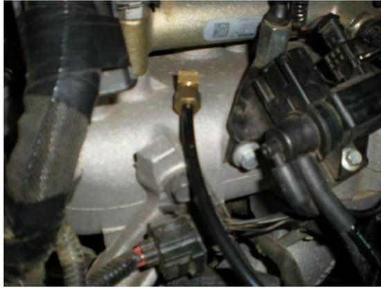
Boost remote sensor mounting location (Note the inline filter that is required to keep soot and crap out of the sensor):
