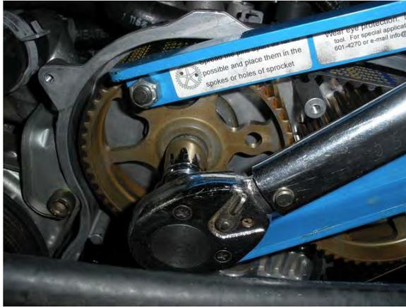
Do not use the locking pins to torque the bolts.
