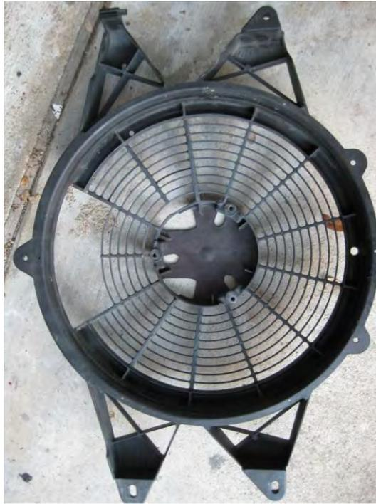
The fan (front of vehicle side). Notice the three lugs for mounting the fan
