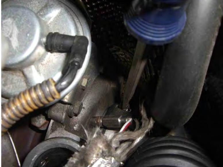
4. Now you have access to the top engine mount retention nut. Remove this using an 18mm socket, with a universal joint and 24" of extension.
