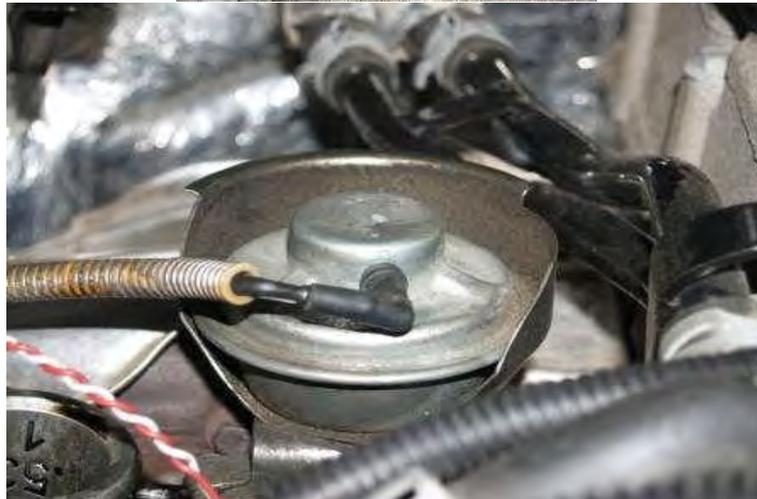
12. Loosen marmon ("V" clamp) flange that holds the exhaust downpipe to the rear of the turbo using a 10mm socket. Completely remove the nut so the marmon flange can slip off the exhaust pipe.
