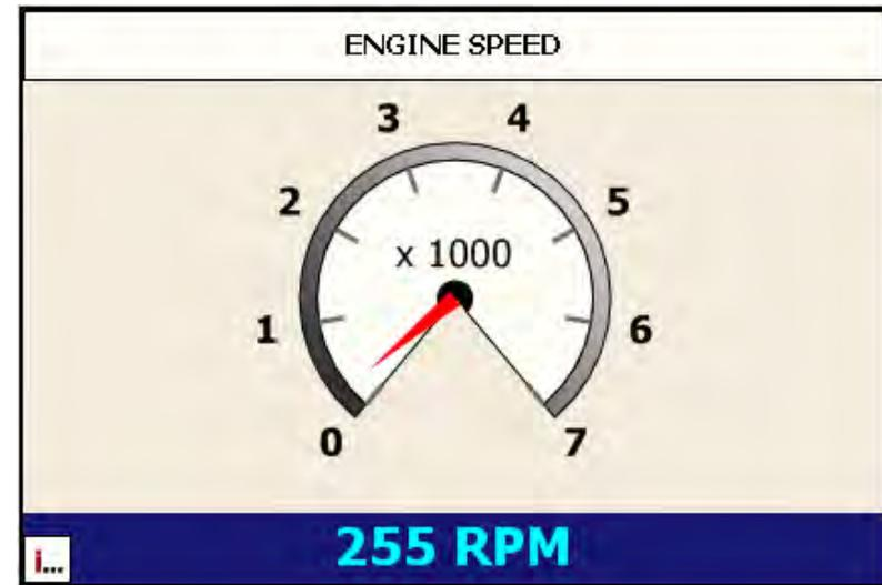
Typical minimum '**manufacturer specified**' value during engine cranking:
