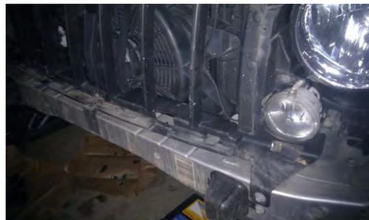
Step 4: I did not insert the cooler like most of the people, from the top. The B&M 70273 is too thick to go through the top. So I cut a hard black plastic bar, the second one from the right hand side. I cut it slanted that pressure will keep it place afterward and that I could easily glue it back. That gives plenty enough space to insert the cooler and put it in place. It went in horizontally, I had then to work to place vertical.
