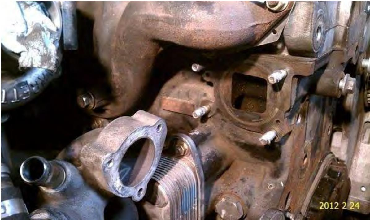
The three bolts on back, securing the manifold to the pump, are 8mm - and a 1/4 inch ratchet, universal joint, and 8mm 6-point socket worked well enough to pull them. Used a short extension to get a good angle on the top-rear bolt. Took a little juggling to get the right angles. I'd left the hose to the oil cooler connected on the bottom - if I'd pulled it the bottom bolt would've been easier to reach.
