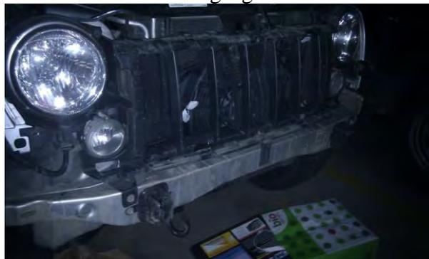
STEP 3: This is where I choose to place my cooler. I wanted the cooler to be fully exposed to the fresh air and to keep clear from blocking the radiator behind.
