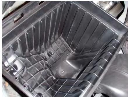
The scratched up area is where the casting process for the plastic left a little "lip" inside the duct... I scraped it off with a knife, then sanded it smooth.
