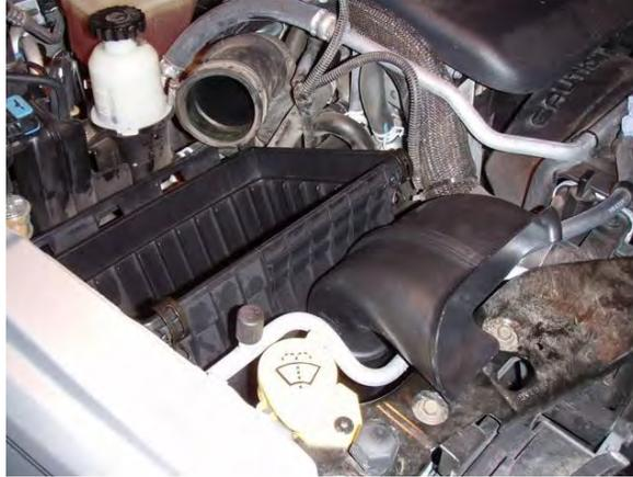
And here it is with the rain shield installed (note the stainless still screw and nylon lock nut holding it on):
