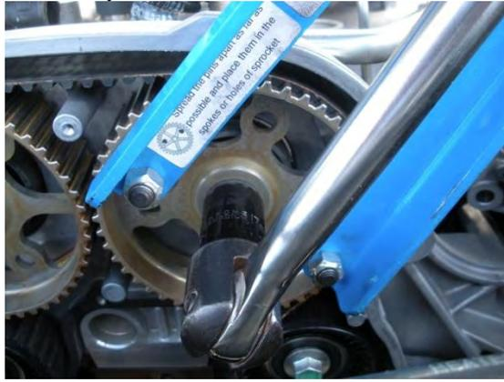
Now remove the bolt on the tensioner and the tensioner then the timing belt and the cam sprockets and the two idler pulleys **TURN THEM CLOCKWISE TO REMOVE THEM.** **NOTE: the next picture shows the cam ends with the sprockets removed.** Notice the 2 notches in those cam ends that face each other with the engine in time, same notches in same position show in a picture from Eugene Buford who confirms that his picture was taken with the 2 cam pins and the flywheel pin installed.
