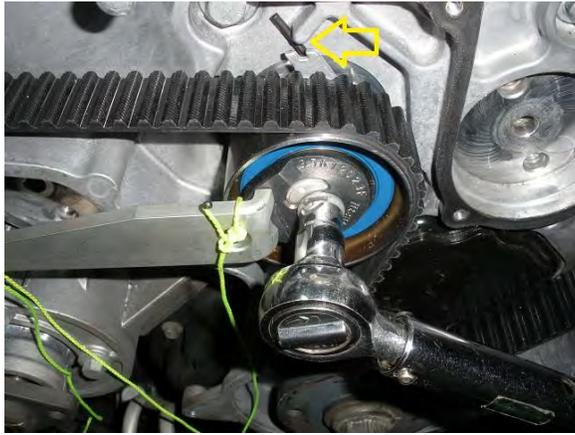
Then torque the cam sprockets...
