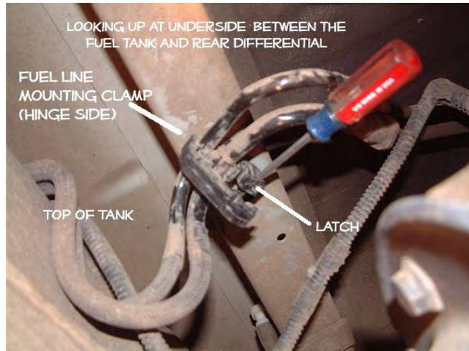
But if the hanger was hard, I found the fuel line "quick disconnects" anything but quick. The tiny "button," flush with the connector, must be depressed fully as shown in this image.
