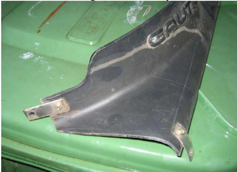
Top view of cut edge of shroud from front of vehicle
