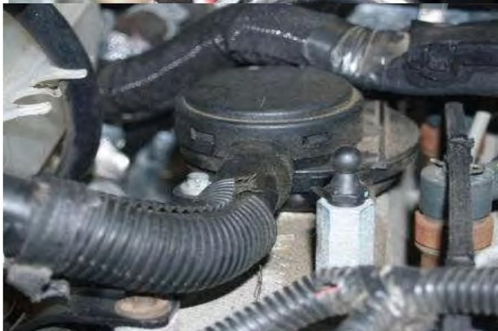
6. Remove two 10mm nuts holding the coolant bottle to the firewall.
