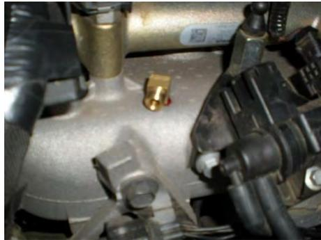
Boost line installed to sensor:
