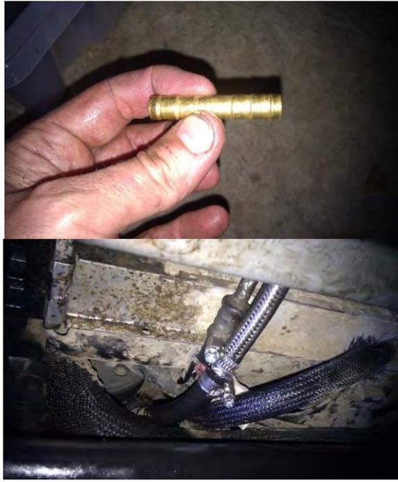
STEP 11: I decided to connect the inflow to the lower inlet of the cooler. My logic is that the oil being pushed up in the cooler has a tendency to spread in all the cooler circuit and give a better cooling effect... seems to work out well so far.
