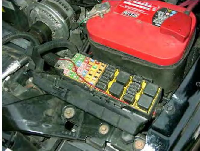
This is the wiring connection to number 5 terminal of the relay and battery ground. I had to add one foot of wiring each because the wire on the pump is short.
