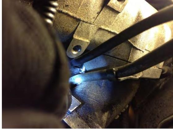
Try sticking the hand in between the elbow and cylinder head, you can use that hand to drive the socket to the bolt while the other hand to untie the bolt with the socket and flex head drive.
