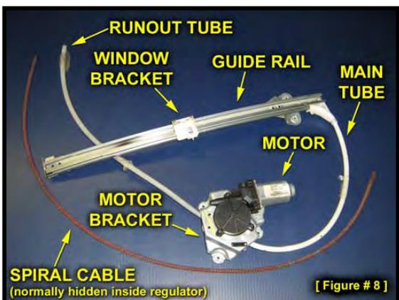
*Figure 8* shows what the window regulator assembly looks like when removed from the vehicle. Various parts of the regulator are labeled for your reference.
