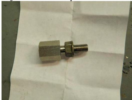
I drilled the manifold with a 5/64 bit, put some pipe dope on the threads and installed the boost bolt. I snugged the nut downward to keep it tight. The McNally MAP sensor is installed with some pipe tape. I used wire conduit for everything for a factory look. You can hardly pick out the new sensors in the engine bay.
