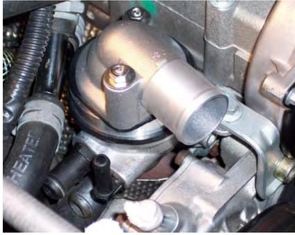
Lightly coat the new gasket (part #05066806AA, \$2-\$3) with high temperature grease (silicone or white lithium) to keep it from sticking again. Bolt the thermostat housing to the engine block and torque the bolts to 20 ft-lbs (the longer of the 2 short bolts is used here). Replace the bracket and torque the bolt on top to 20 ft-lbs and the 8mm Allen bolt (to the viscous heater) to 25 ft-lbs. This is the modified thermostat. The actual new thermostat part number is 05142601AA.
