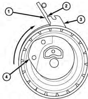
Fig. 176 TIMING BELT TENSIONER ALIGNMENT
