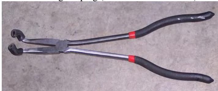
Long pliers are required to get at these. The picture shows hose pliers with vacuum hose for protection.
