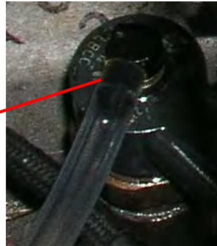
There should **not** normally be any fuel collected in receptacles during engine cranking.
