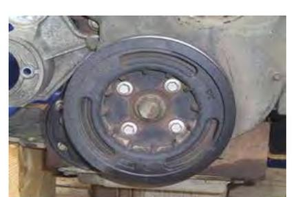
6. Remove the front timing cover (17-7mm bolts)
