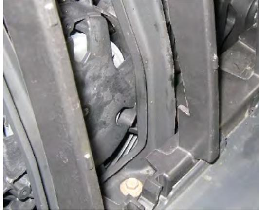
I notched one of the posts to allow the cooler to fit flush against it.
