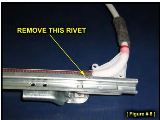
At the top of the guide rail (where the main tube attaches) you will find a small rivet. (*Figure 8*) Remove the head of this rivet. You can use a drill, grinder, cutoff wheel, Dremel® tool or even a hand file if you have the elbow grease to spare, but whatever method you use, be careful to only remove the head of the rivet itself; do not damage the underlying metal guide rail.
