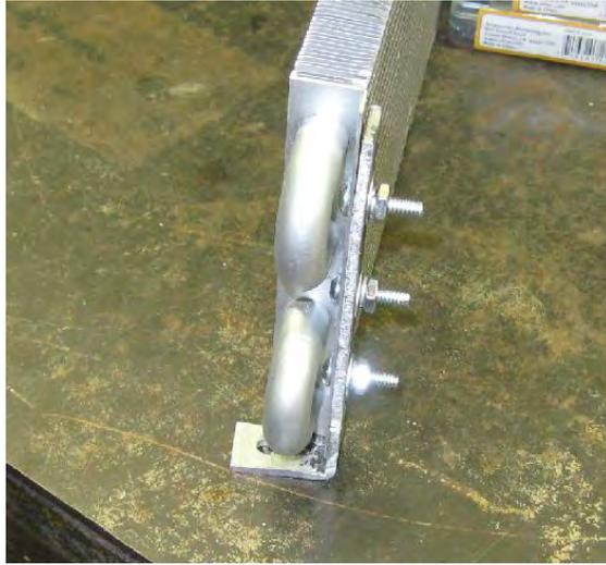
An easily fabricated aluminum L-bracket.
