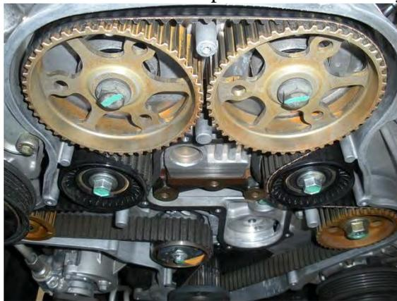
Make sure the fuel pump is aligned with the timing marks then using a pin wrench adjust the tensioner so the spring lines up with the notch. If you have a pin wrench from a VW TDI it will fit your jeep.
