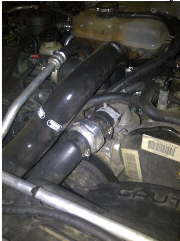
**In-line thermostat install per secondechomatt on LOST**
