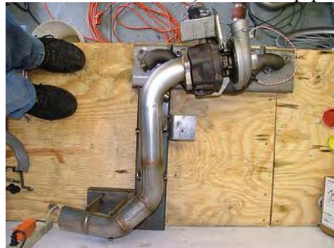
Not seen is the support bracket for the turbocharger.
