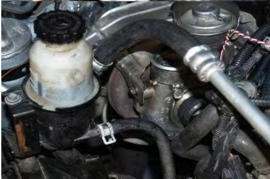
10. Spray penetrating oil (WD-40 or equivalent) on the four nuts/studs holding the turbo to the exhaust manifold.
