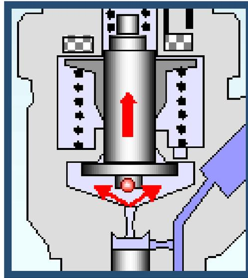
Maximum stroke of solenoid valve:
