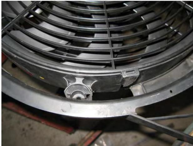
Here is the Haden 3814 mounted in the OEM fan shroud as viewed from the front of the vehicle. NOTE 1) the Hayden fan spins clockwise and 2) the finger guard seen here is on the engine side and cannot be removed as it's a functional part of the Hayden fan shroud. I used some hardware supplied by Hayden and mounted the fan by drilling through the bolt lugs and the OEM shroud.
