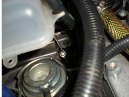
Run the sensor wires through the firewall, and I thought the obvious place was what I assume to be the clutch grommet (which is unused on my automatic).
