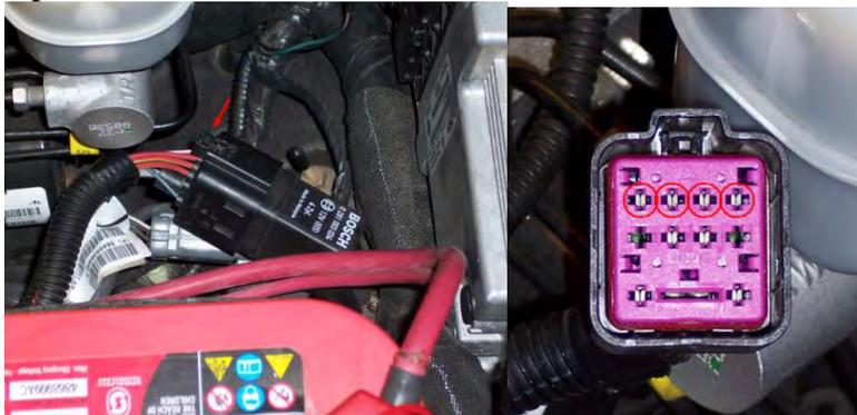
Connect one lead of the ohm meter to the negative battery terminal and measure at the indicated terminals. Unless the wiring harness is on backwards (can happen), the glow plugs should be 4-3-2-1 (left to right).
