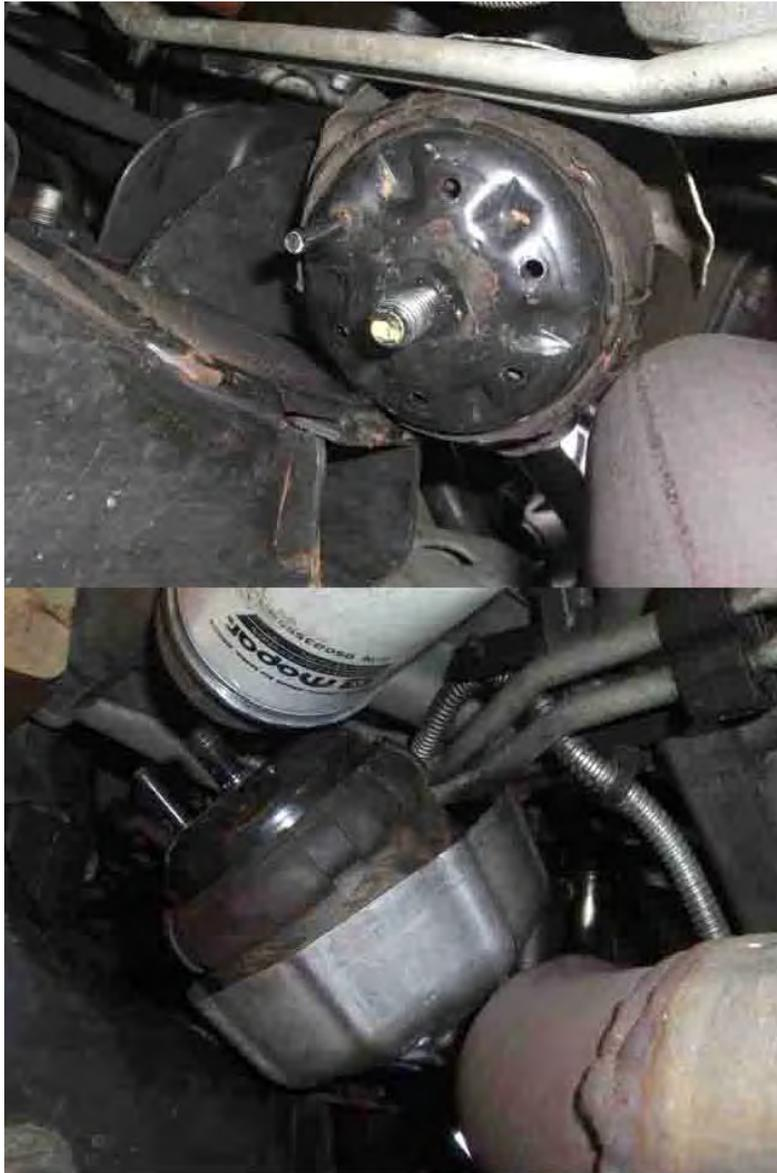
9. The engine mount heat shield needs to be removed and installed on the new mount prior to reassembly.
