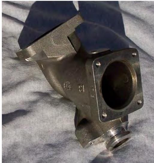
Clean up the elbow and intake manifold that is accessible. The new gasket to the manifold is #05066946AA (my dealer cost, Aug. 2012, \$14.45!). The 8mm M6 (10.9) bolts should be torqued to 6 ft-lbs
