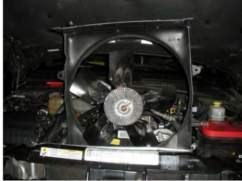
remove the serpentine belt and Tensioner Pulley unbolt the alternator (**NOTE - makes it easier to get at driver's side cam locking point**) you can leave the wires on just move aside so you can install the locking pin. remove the idler pulleys **TURN THEM CLOCKWISE TO GET THEM OFF**. Remove the crankshaft pulley and the fan pulley; remember there is a hidden bolt behind the pulley and the power steering pump pulley.
