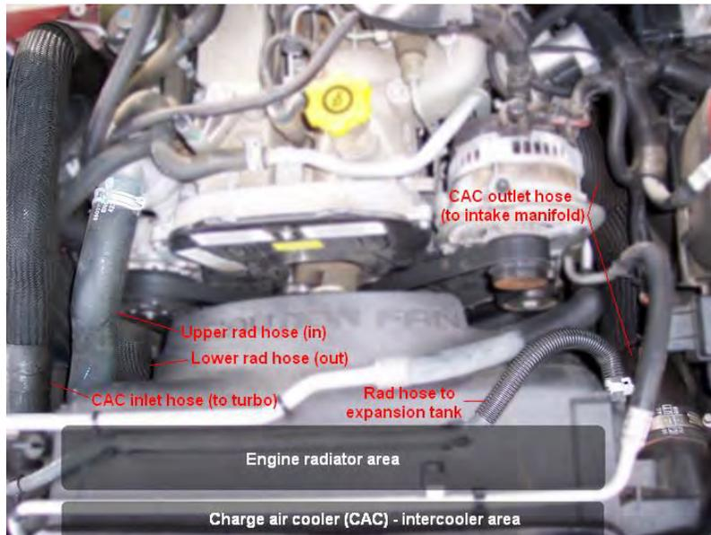
Remove the engine cover. Disconnect the cac inlet hose at the intercooler (8mm socket). Disconnect the upper radiator hose from the thermostat.
