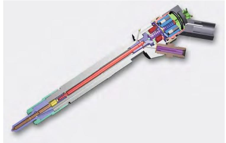
The fuel injectors are controlled by either a solenoid or piezo actuator.
