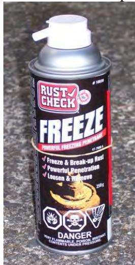
The glow plugs can be removed with a 10mm deep socket and a 6 inch wobble extension. Put a rag around the plug and use a good penetrating oil/freeze spray to help when "cracking" it loose. Heat expansion, rust and
