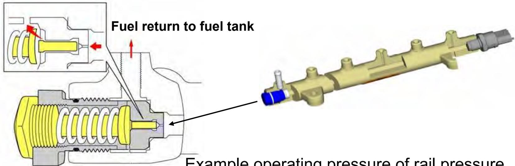
Example operating pressure of rail pressure limiter valve (Denso HP3 system):
