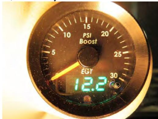
So far the highest egt I saw just fooling around a little was 715F. Normal driving is like 500F. Highest boost was 21psi with the GDE hot tune.
