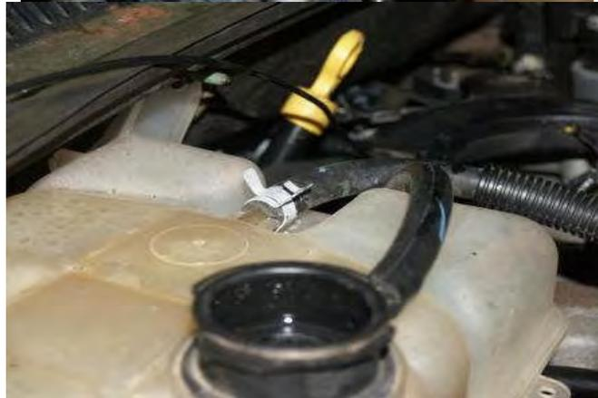
8. Cut off the two plastic tabs on the bottom of the coolant bottle.
