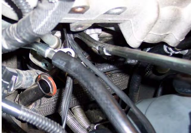
For re-install, the EGR pipe should have high temperature RTV Silicone re-applied (Permatex Red, or Orange as a 2nd choice).
