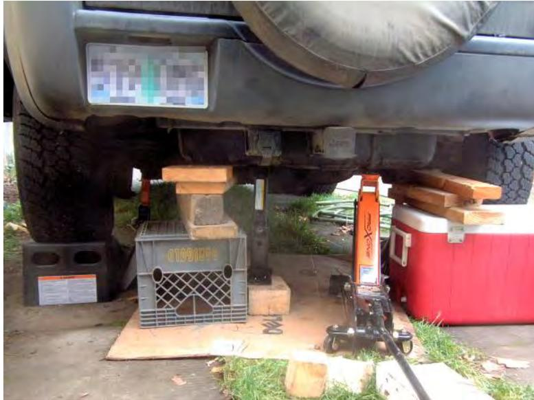
This was tedious work. The more so because I thought I might break the plastic fuel lines, so I didn't put them on until the tank was half way up. A difficult task in tight space. Reconnect and re-hang:: Filler Hose, Vent Hose, Fuel Lines, Fuel Pump, VSS.
