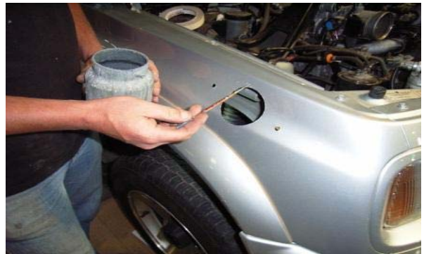
3.28 Paint ALL raw metal surfaces with Zinc rich primer (4 snorkel fixing holes, 1 air intake hole, 2 "A" pillar holes)
