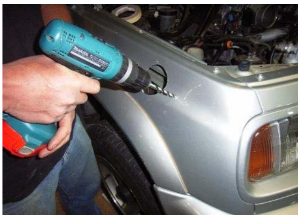
3.18 Then drill the four fixation holes at 10mm
