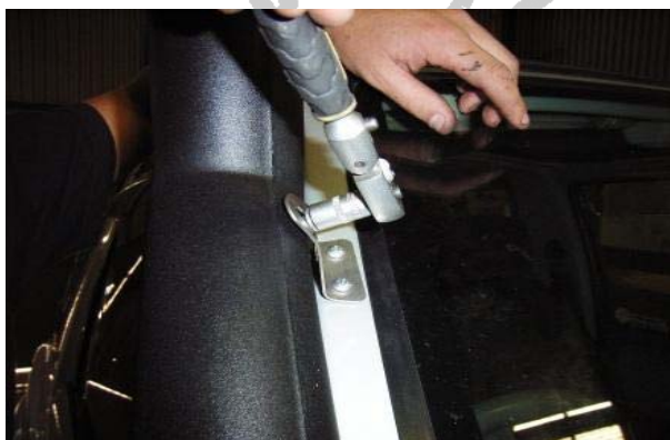
3.50 Secure the snorkel to the bracket with the washer SP023 and the bolt SP024 Do not over tighten fixings to avoid damage to the snorkel
