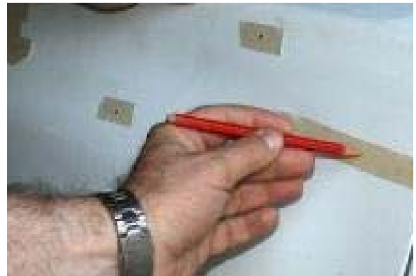
3.14 Cover the areas to be drilled with masking tape
