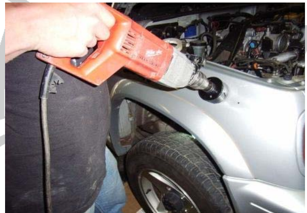
3.17 Using the hole saw, drill at LOW SPEED a 76mm hole
