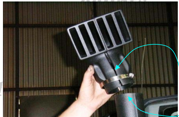
3.51 Slide the hose clamp SP142 on the air ram SP064 then slide it on the snorkel SP093
