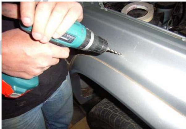
3.16 Pre-drill all holes at 5mm (4 snorkel mounting holes, 1 hole saw hole)
