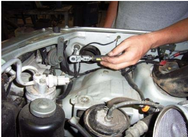
3.5 Unbolt the factory air box ducting...
