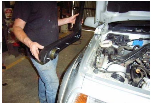
3.30 Mount the bracket SP113 with the screws SP029
