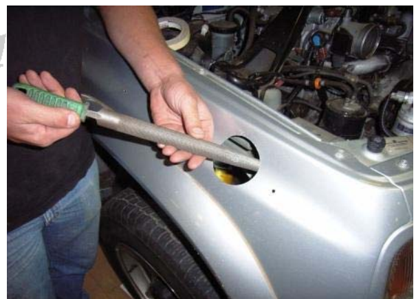
3.19 File to suit snorkel tube and to remove any burr
