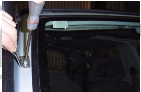
3.30 Mount the bracket SP113 with the screws SP029
