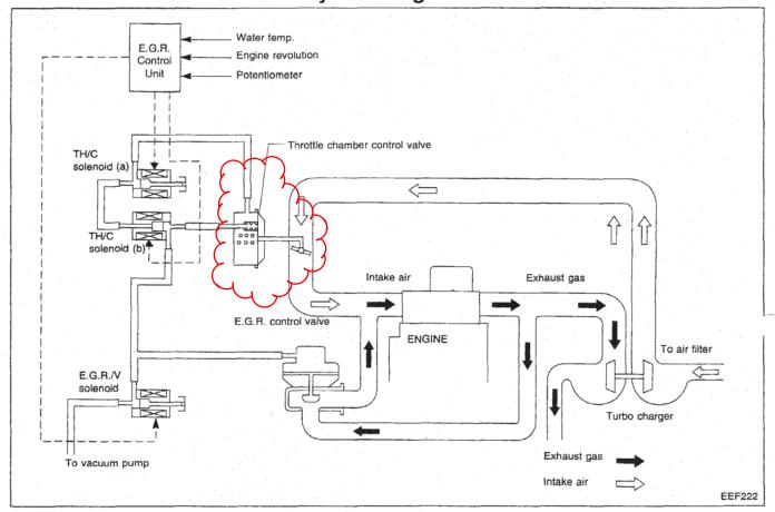
The E.G.R. system is designed to control the formation of NOx emission by recirculating the exhaust gas into the intake manifold passage through the E.G.R. control valve.
