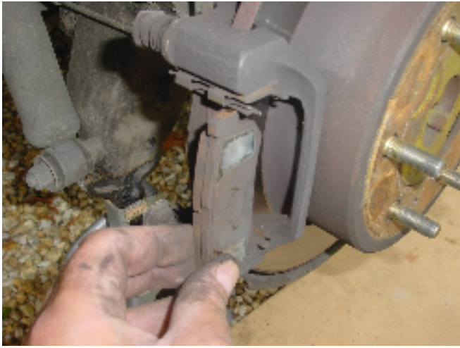
Take of the pads. The one with the wear indicator sits at the inner side.
