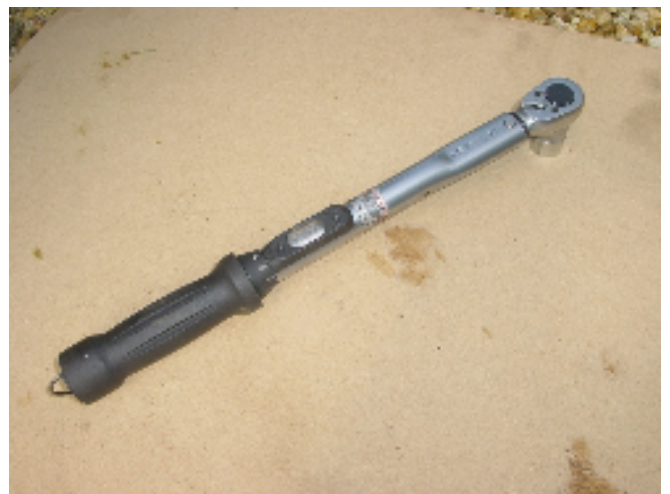
For this mountings I always use a torque wrench.
