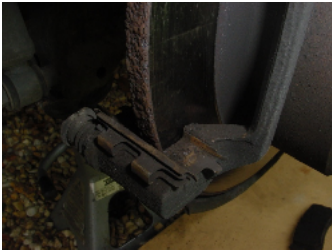
View on the dirty wear shims. Top and bottom are the same.
