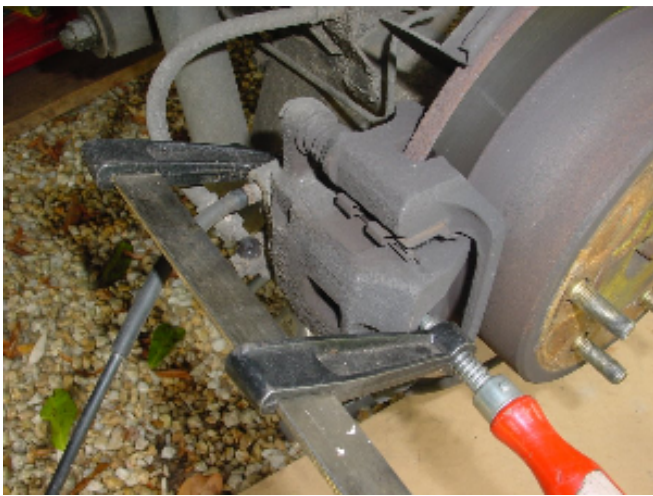
Open the bleeding screw and push the caliper in with a clamp.
