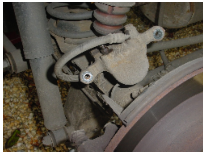
Lay the caliper on the axle. Beware that the hose not twist.
