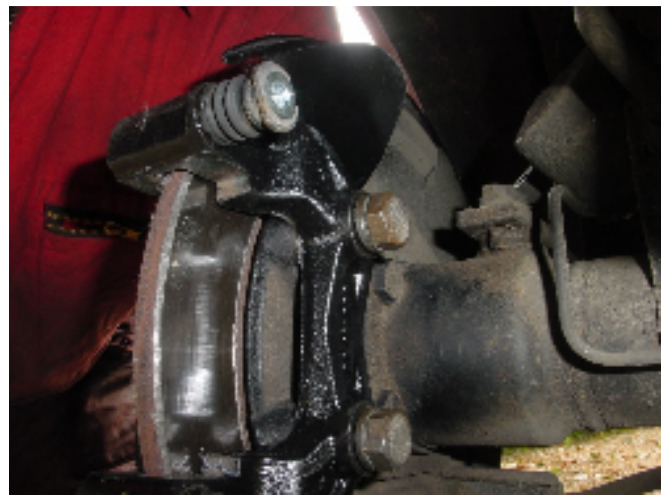
Tight the two bolts with the right torque.
