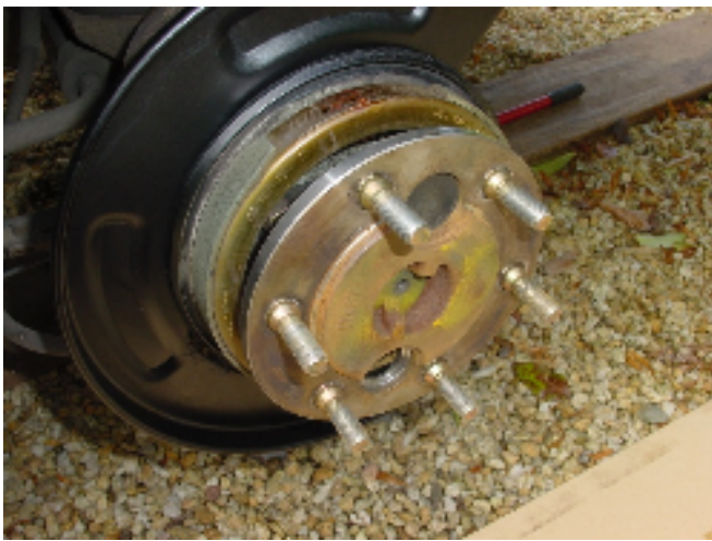
View on the clean parking brake shoe. Sprayed the dust plate.
