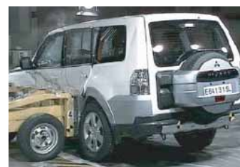
Side collision test (55km/h)
