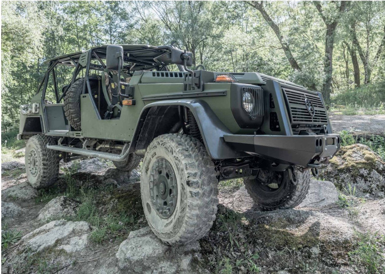
Commonality with other Mercedes-Benz products, EMC, 3,000 kg payload and a fording depth of 1,000 mm.
