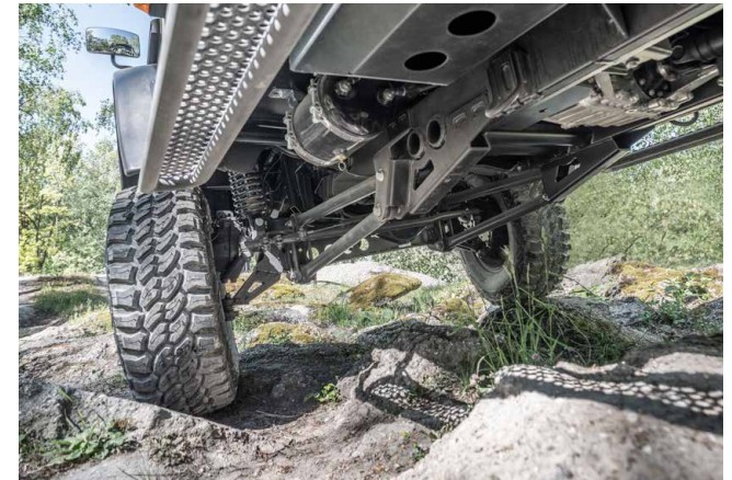
Suitable for poor-quality fuel (Euro 3), global service network, proven chassis and portal axles.
