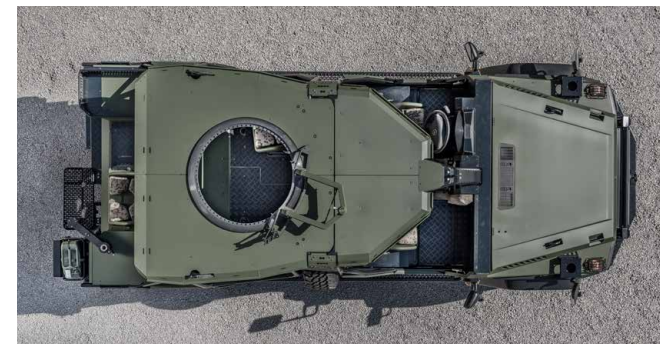
Modular structure, 2 to 6 seats,, modular protection concept, air-portable and a range of 800 km.
