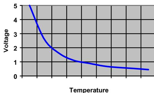
However, when the original engine coolant temperature signal is not useable to the SGI computer, the temperature signal will be provided by an additional sensor, which is supplied in the engine kit. The signal will be similar to the signal like shown above.
