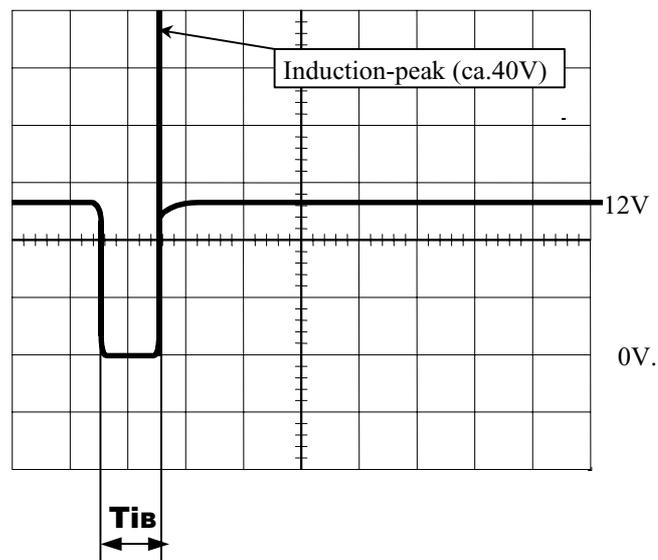
In most contemporary engines the petrol injectors are actuated separately (fully sequentially), but the injectors can also be actuated simultaneously. A hybrid form, in which the injectors are actuated in groups of two (half sequential), is also possible. In each case the injection strategy of the engine-management system will be followed completely.
