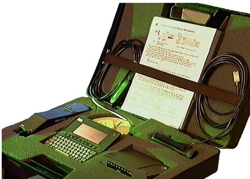
Modem communication is possible because a connection can be made (by means of the modem in the test kit) between the SGI computer and a computer located at the relevant Technical Department (see picture below).
