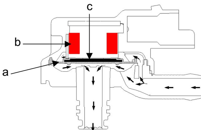
2. As soon as the magnetic field in the injector coil (b) drops the injector closes after the opening period, under the influence of the LPG pressure across the diaphragm (a), which is delivered by the vaporiser.
