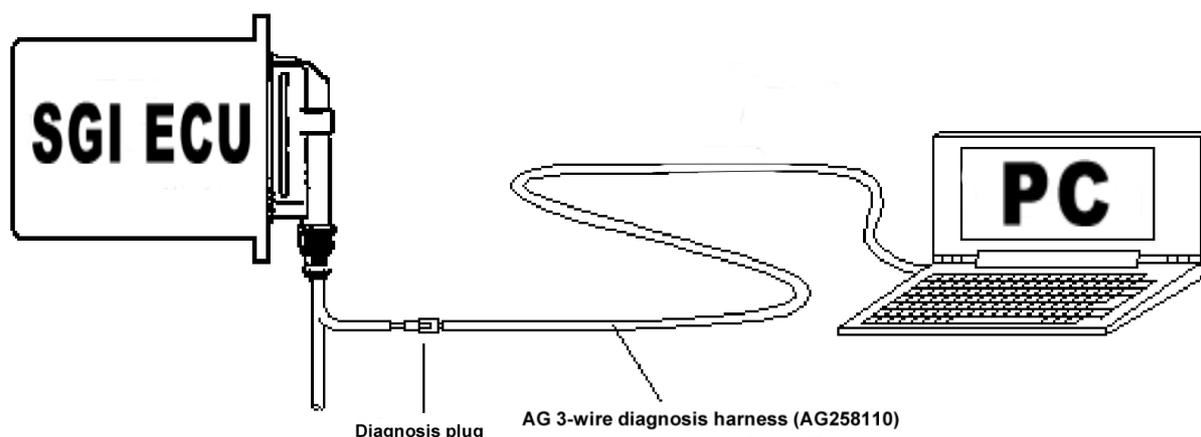
When using a PC or a laptop computer instead of the Psion, the "AGT" communication program must first be started from the MS-DOS prompt. This program can be found on the diskette supplied with the test kit. After that, making a diagnosis is exactly the same as when using the Psion..
