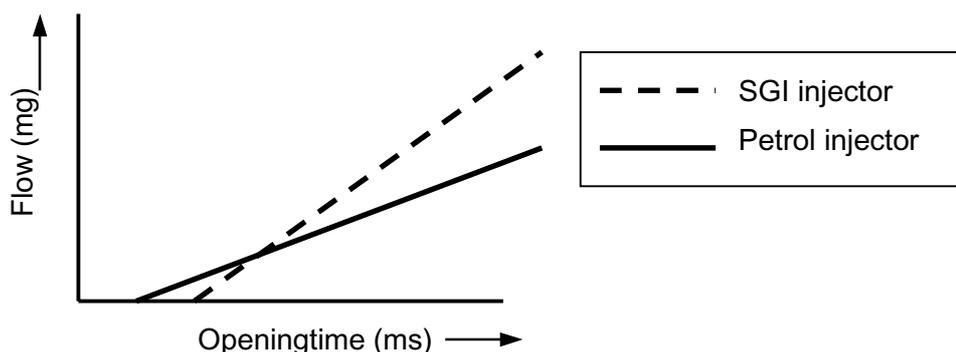
To be able to measure the opening period of the petrol injectors, they are simulated by the interface unit when driving on LPG. This simulation signal communicates the opening periods separately to the SGI computer. The computer then converts these periods to the exact opening periods for each SGI injector separately.
