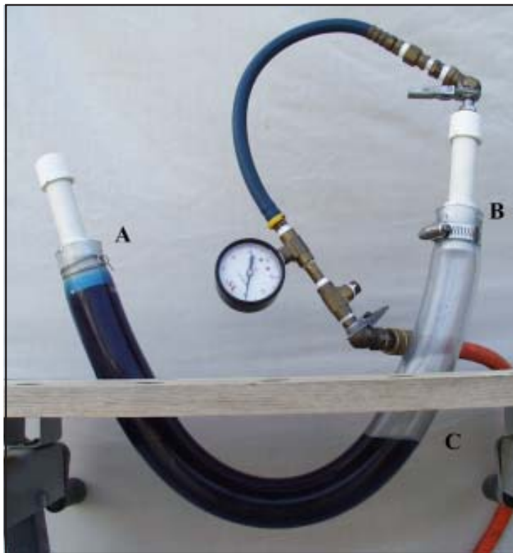
Figure 3 The test setup, at full pressure, on the ClampTite clamp.
