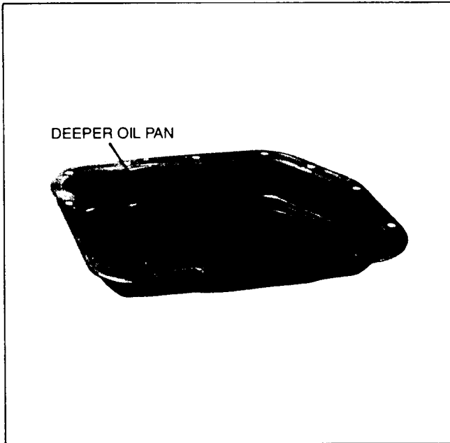
OIL PAN: A new deeper oil pan was required to provide room for the added valve body controls.
