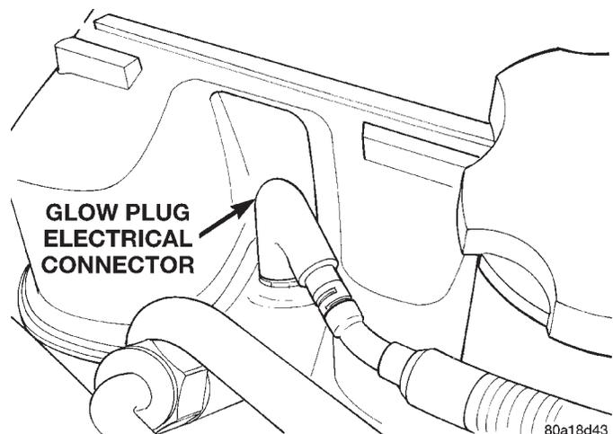
**Fig. 22 Glow Plug Electrical Connector**
