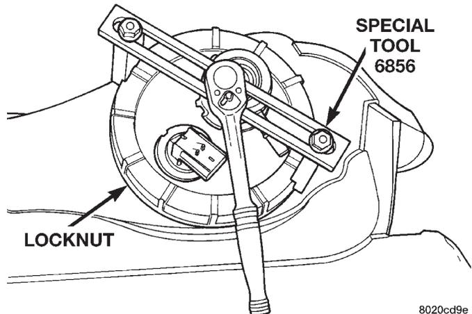
**Fig. 47 Fuel Reservoir Module Lock Nut Removal**
