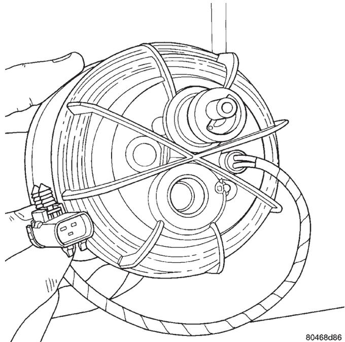
**Fig. 10 Fuel Heater Temperature Sensor and Element Location**
