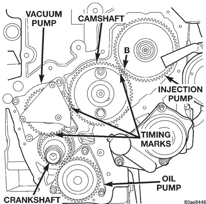
**Fig. 21 Vacuum Pump at Front of Engine**
