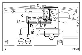
(e) Check that the voltage of terminals 5 and 6 of the connector E is battery positive voltage after terminals 1 and 2 of connector E have been disconnected and reconnected.
