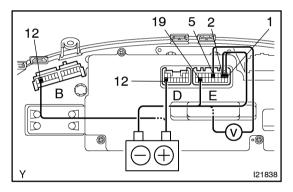
(c) Check that the voltage of terminal 5 of connector E is the battery positive voltage after the positive (+) lead from the battery has been connected to terminal 1 of connector E.
