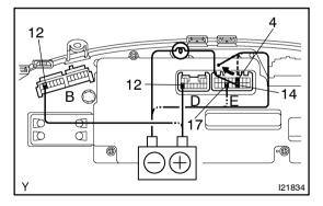
(g) Check that the bulb flashing when disconnecting terminal 4 of connector E from the negative (–) lead.
