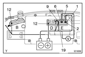
(d) Check that the voltage of terminals 5 and 6 of the connector E is 0 V after terminal 12 of connector B has been disconnected, and the positive (+) lead from the battery has been connected to terminal 9 of connector E.
