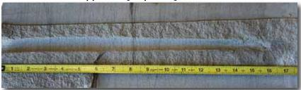
The PowerJet Nova charge's sandstone performance reveals increased penetration compared with previous-generation deep penetrating charges.
