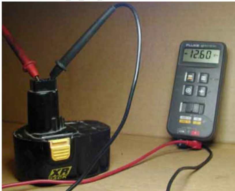
A 14.4V pack that reads 12V fresh off the charger.—This is not good.
