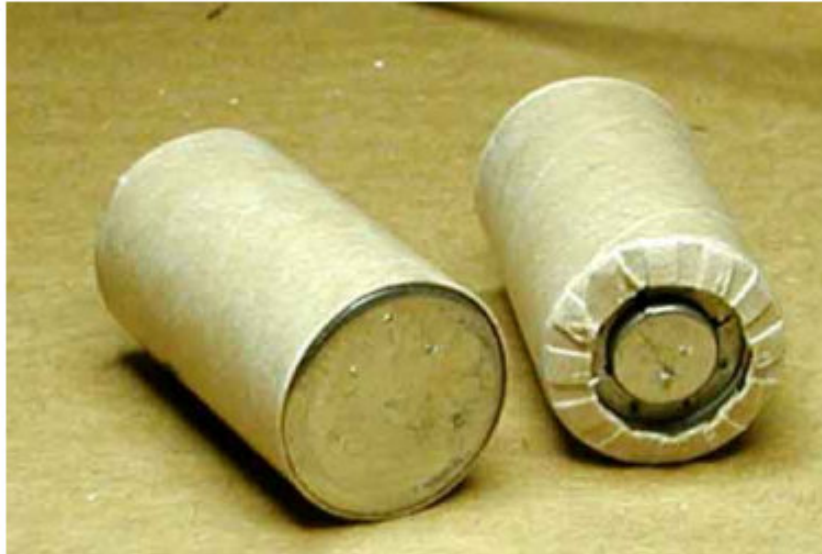
These cells have been removed. You can see the marks from the spot welds.
