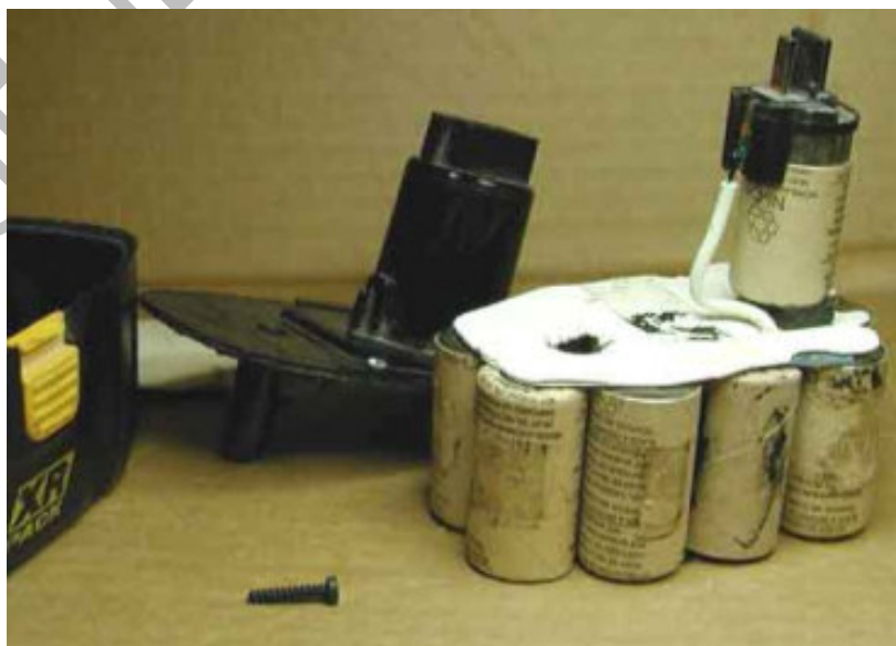
The cells inside a battery pack.
