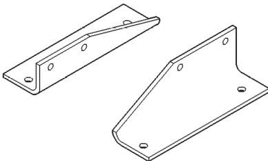
**Support Brackets Engine Removal/Installation
