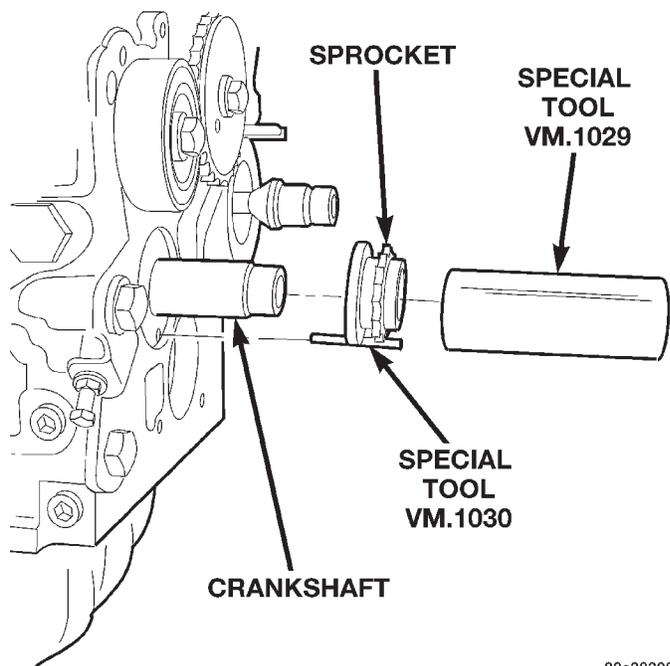
**Fig. 49 Crankshaft Sprocket—Installation**
