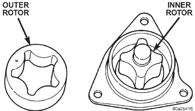
Fig. 92 Oil Pump Inner and Outer Rotors
