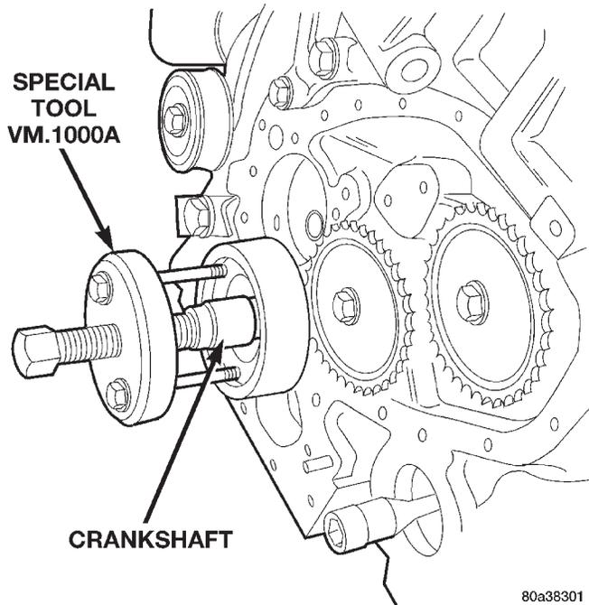
**Fig. 48 Crankshaft Sprocket—Removal****INSTALLATION**
