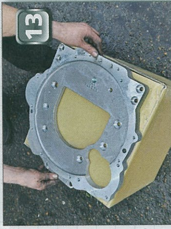
PICTURE 10 ...and a bolt-on cover plate fitted later. It's all beautifully accurate and well machined by Motor & Diesel Engineering from whom I bought the parts, via Ashcroft Transmissions.
