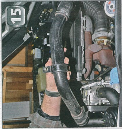
PICTURE 21 He then refitted the bottom intercooler hose only this time...
