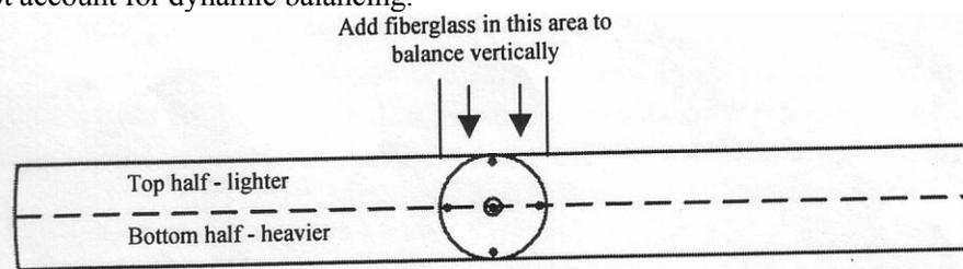
Insert through prop and rest on angle iron knife edge so the prop is between the two sawhorses.
