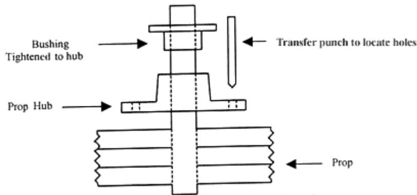
Proper aligning to mark bolt hole location.
