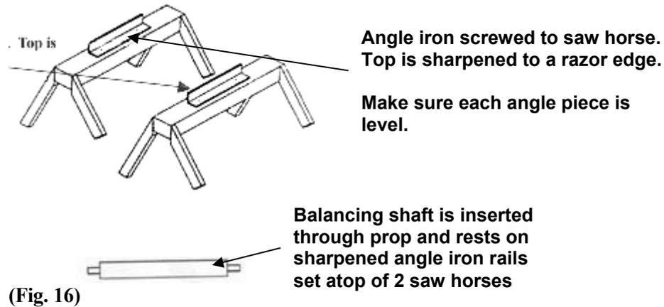
The propeller should be balanced statically. If you have access to a dynamic balancing machine and an experienced person get the propeller dynamically balanced. For approximate balance, position the propeller blades horizontally. Release and observe which blade falls. Add extra fiberglass to the lighter side to balance the weight until the propeller remains in a horizontal position after releasing. This statically balances the prop, but does not account for dynamic balancing.
