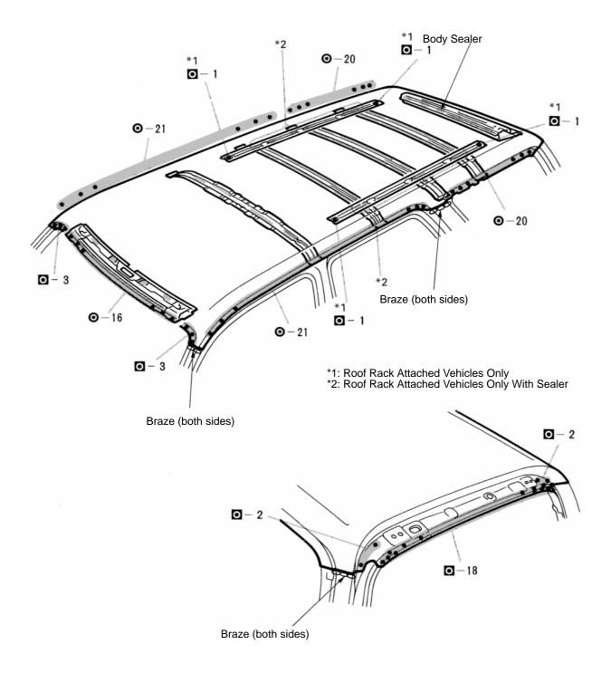
Before temporarily installing new parts, apply body sealer to the windshield header panel, roof panel reinforcement, roof rack support and back door opening frame.
