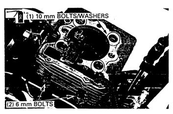
Install the cam chain guide.
