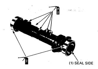
Install the camshaft bearing set pins.
