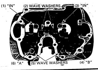
Apply locking agent to the sub-rocker arm shaft threads as shown.
