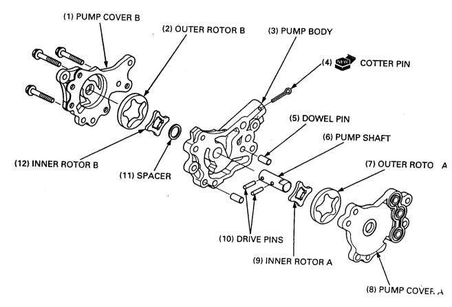
Install the following to the pump body.
