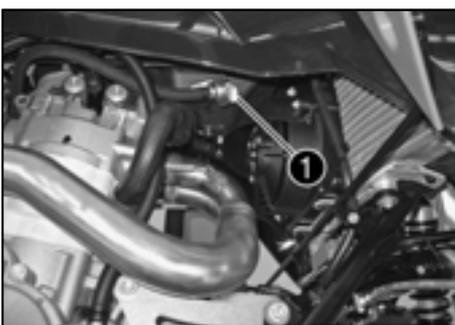
The fuel tap is located on the right side of the fuel tank.
