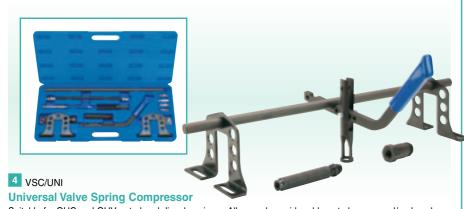
Suitable for OHC and OHV petrol and diesel engines . Allows valve guide rubbers to be removed/replaced without the need to remove the head. Supplied complete with valve holder, quick-release air couplings and valve stem installer/remover. Packed in handy case with display sleeve.
