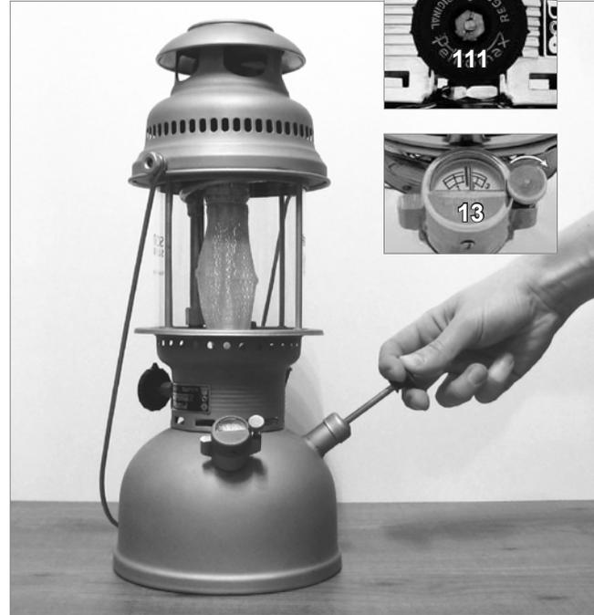
Nose of the grip wheel (#111) has to face upwards. Rocker arm (#223) of the pre heater and ventilating screw (#13) at the manometer have to be closed. Inflate until manometer needle exceeds the red mark.
