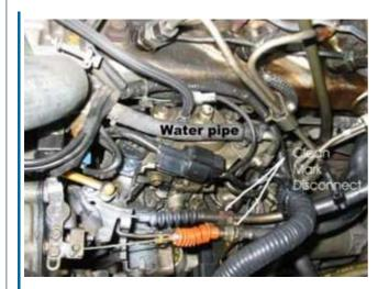
Disconnect the orange and black cables marking the position of the adjusting nuts.
