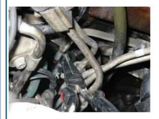
Disconnect the fuel pump water hoses X2. (You may not have these if you don't have the cold start pack) Hose 1 runs across the top of the fuel pump. Hose 2 is between the 4 fuel pipes and the engine
