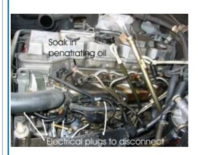
Disconnect the electrical harness. Take note which connector plugs onto what.
