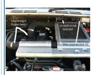
Disconnect the 2 hoses as shown. Use a plastic bag to block the hole next to the oil filler cap. There are 4 bolts securing the frame of the intercooler.
