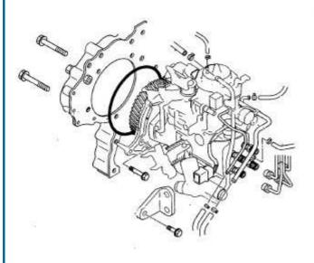
Now for the swearing. There is a short bolt that holds the fuel pump to a bracket. From the rubber water hose that went across the top of the fuel pump, follow it down the side of pump (now a metal pipe). It ends in a banjo bolt (I recommend you remove this pipe for access). Go under the pump and slightly forward. I told you you'd swear. It needs a 14mm socket.
