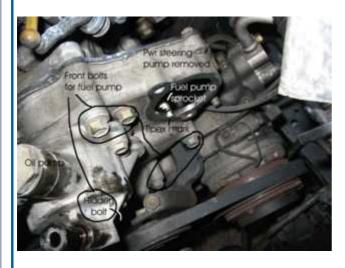
Remove the oil pressure switch and the metal pipe that connects the oil pump to the engine. Take care not to
