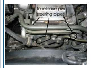
Release the brackets that support the pipes for the power steering pumps.
