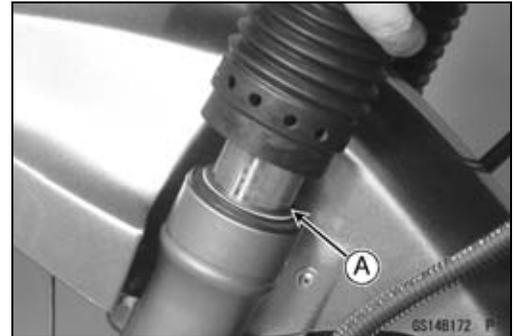
*Rear Shock Absorber Oil Leak Inspection*
