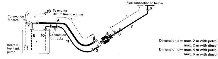
2.2 If it is not possible to fit a separate riser pipe in the case of cars with petrol injection engines, the return line can be tapped using a T-piece.
