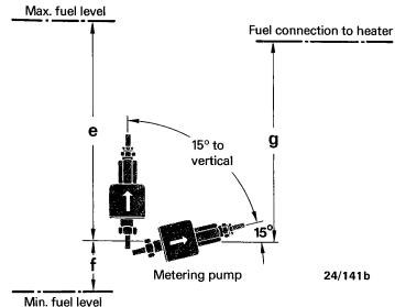
Supply pressure from tank to metering pump:
