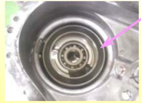
If EMC is energized, the multiple disc clutch is engaged so the torque is transmitted to front wheel. Depends on EMC duty ratio, the amount of transmitted torque to front side is changed.
