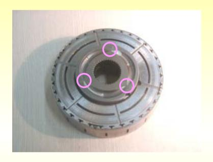
3 steel balls (Ball ramp mechanism) were installed to be controlled by EMC.
