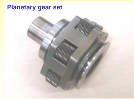
To make 4LOW gear ratio (2.480), the planetary gear set was installed and controlled by electronic shift fork. The connecting point 'A' and 'B' is shifted depends on the moving direction of shift fork.
