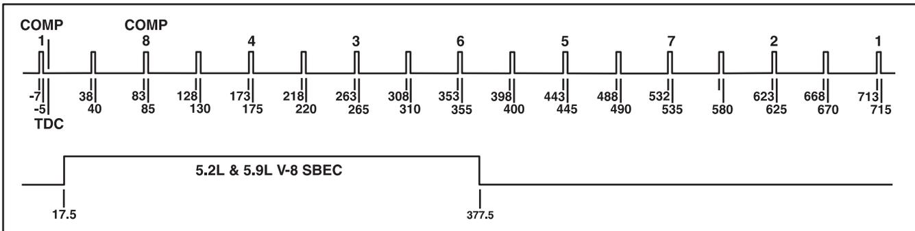
Figure 24 Crankshaft Position Sensor Notches — 5.2L/5.9L
