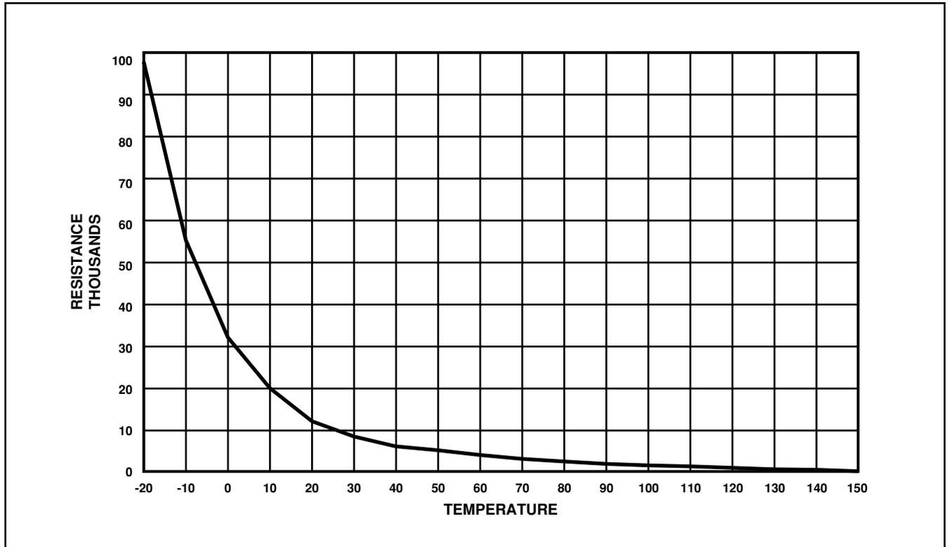
Figure 56 Battery Temperature Sensor — Resistance vs. Temperature
