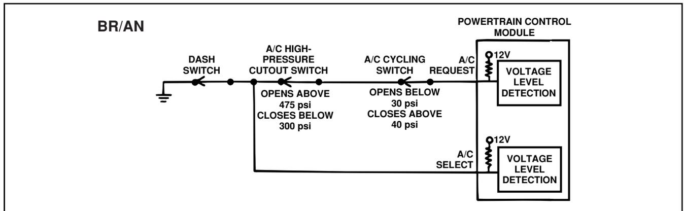
Figure 58 BR/AN Air Conditioning Switch Circuit
