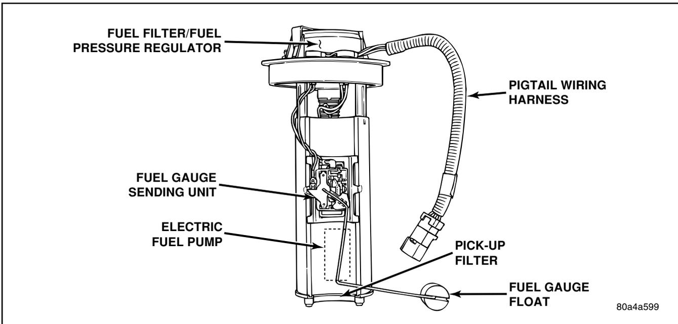
Figure 7 Typical 1997 Jeep® Fuel Pump Module
