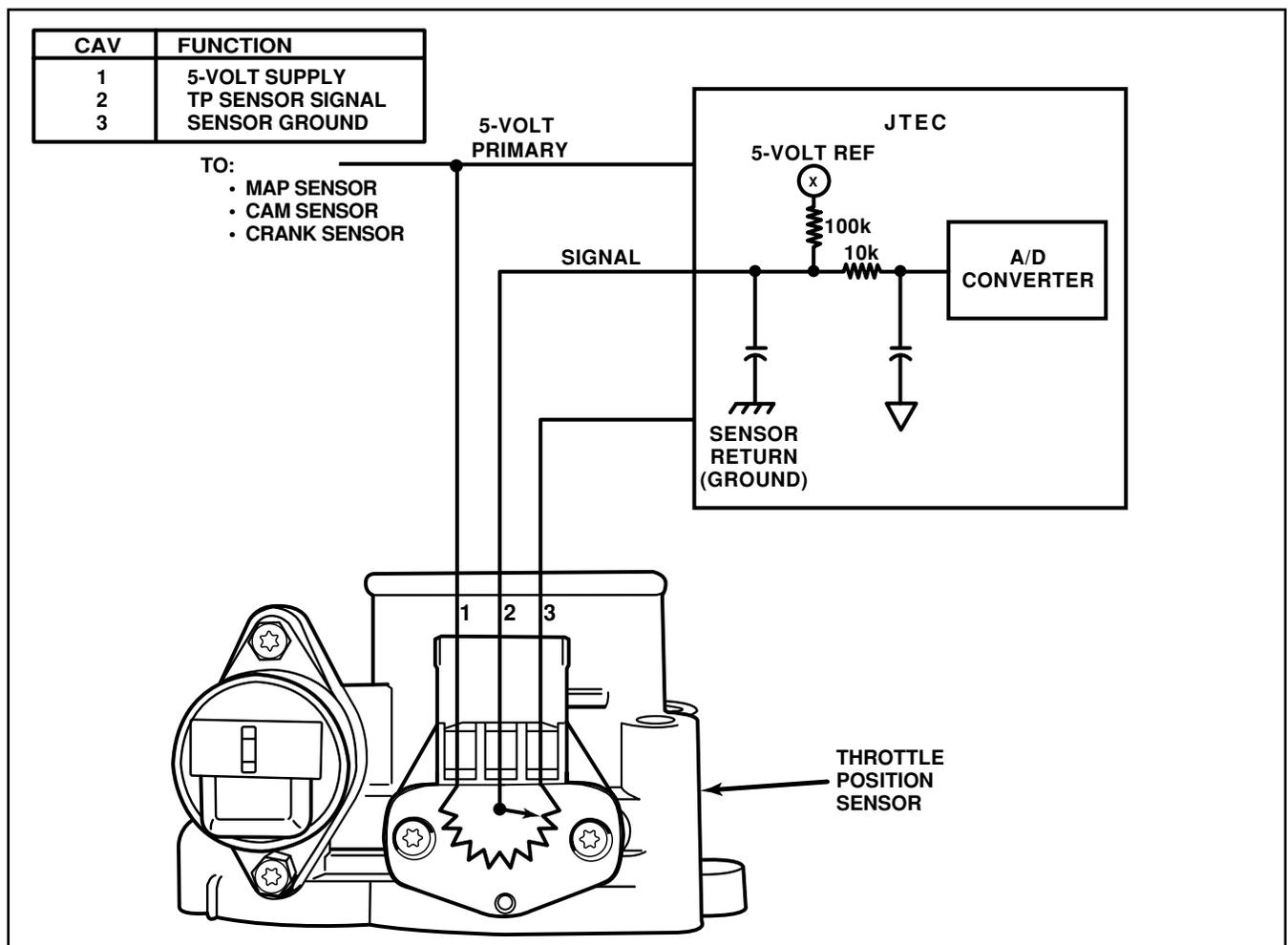
Figure 35 Throttle Position Sensor Circuit
