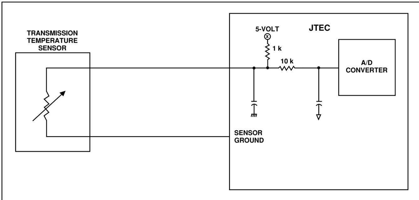
Figure 85 Transmission Temperature Sensor Circuit
