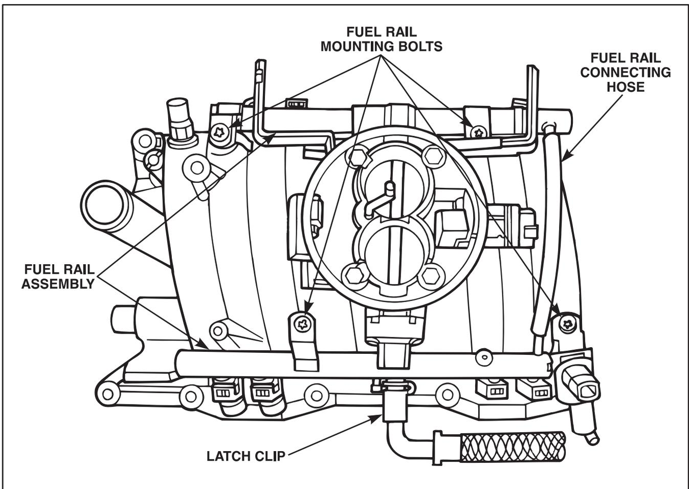
Figure 11 Fuel Rail — V6/V8 Engines
