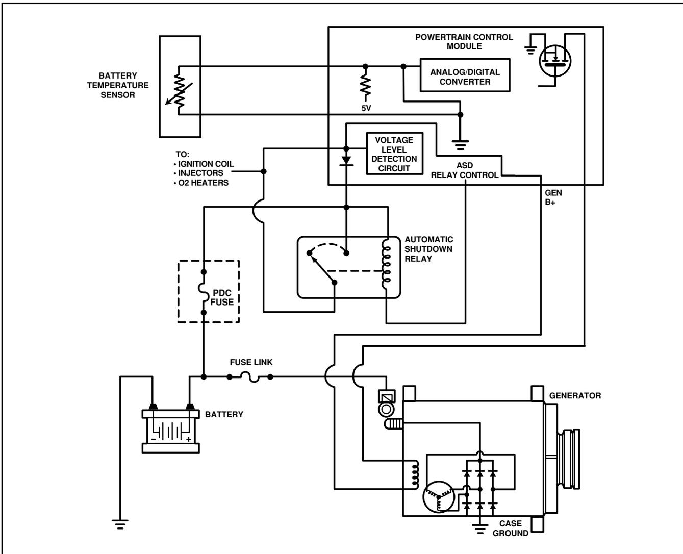
Figure 72 Generator Field Control Circuit — Typical '97
