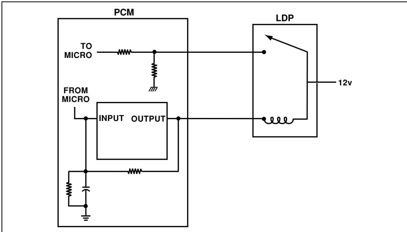
Figure 76 Leak-Detection Pump Control Circuit
