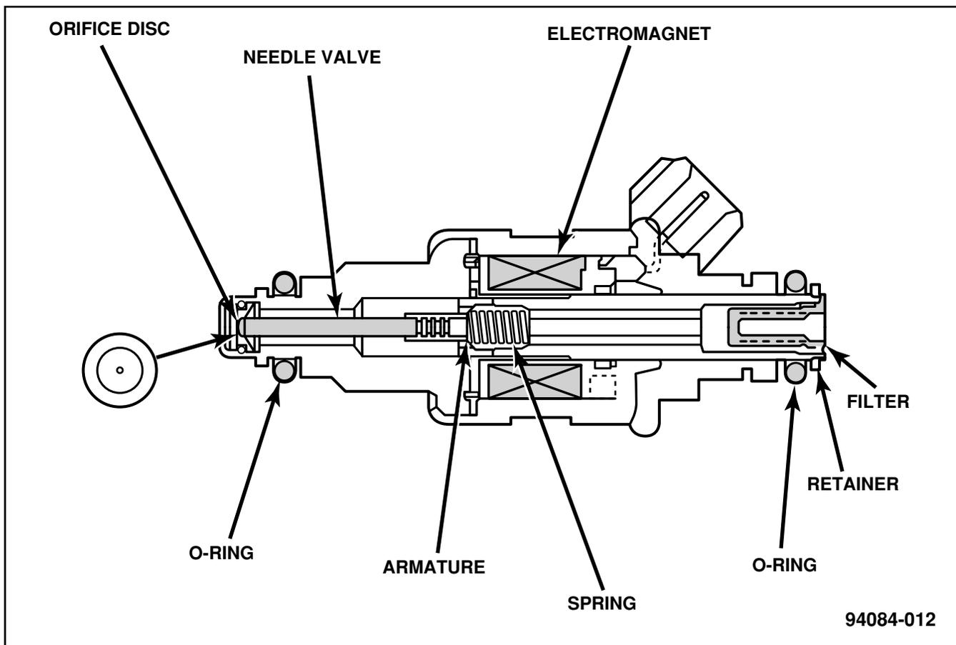
Figure 10 Fuel Injector
