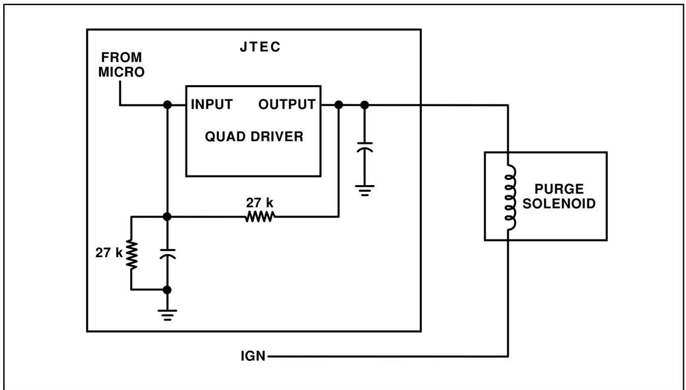
Figure 75 Duty-Cycle Purge Solenoid Control Circuit
