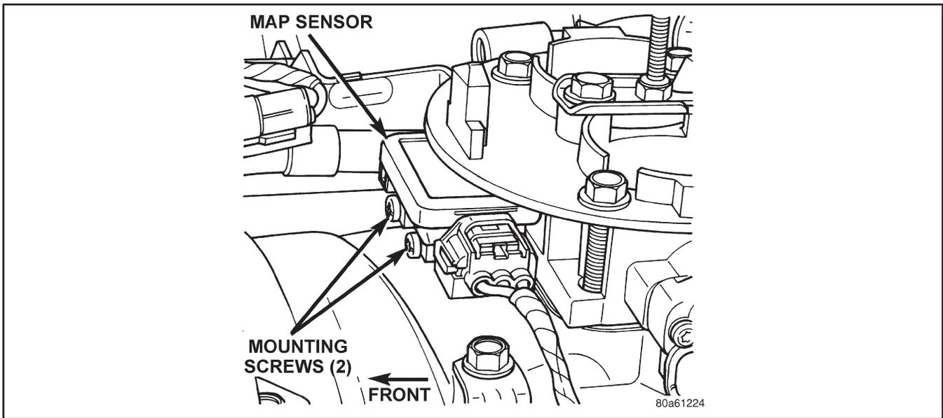
Figure 32 Manifold Absolute Pressure Sensor Location
