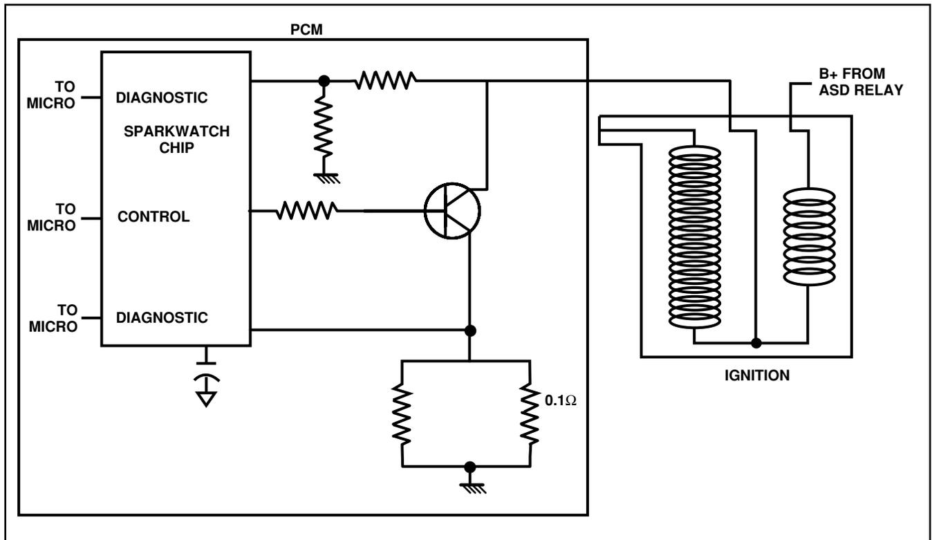
Figure 67 Ignition Control Circuit
