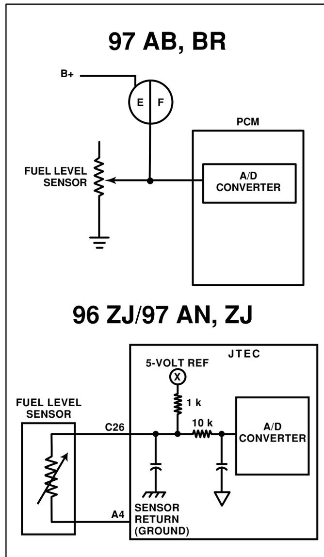
Figure 54 Fuel-Level Sensor Circuits
