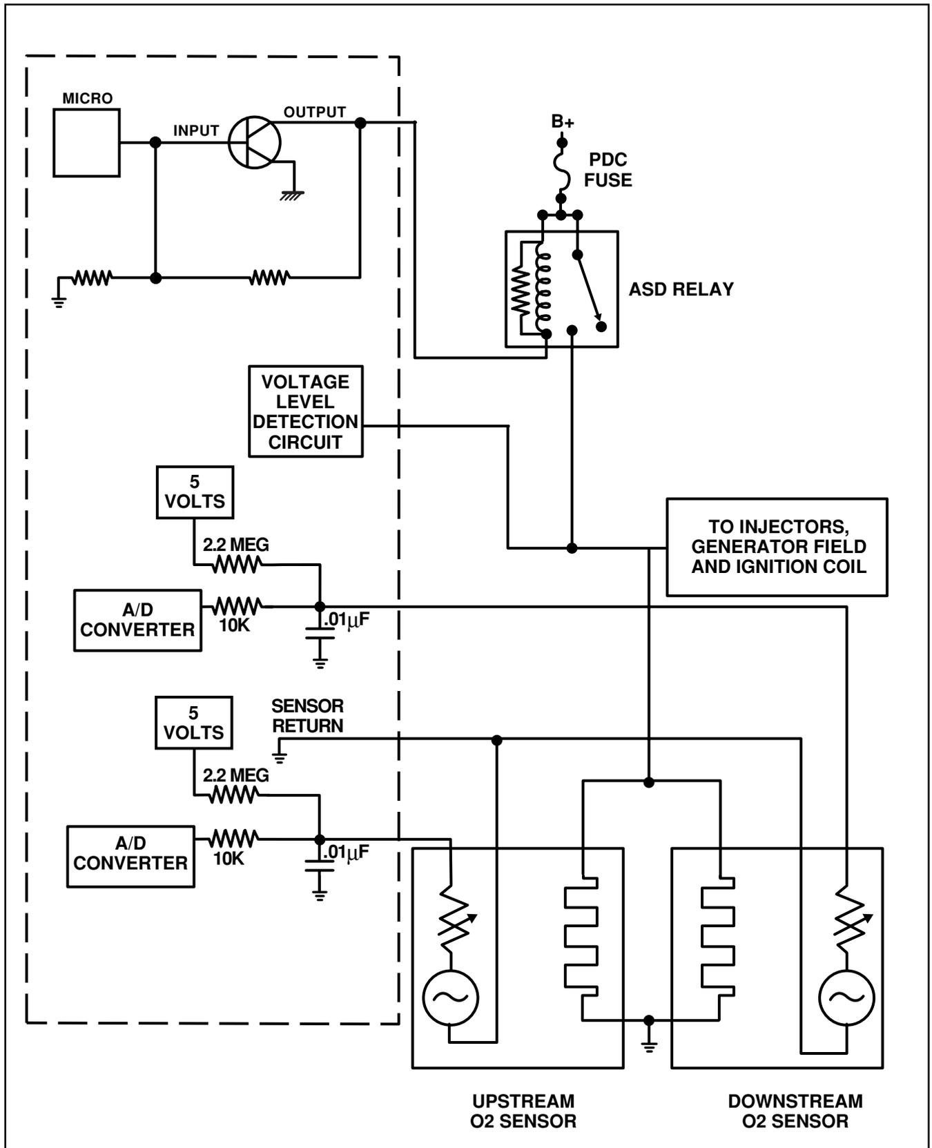
Figure 45 Dual O2 Sensor Circuit
