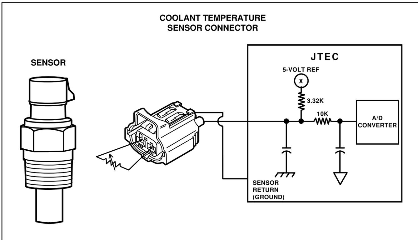
Figure 36 Engine Coolant Temperature Sensor Circuit
