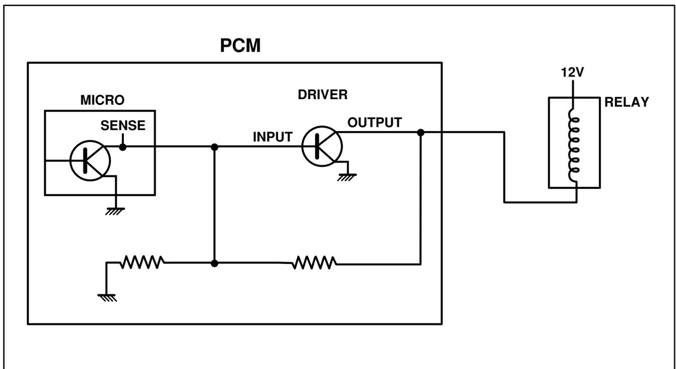
Figure 61 Sense Circuit
