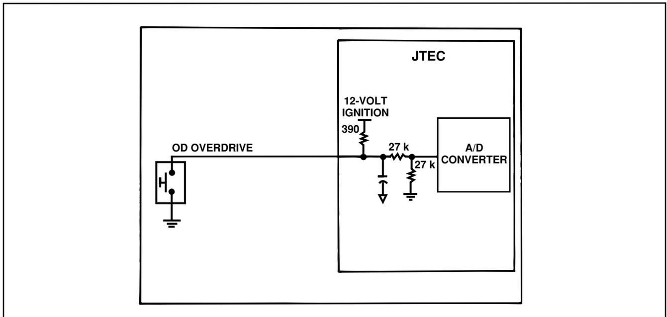
Figure 87 Overdrive Off Switch Circuit
