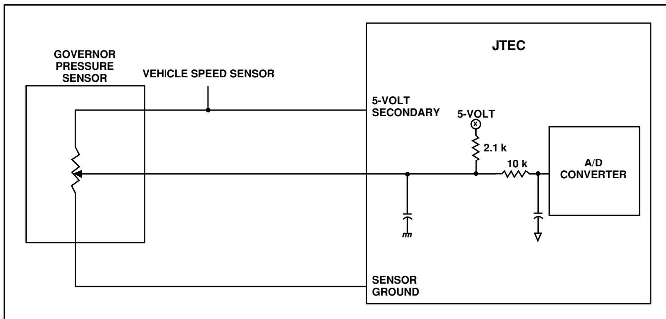
Figure 83 Governor Pressure Sensor Circuit
