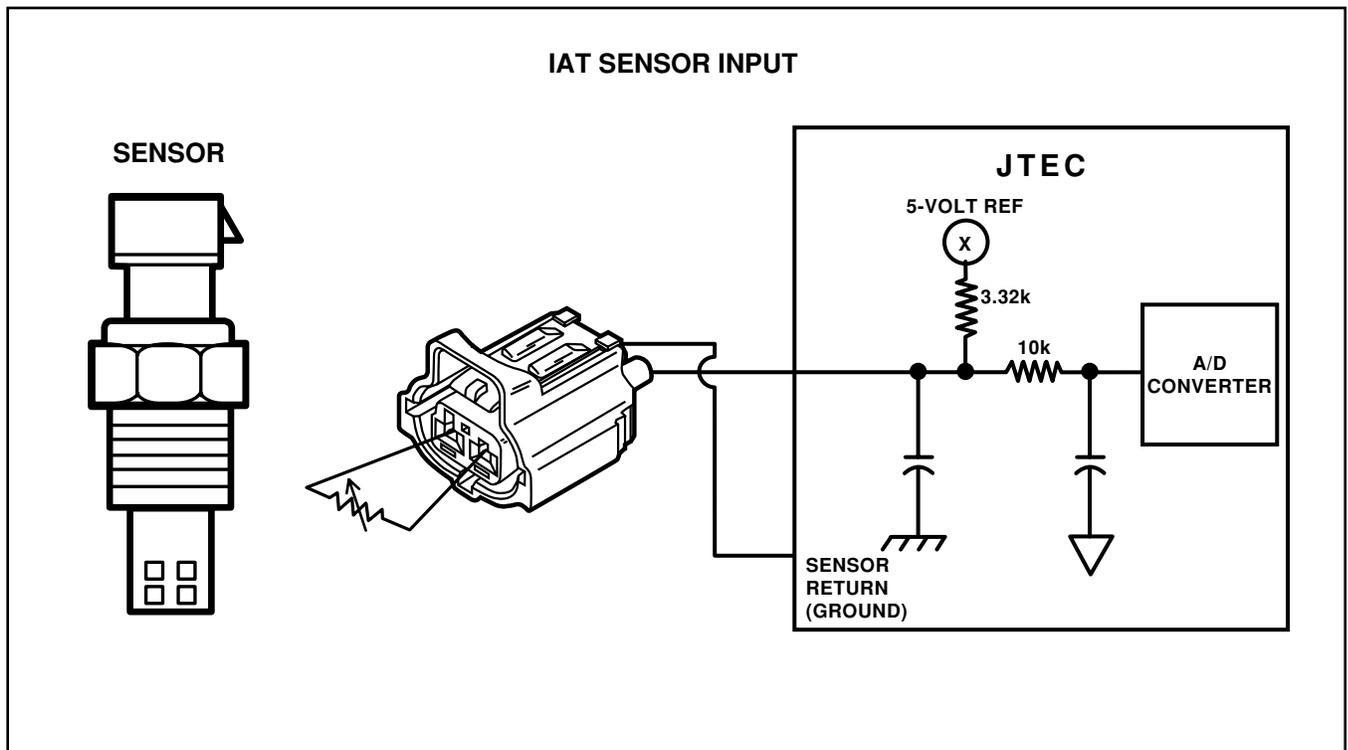
Figure 40 Intake Air Temperature Sensor Circuit
