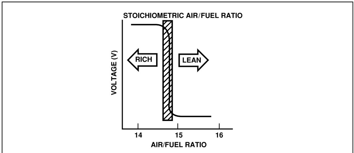
Figure 46 Oxygen Sensor Output
