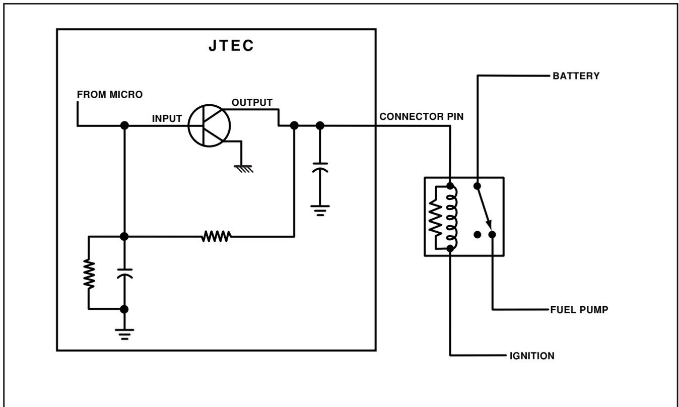
Figure 64 Fuel Pump Relay Circuit
