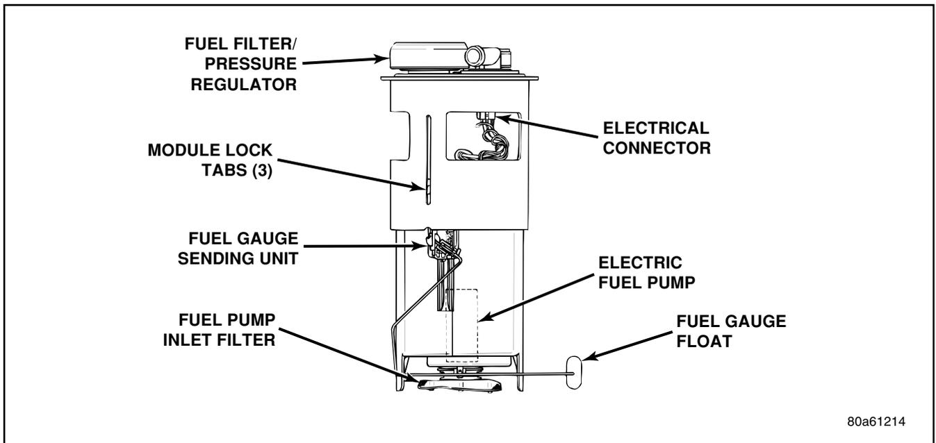
Figure 6 Typical 1997 Dodge Truck Fuel Pump Module
