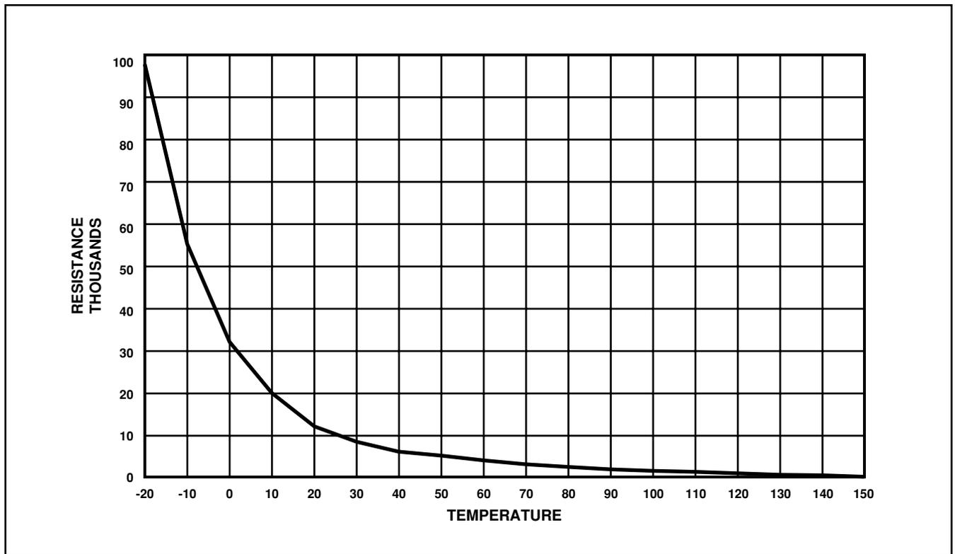
Figure 38 ECT/IAT Temperature/Resistance Curve
