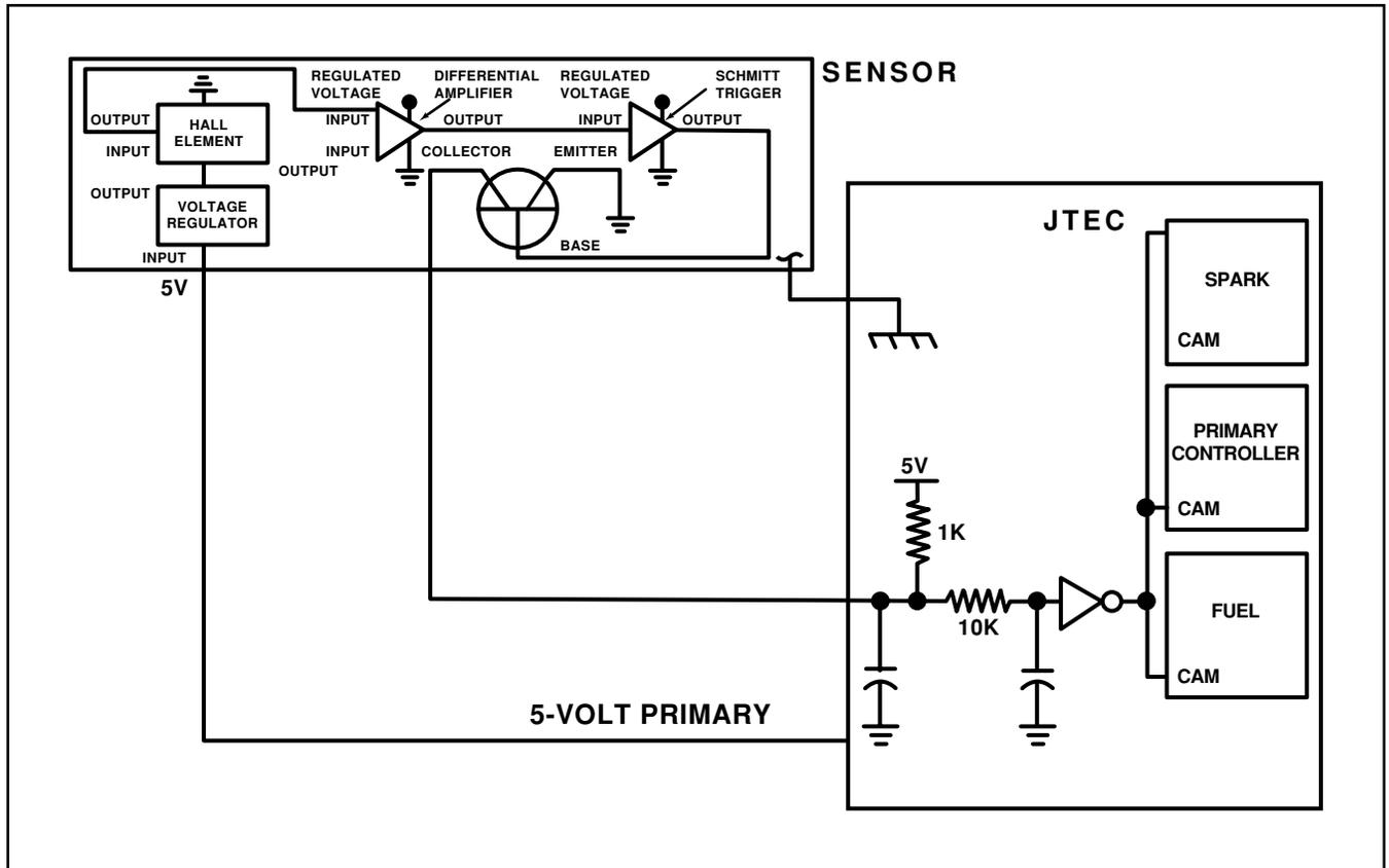
Figure 25 Camshaft Position Sensor Circuit
