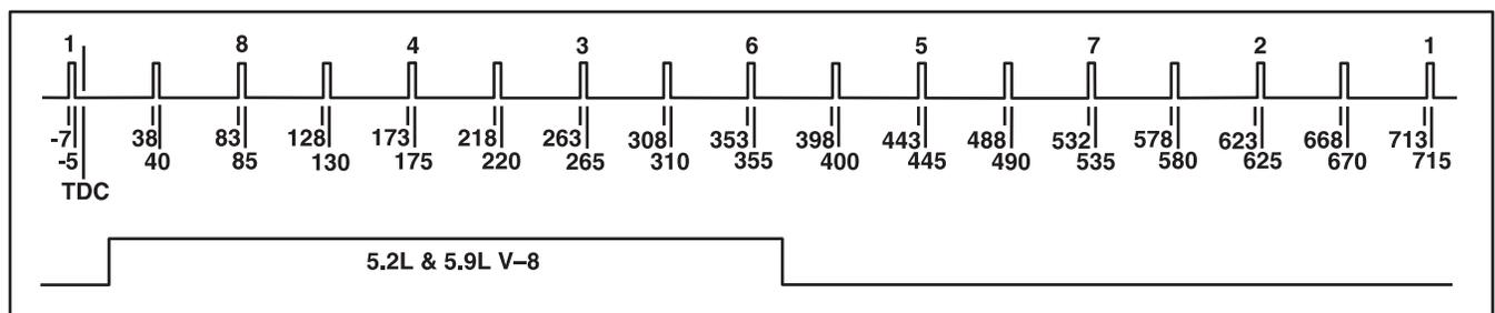
Figure 28 V8 Injector Pulse Widths
