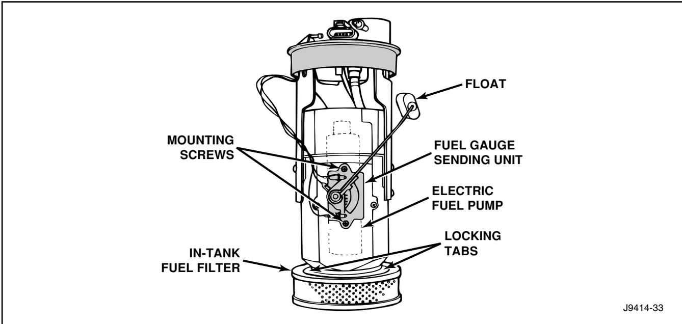
Figure 4 1996 Typical Dodge Truck Fuel Pump Module
