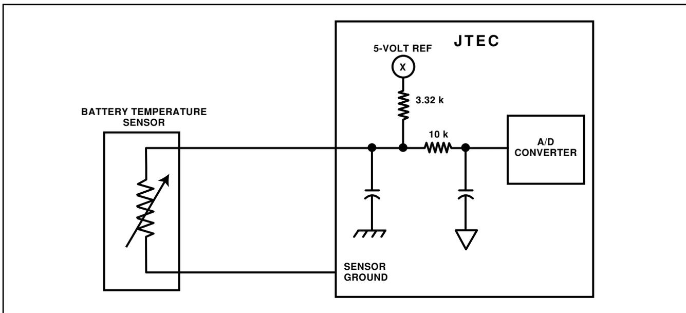
Figure 55 Battery/Ambient Temperature Sensor Circuit
