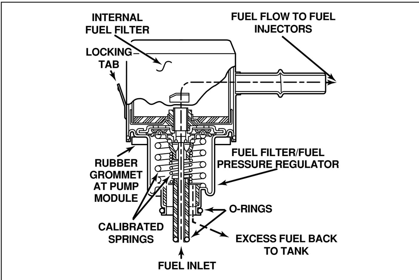
Figure 8 Typical One-Piece Filter/Regulator
