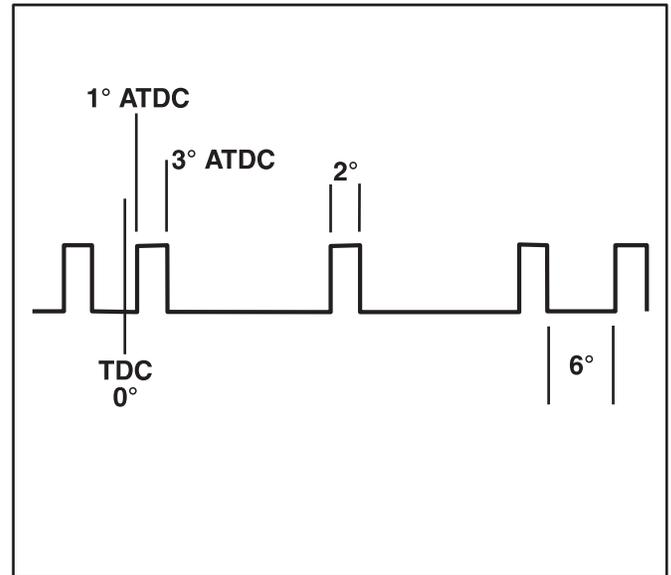
Figure 20 3.9L Crankshaft Syncs
