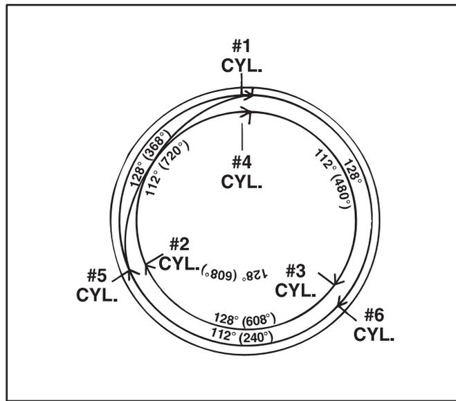
Figure 30 3.9L Ignition Coil Firing Sequence
