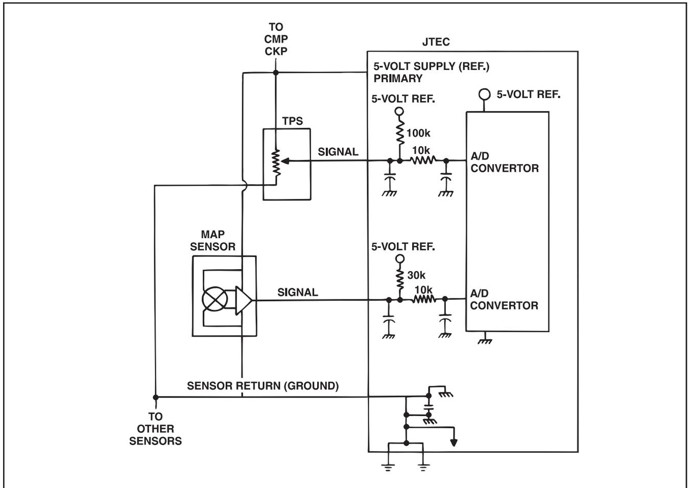
Figure 31 Manifold Absolute Pressure Sensor Circuit
