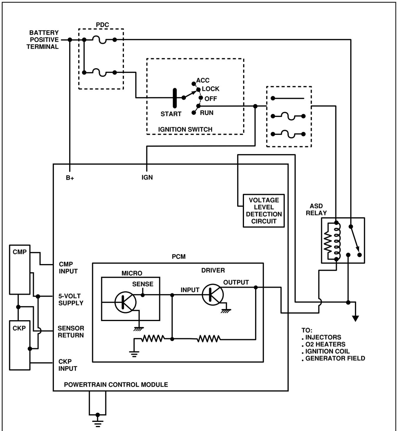
Figure 62 ASD Relay Circuit — Typical '96
