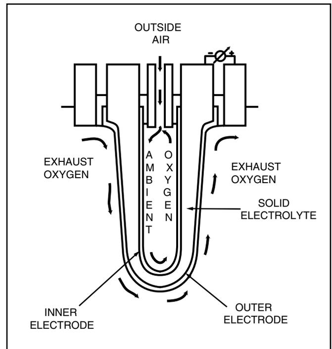
Figure 42 Oxygen Sensor Internal Operation
