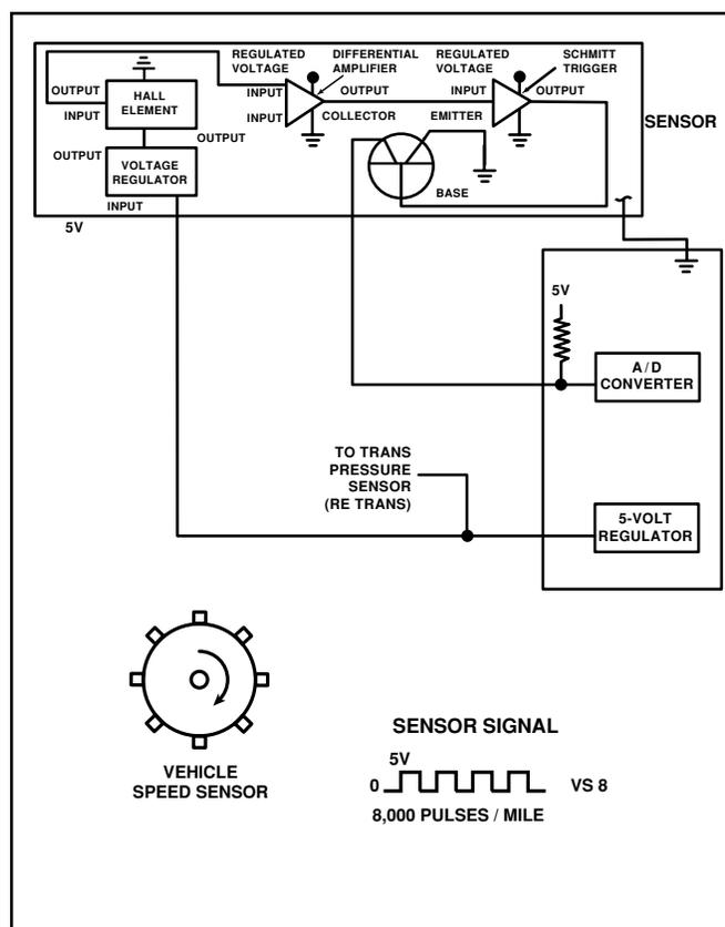
Figure 53 Vehicle Speed Sensor Circuit
