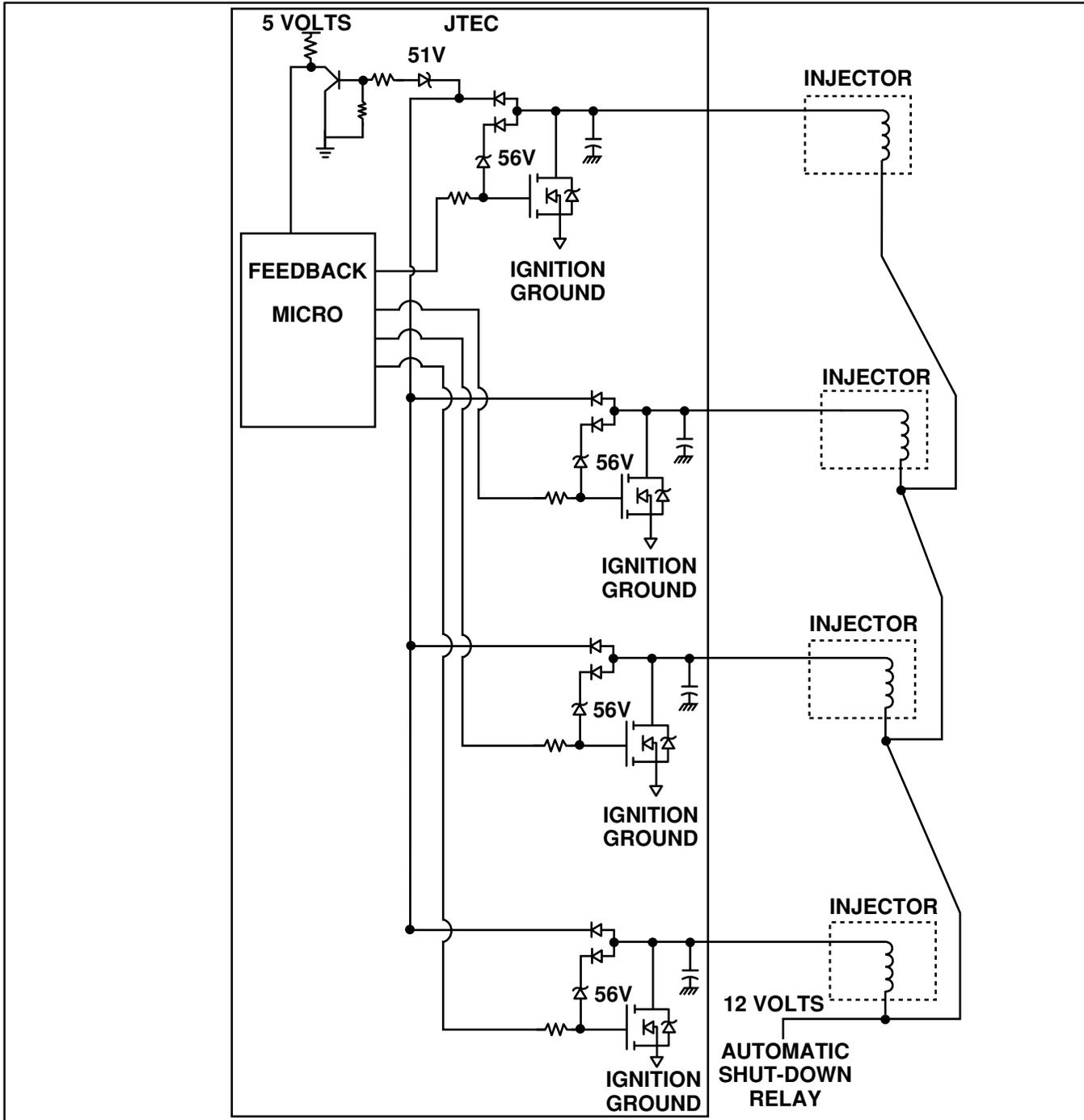
Figure 65 Fuel Injection Circuit
