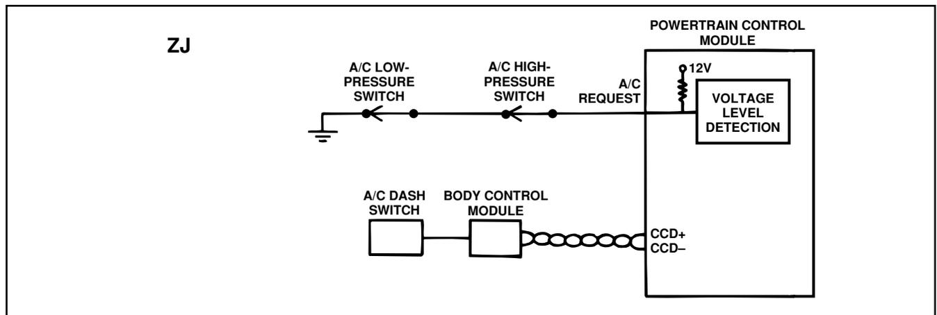
Figure 59 ZJ Air Conditioning Switch Circuit
