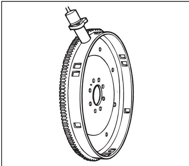
Figure 19 V6 Crankshaft Sensor
