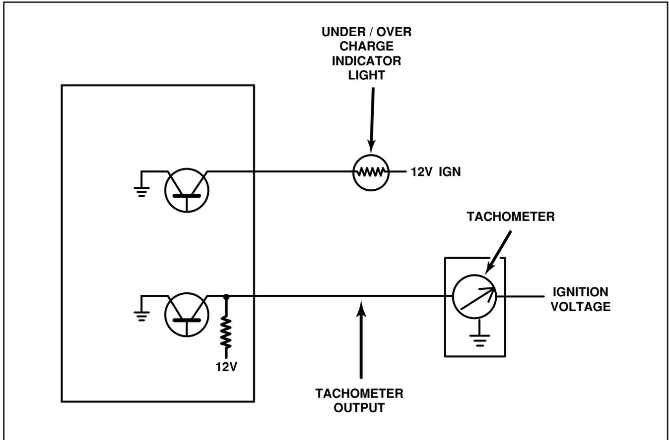
Figure 73 Generator Lamp Control Circuit
