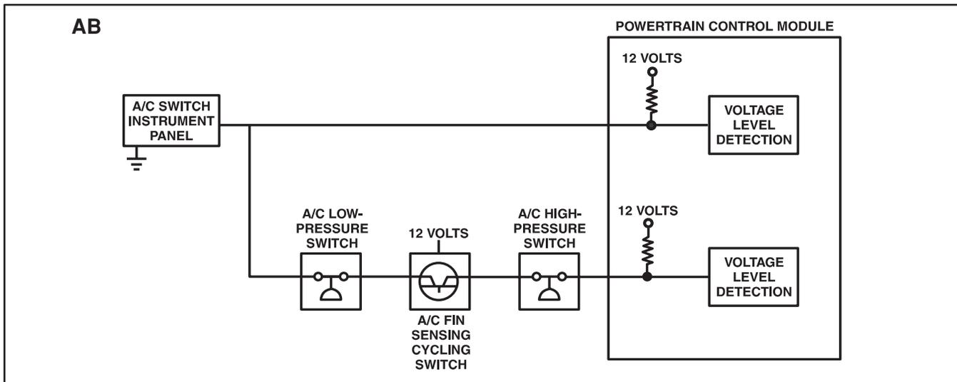
Figure 60 AB Air-Conditioning Switch Circuit
