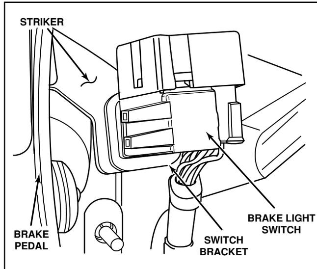
Figure 52 Brake Switch Location
