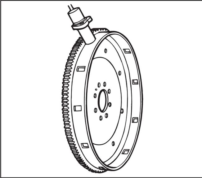
Figure 22 V8 Crankshaft Sensor
