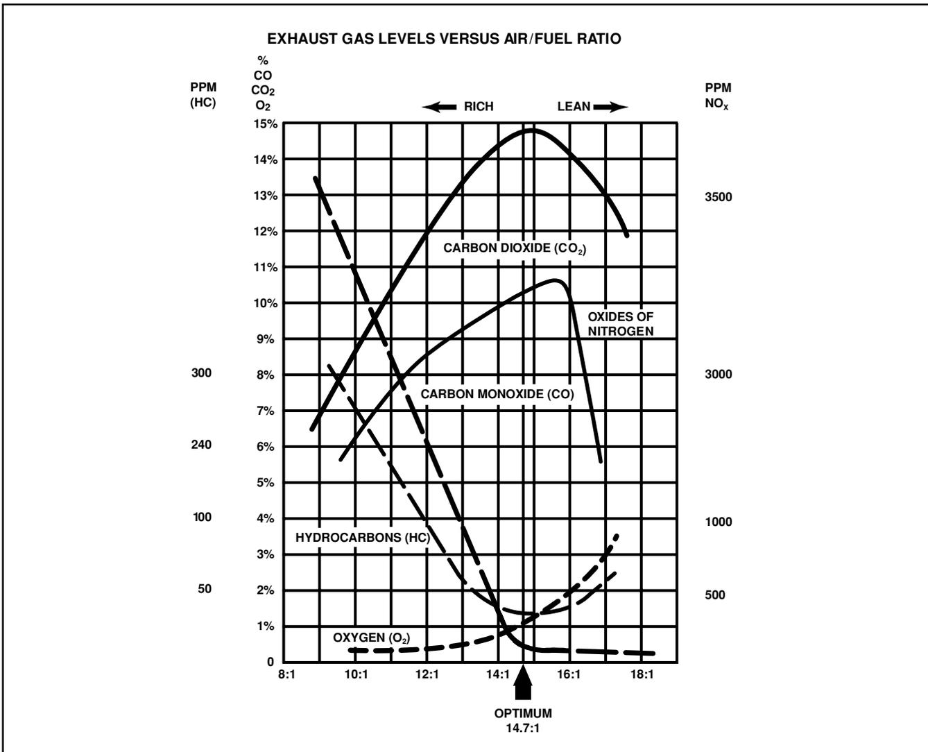
Figure 43 Exhaust Emissions vs. Air/Fuel Ratio
