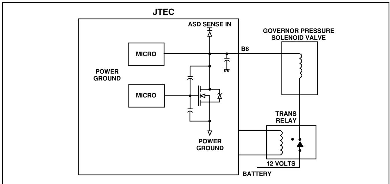
Figure 84 Governor Pressure Solenoid Valve Circuit
