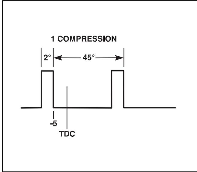
Figure 23 5.2L/5.9L Crankshaft Syncs
