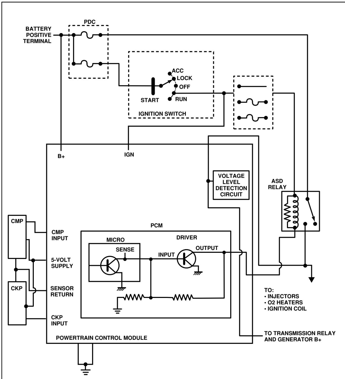
Figure 63 ASD Relay Circuit — Typical '97
