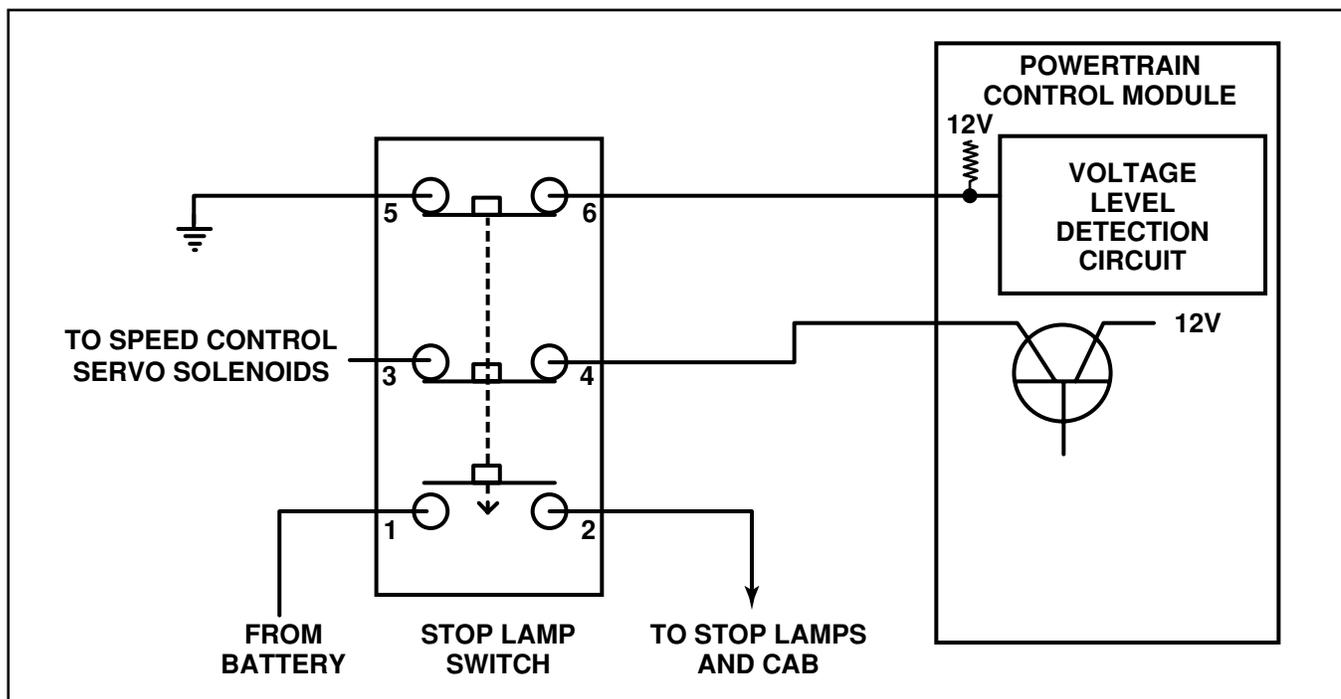
Figure 51 Brake Switch Circuit
