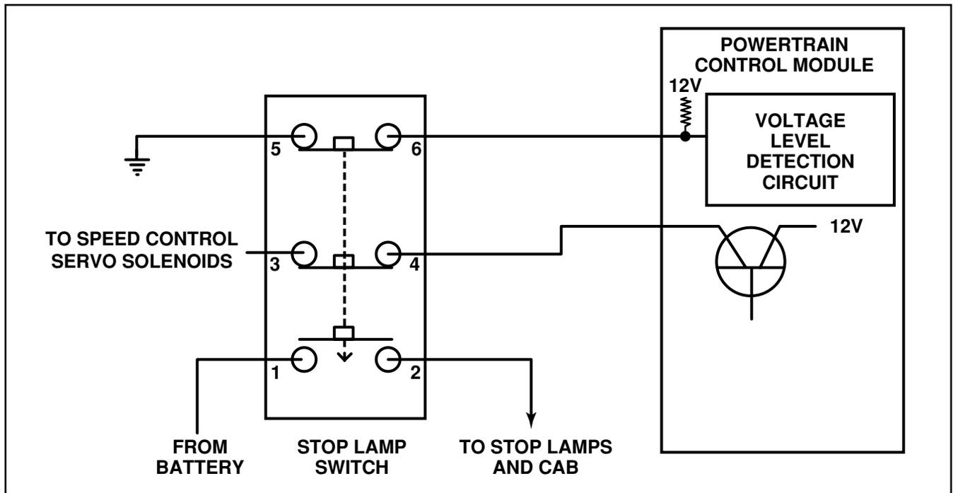
Figure 78 Brake Switch Circuit
