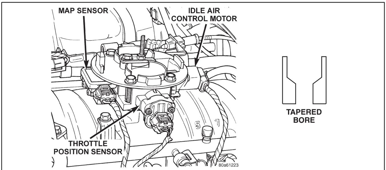
Figure 12 V6/V8 Throttle Body
