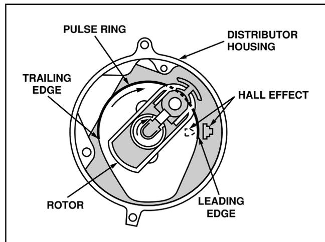
Figure 27 Camshaft Position (Hall-Effect) Sensor
