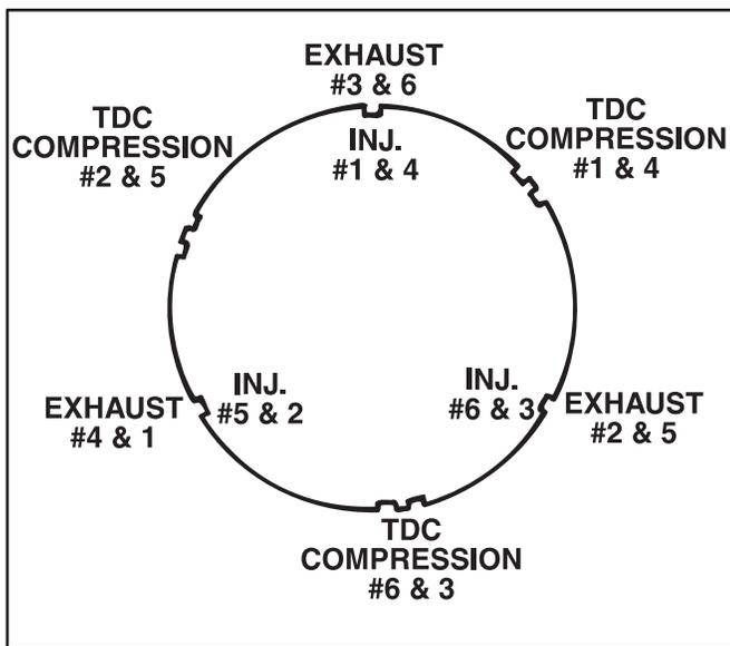
Figure 29 3.9L Injector Firing Sequence
