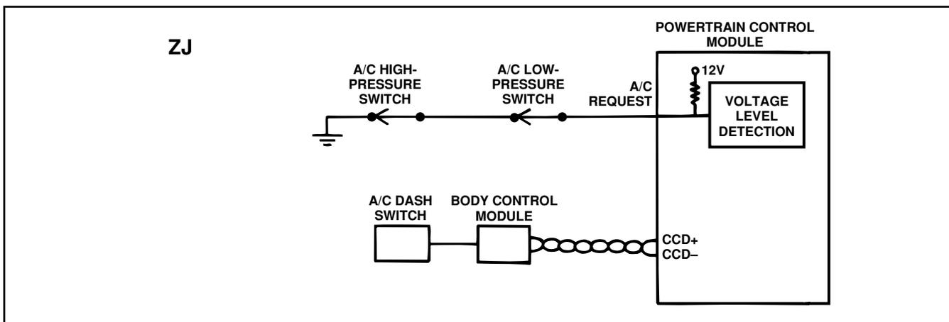
Figure 81 ZJ Air Conditioning Switch Circuit
