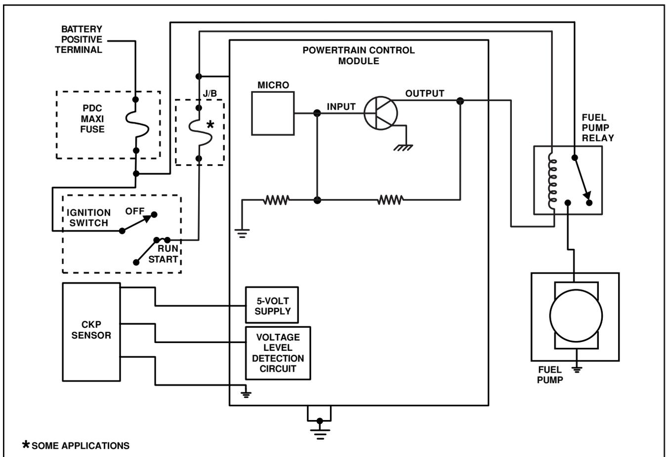
Figure 9 Fuel Pump Relay Circuit
