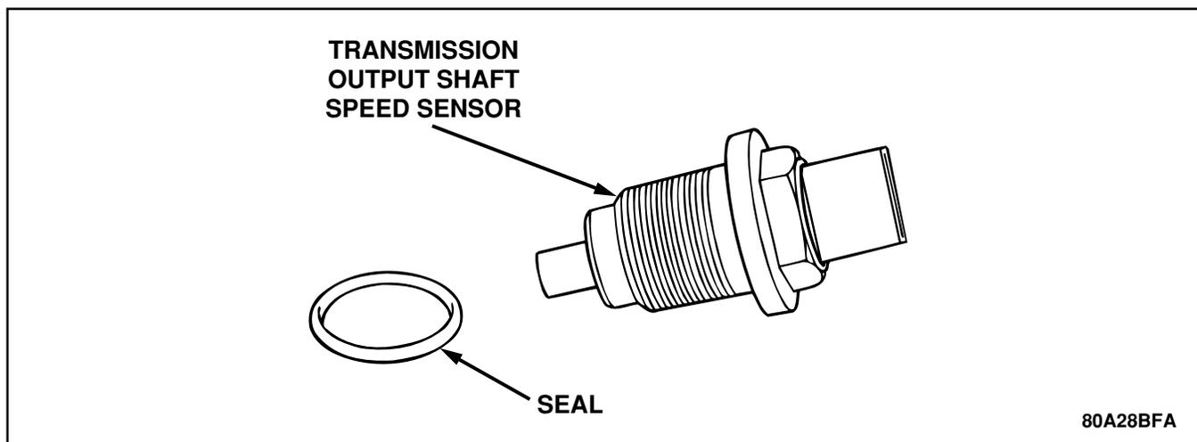
Figure 86 Speed Sensor Location
