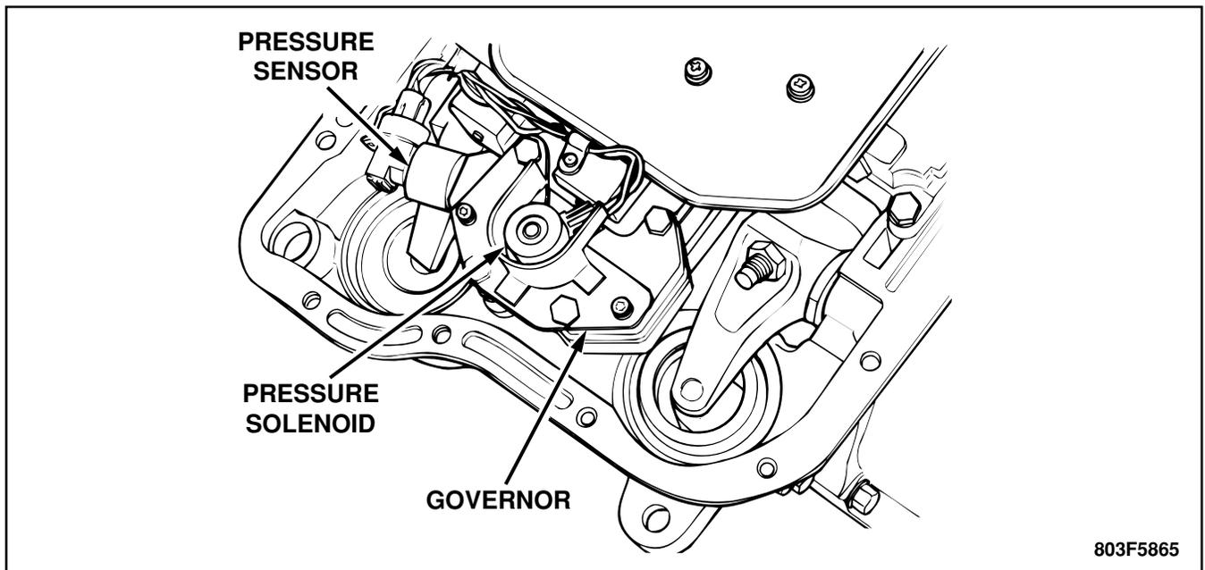
Figure 82 Governor Pressure Solenoid Location
