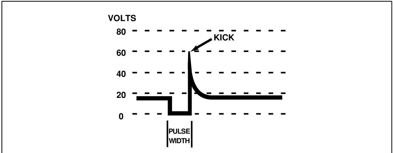
Figure 66 Injector Spike
