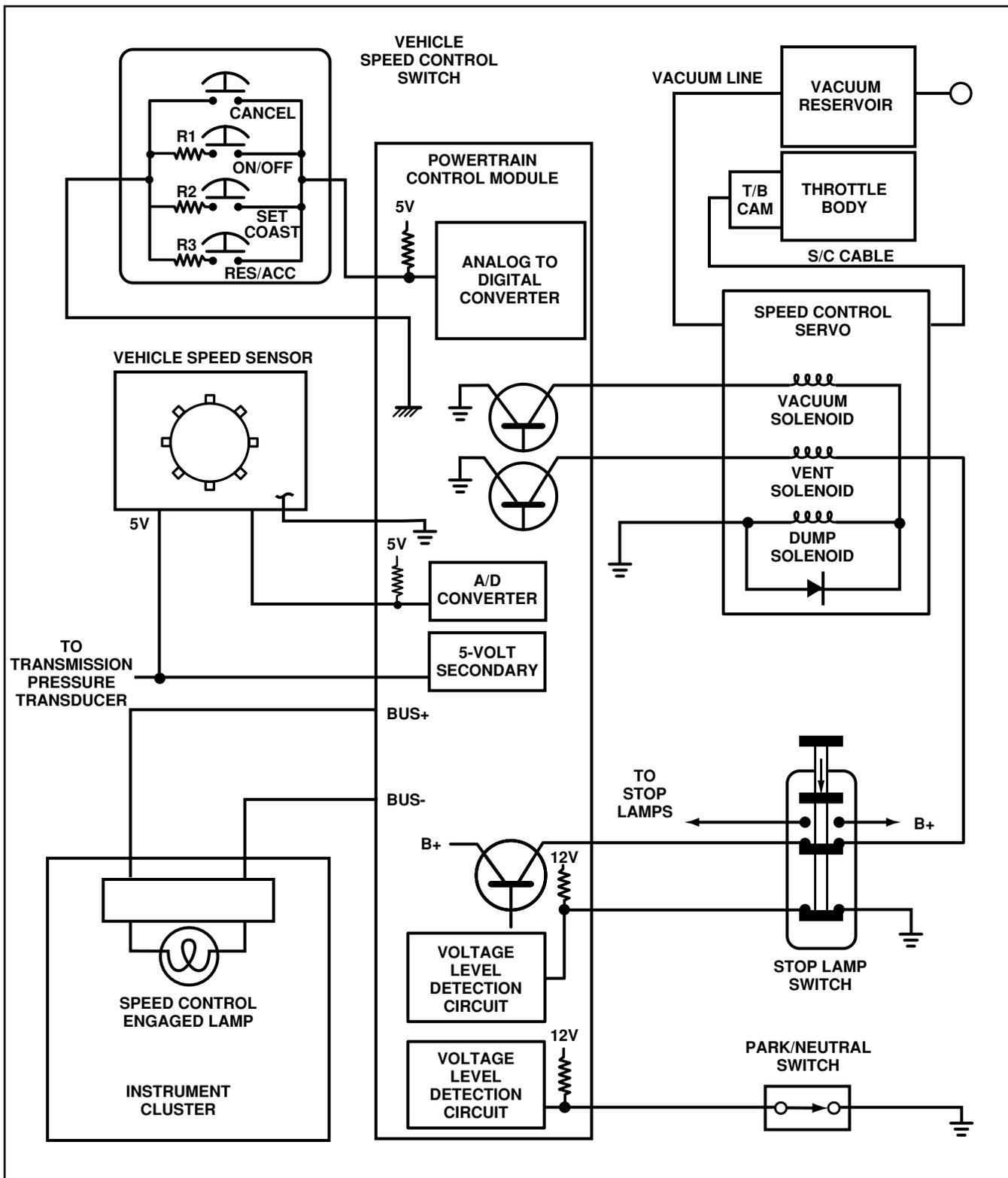
Figure 77 Typical Speed-Control System Circuit Schematic
