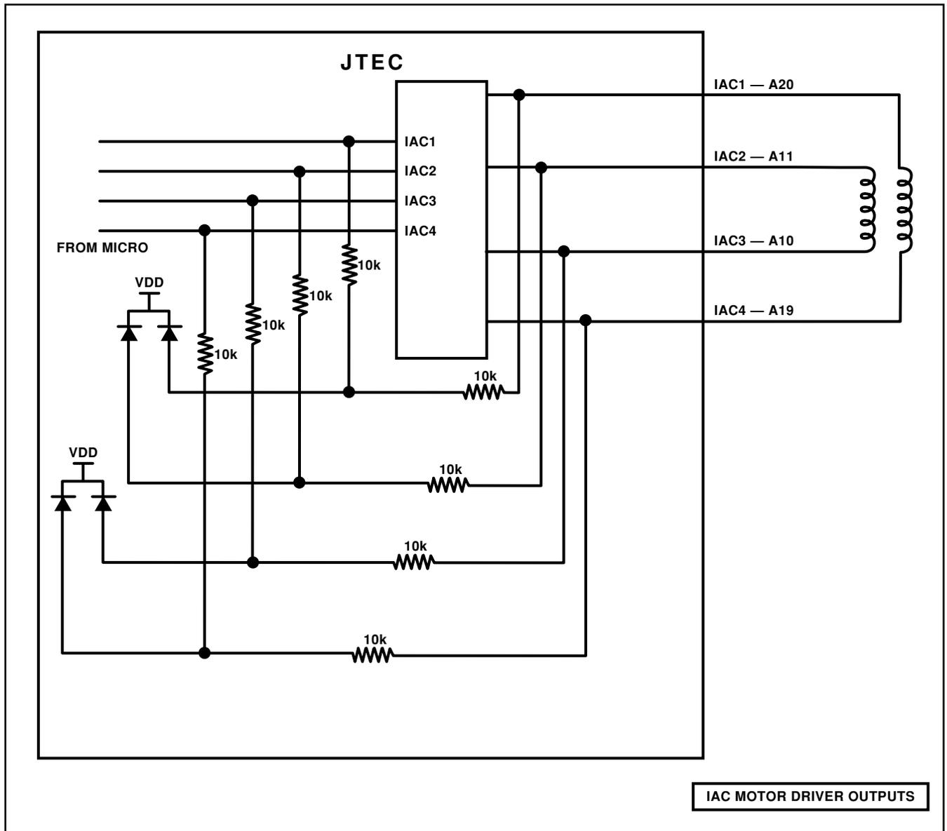
Figure 68 IAC Motor Control Circuit
