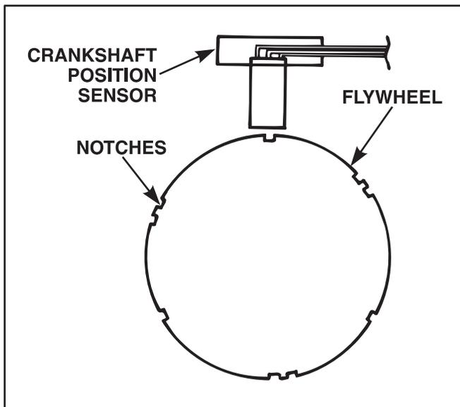
Figure 16 Sensor Operation —
