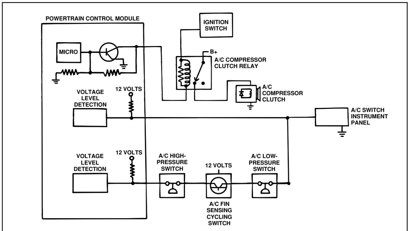
Figure 80 AB A/C Circuit
