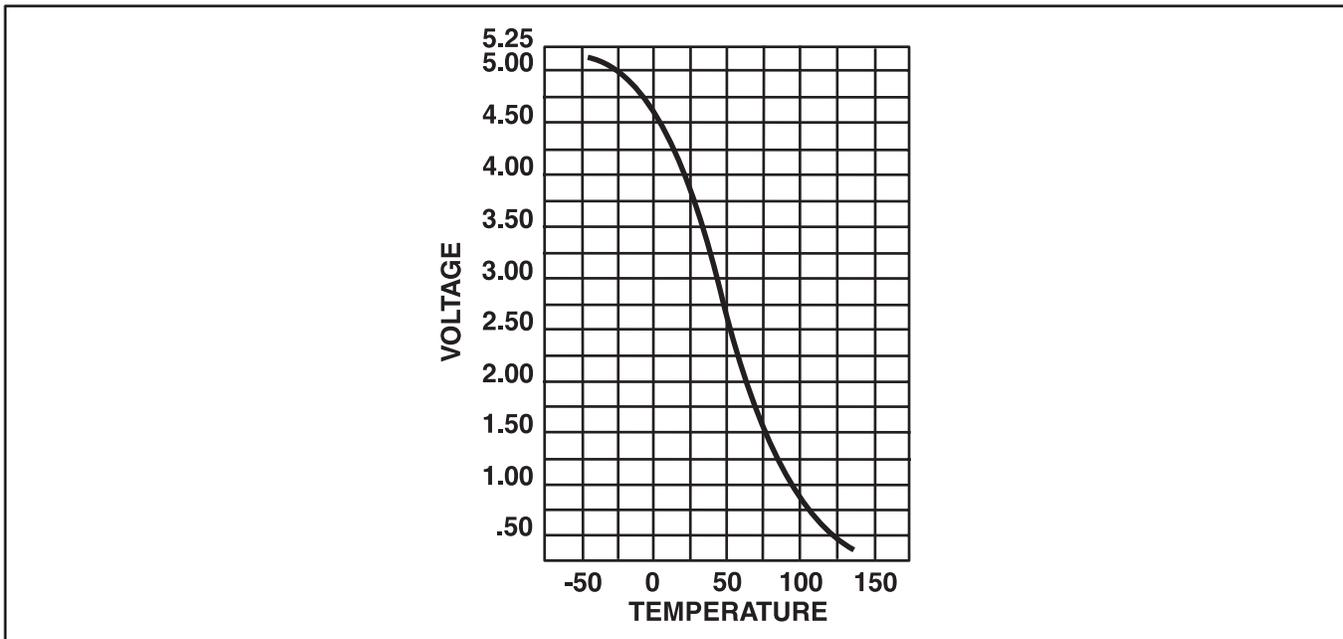
Figure 39 ECT/IAT Temperature/Voltage Curve
