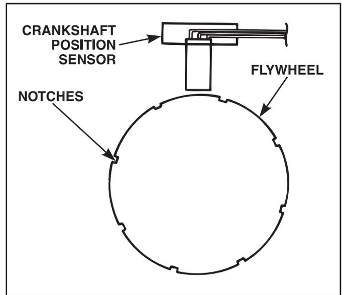
Figure 17 Sensor Operation —
