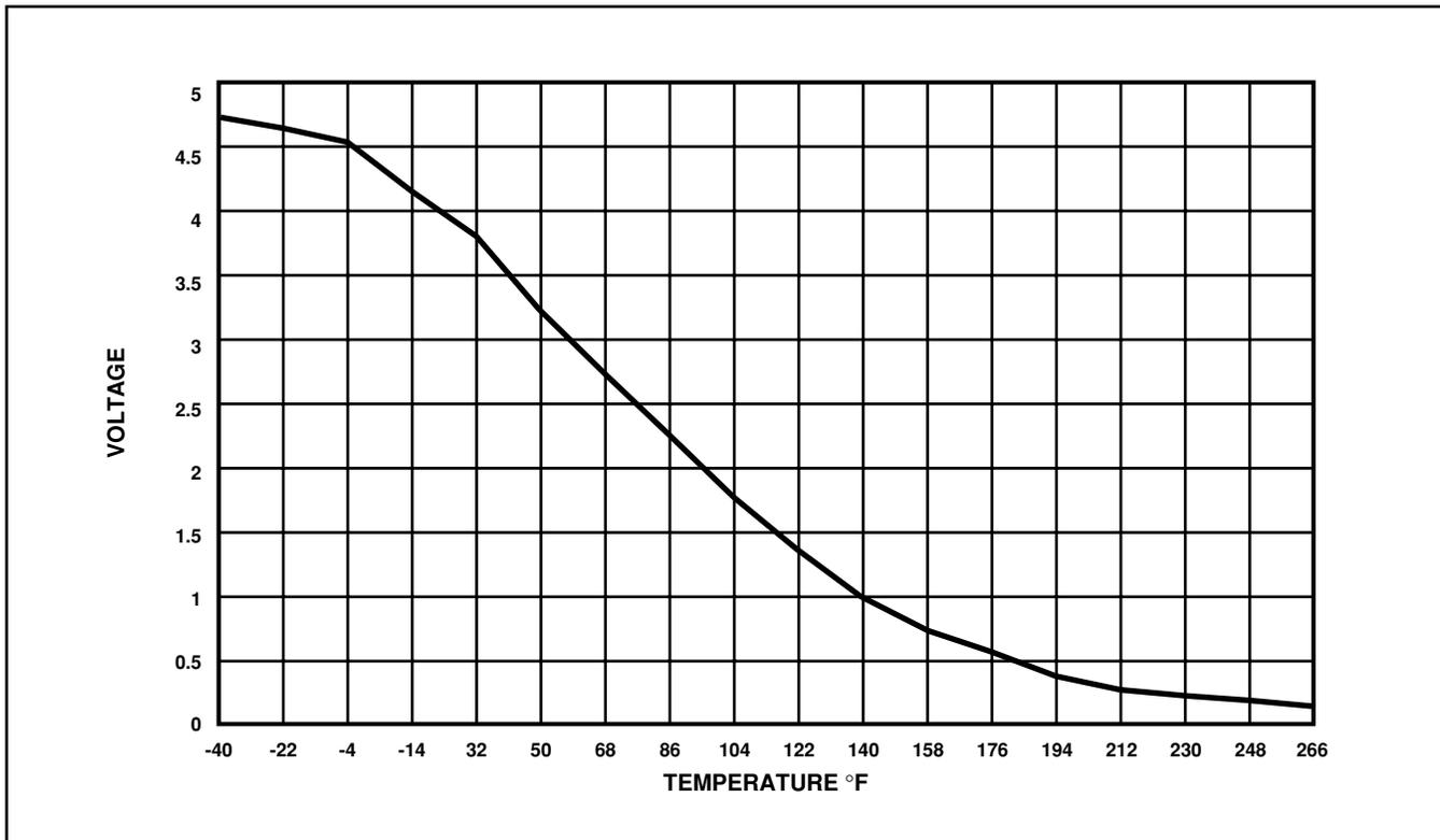
Figure 57 Battery Temperature Sensor — Temperature vs. Voltage
