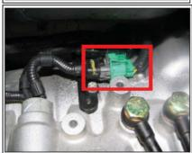
Peel back electrical harness conduit. Cut wire back on the harness side approximately 3 inches from terminal A6, blue corner wire.
