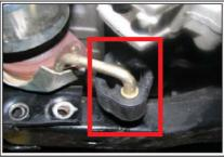
5. Disconnect the green transmission connector 'A' from the mounting bracket on the right side of Transmission.
