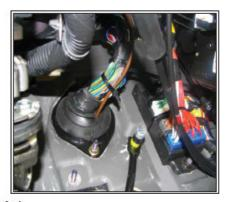
20. Locate the TCM on the left side under dash to the left of the brake pedal. The TCM can be identified as having 3 vertical electrical connectors (green, grey and white).
