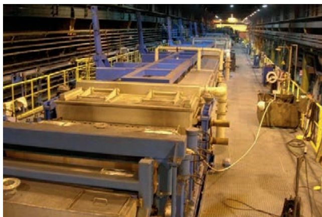
Figure 4:11. Mixed-acid pickling line.
