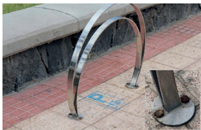
Figure 6:18. Bicycle parking on Tenerife, Canary Islands, 100 m from the Atlantic Ocean. Galvanic corrosion on galvanized bolts.
