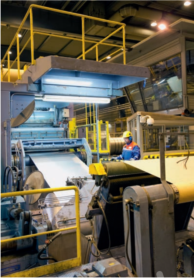
Figure 4:13. Skin pass mill at Outokumpu Tornio Works.
