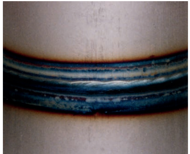
Figure 11:2. Weld with remaining weld oxide.
