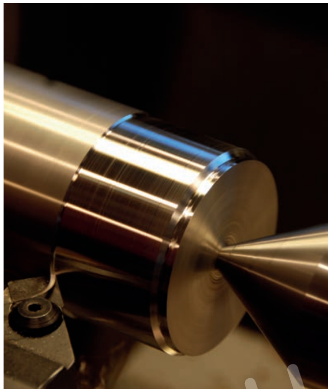
Figure 9:6. Duplex grade LDX 2101® shows excellent machinability.
