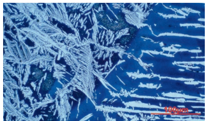
Figure 10:3. Duplex weldment. Weld metal left and HAZ right.
