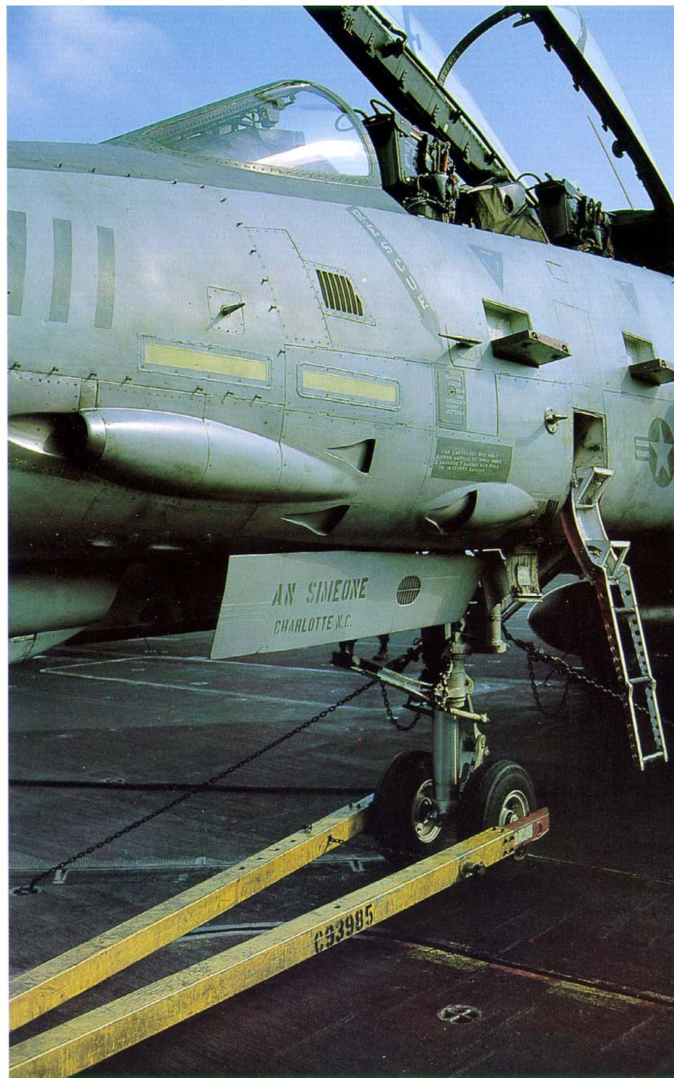
(Left) Left nose section detail with M-61 gun fairing up front. The front fairing is located over the multi-barrel assembly while the aft fairing clears the actual gun housing. Note the initial F-14 gun gas slots have been replaced by cooling air intake scoops. Also note interior canopy frame detail.
