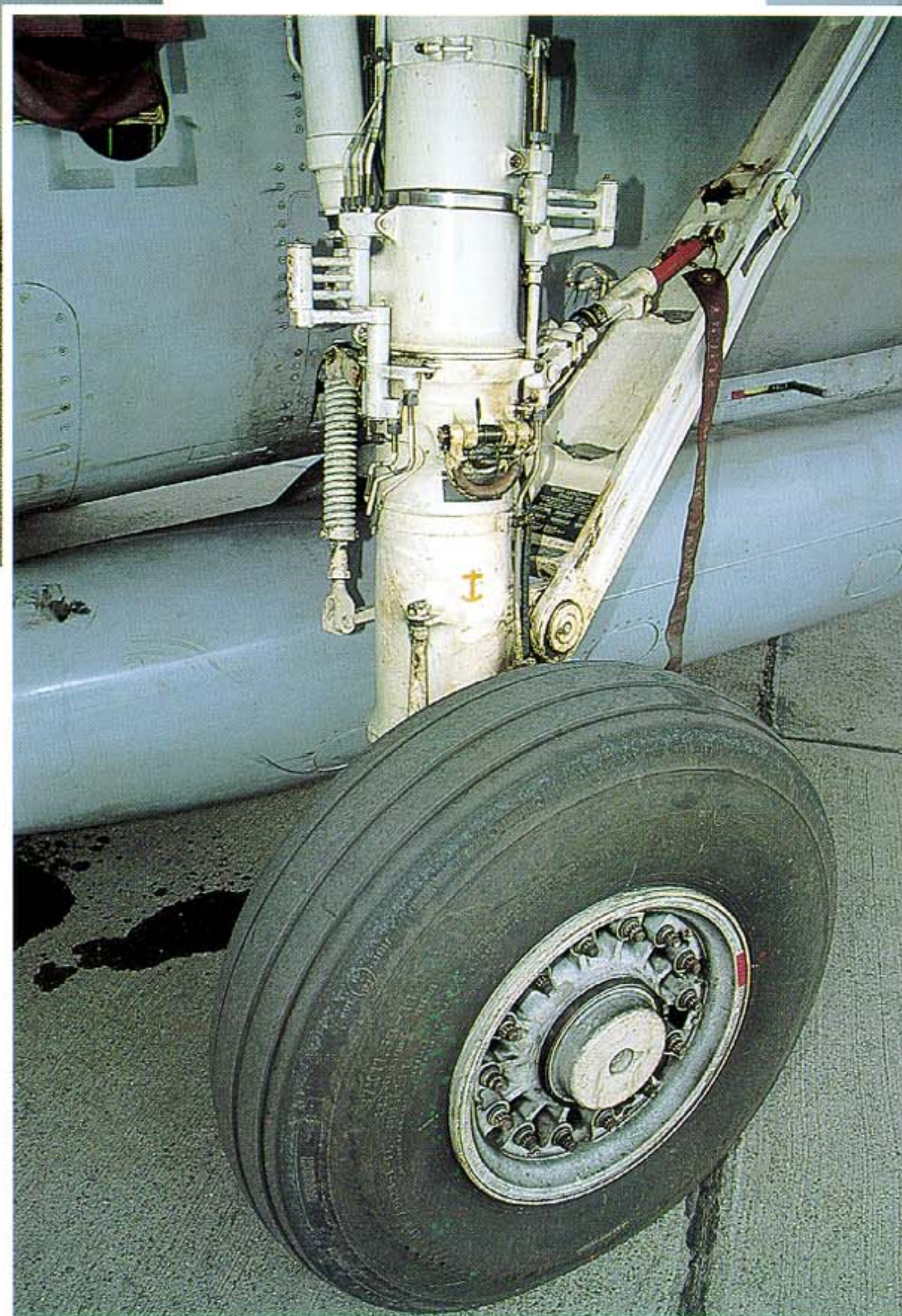
Massive main landing gear strut of conventional concept located aside the engine nacelles, designed to take the heavy punishment of deck landings. Note bottom left detail shot of the main gear locking bracket in the lower nacelle edge.
