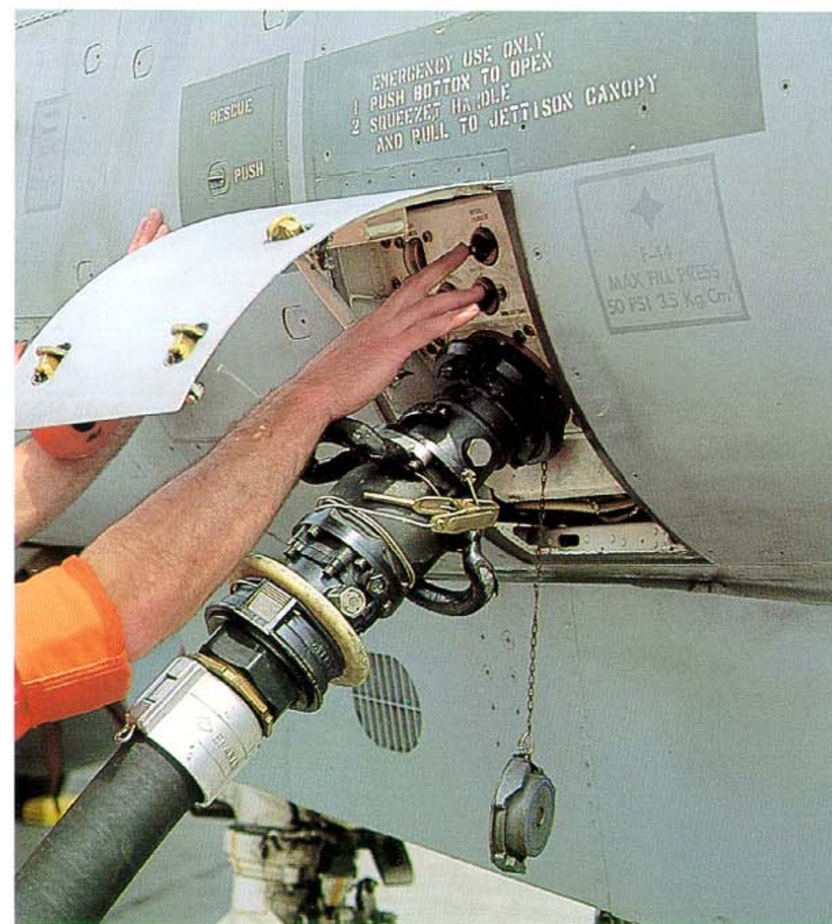
Ground refueling panel and control switches is located just above the nose gear well and in front of the rescue panel. Note the fuel servicing marking next to the panel.
