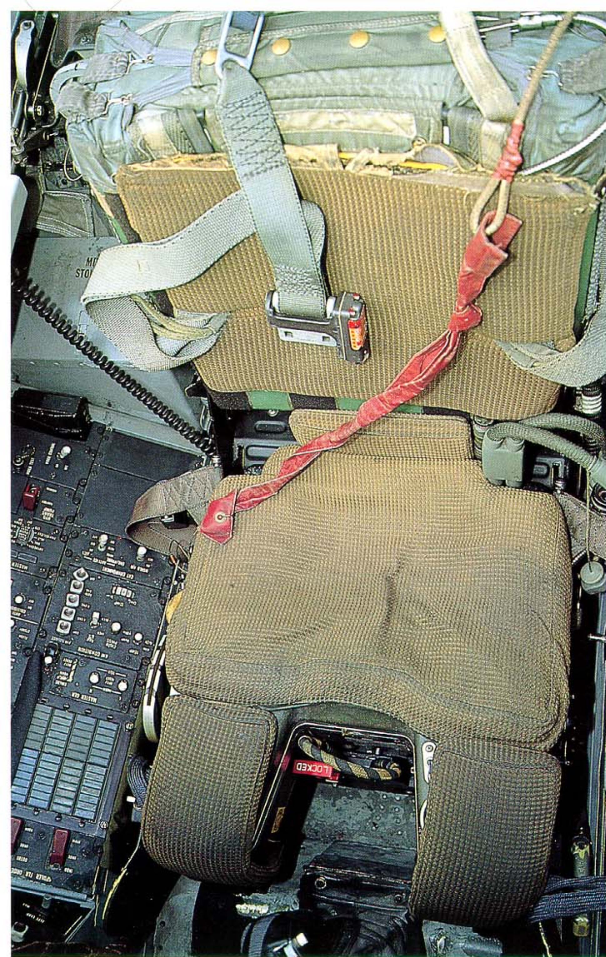
Reliable Martin Baker GRU-7 rocket propelled ejection seats guarantee both crewmembers a safe retreat from the aircraft in case of emergency. Dual activating handle on the headrest and single handle in front of the seat cushion (between the pilot's legs) provides eject options.
