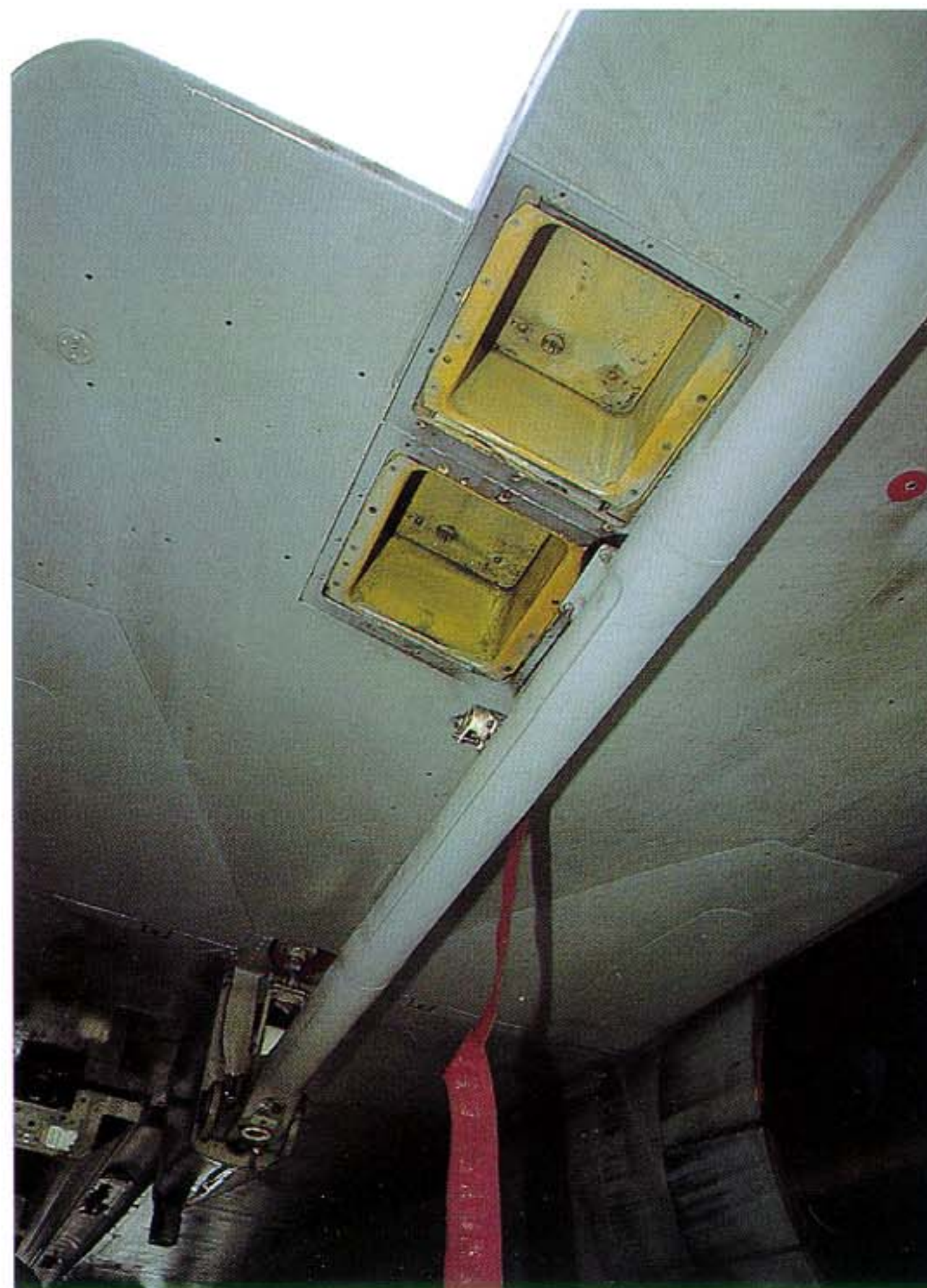
On the ground the arrestor hook is secured with a safety pin halfway up the bar. Just forward of it is a rubber block assembly blocking the hook inches from the bottom fuselage. Chaff/Flare dispenser is, again, not installed.
