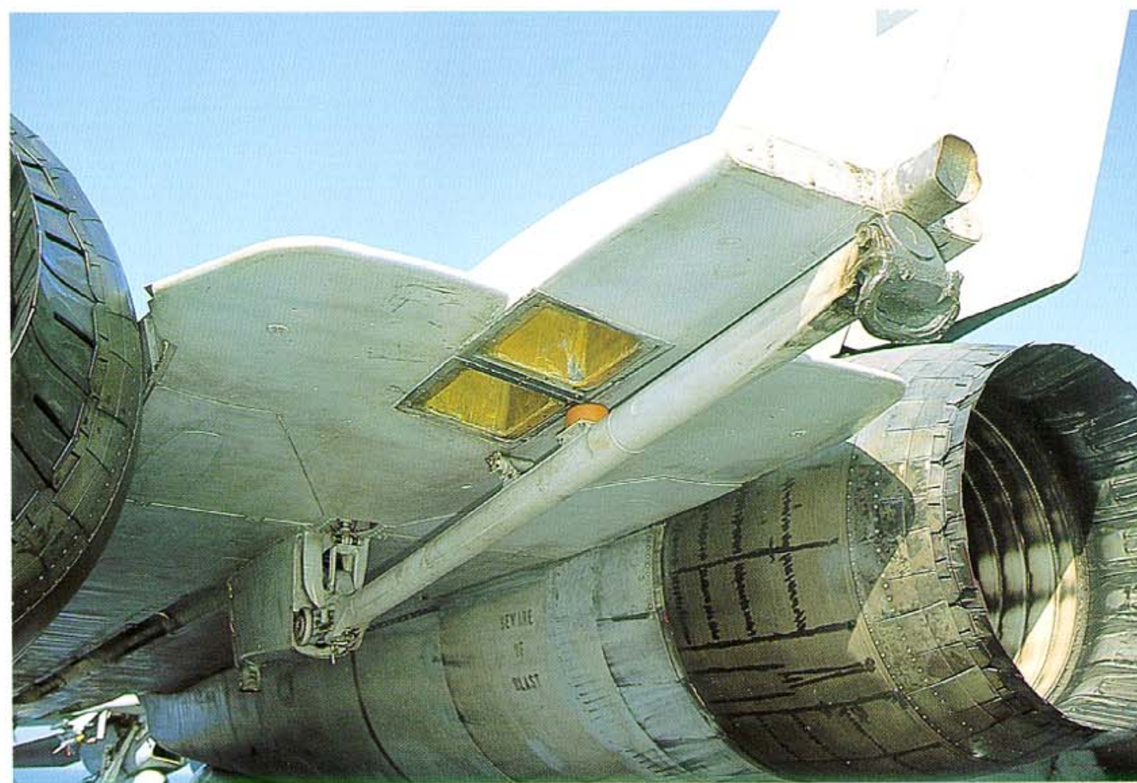
(Below) Arrestor hook/fuel dump assembly on fuselage empennage section. Chaff/Flare dispenser box is not installed.
