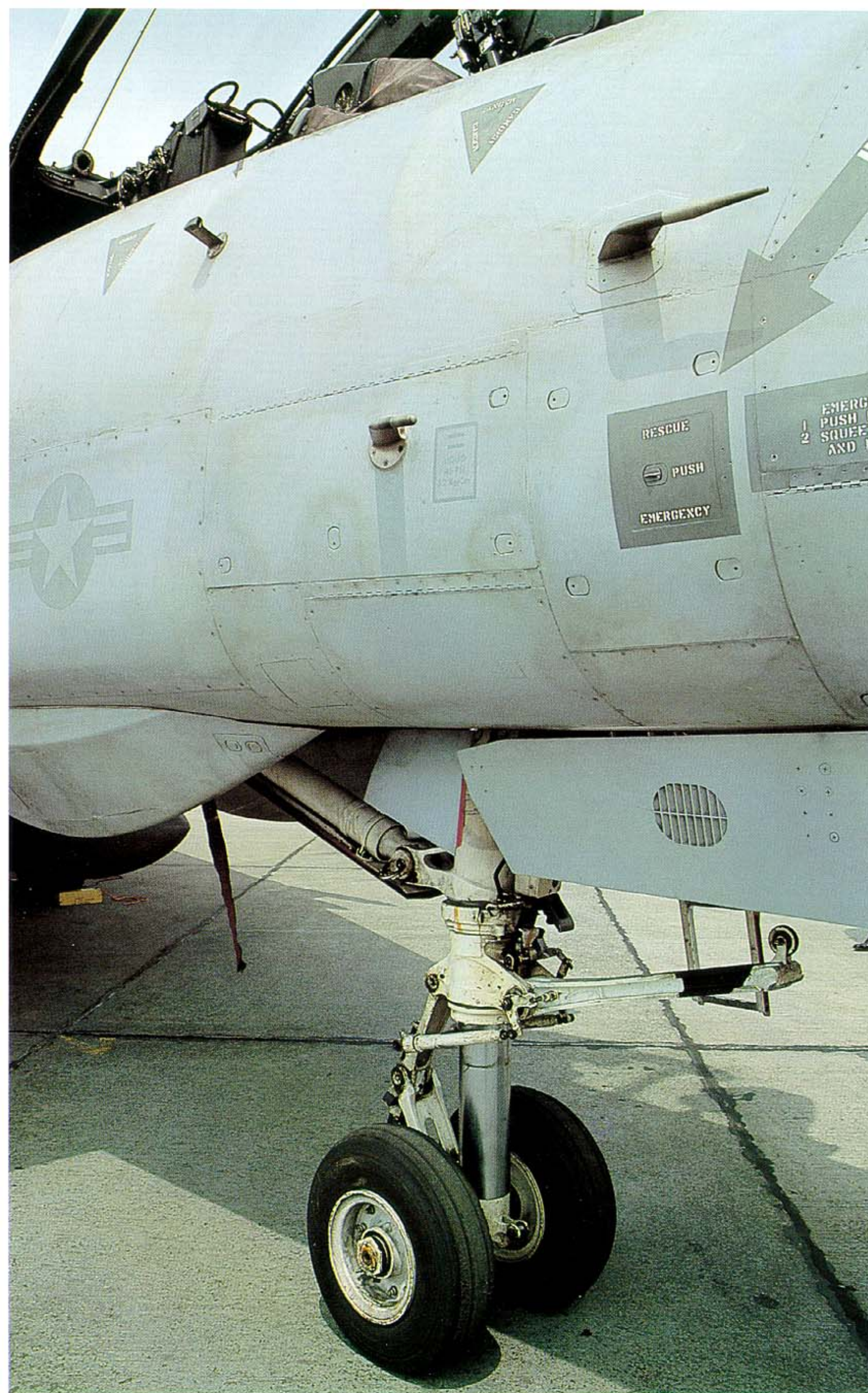
The larger panel aft of the rescue panel covers the liquid oxygen compartment, this one holding only one bottle although two are usually installed.
