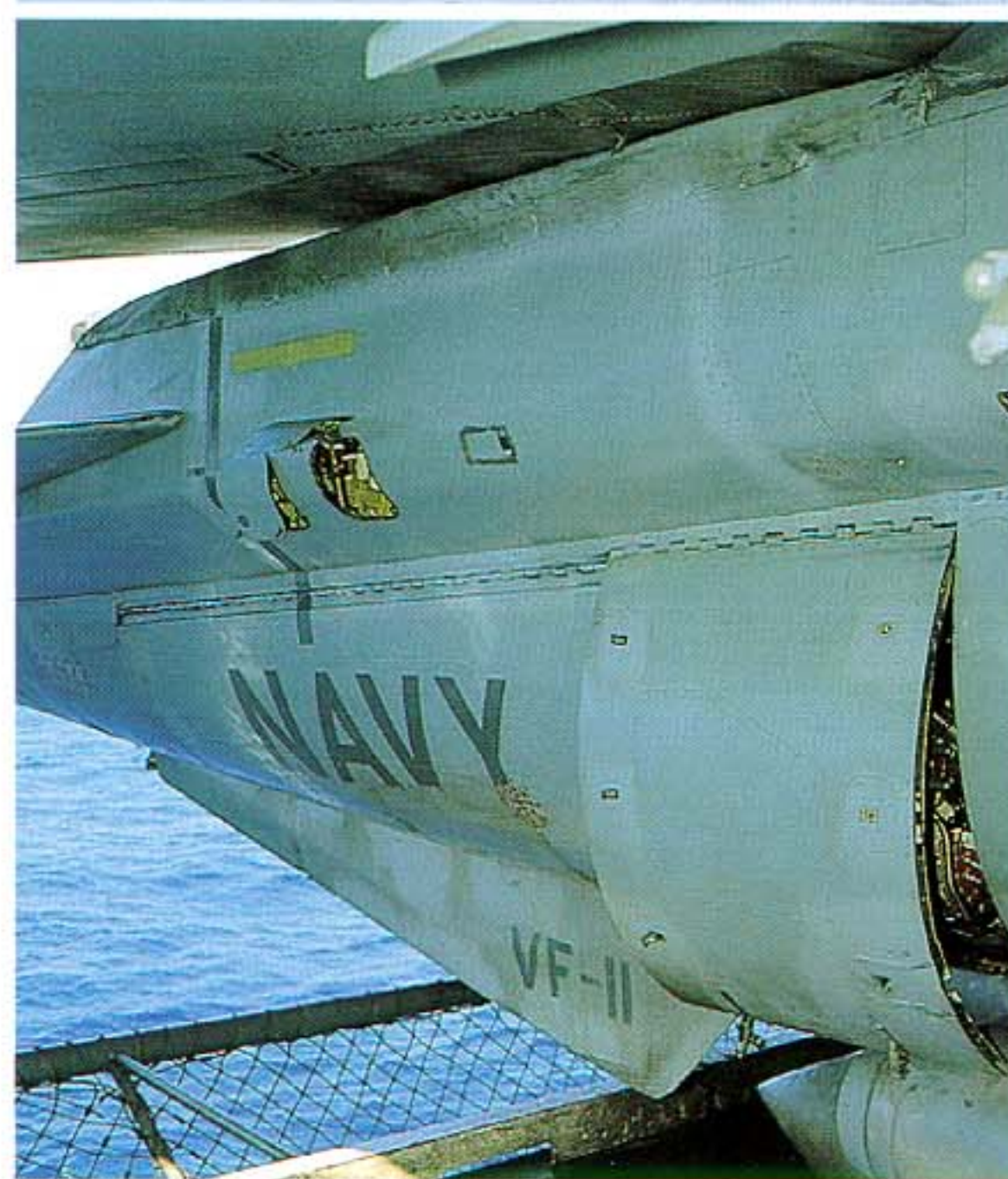
Partially opened inspection hatch of the engine compartment and some inspection panels on the bottom fuselage fairing. Note the discoloration on the partially retracted sweep wing.
