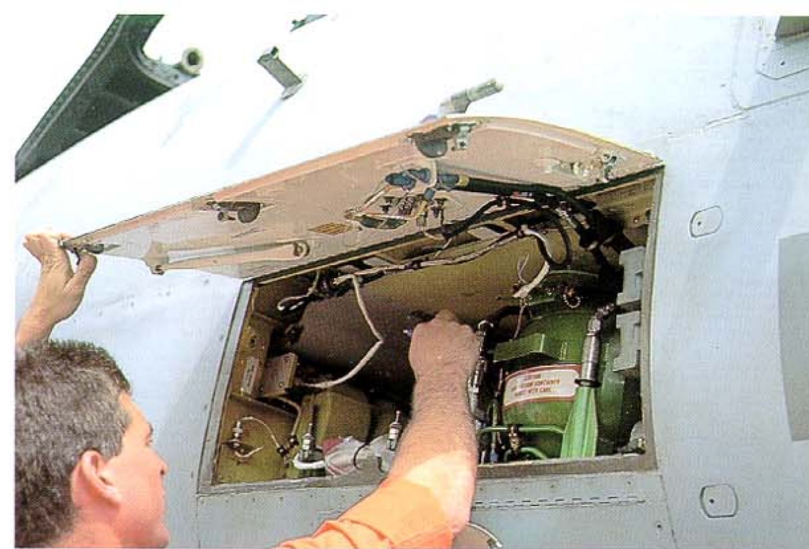
The larger panel aft of the rescue panel covers the liquid oxygen compartment, this one holding only one bottle although two are usually installed.
