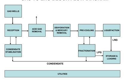
The chilling of the gas to moderately low temperatures causes at first the condensation of heavy hydrocarbons, which might also freeze and cause blockages of equipment at lower temperatures. These components of the gas are removed in a 'scrub' column along with some of the LPG (propane and butane) as the gas is cooled to about -35°C.
