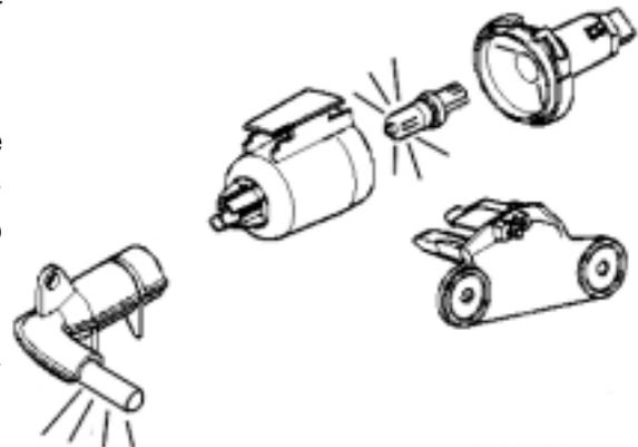
**Fiber Optic Light Conductor Cable:** The fiber optic cables carry the light to their respective light output modules at each exterior door handle.
