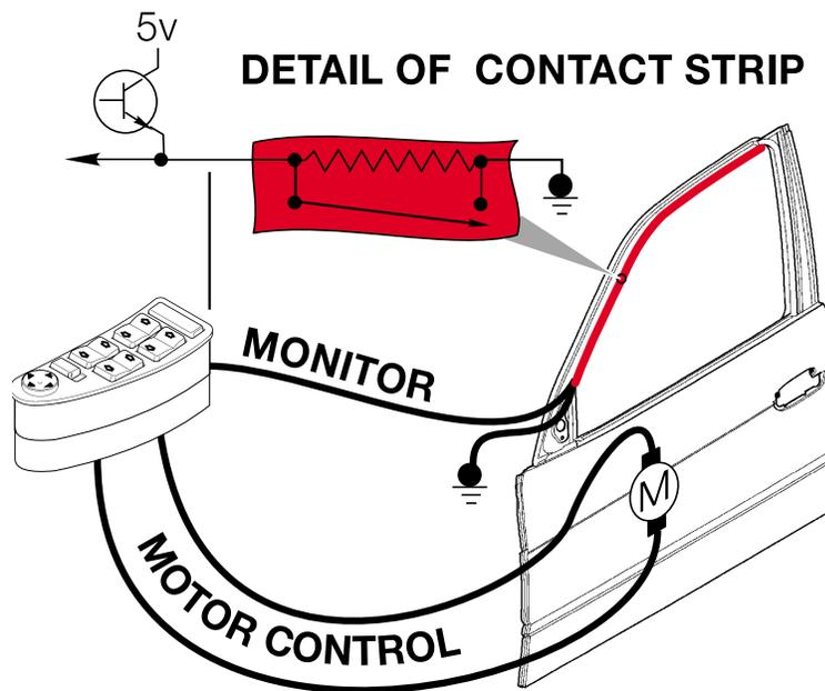
The example shown represents the driver's door window control and monitoring carried out by the Driver's Door Switchblock Module (PM- FT/ SB).
