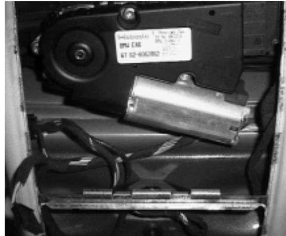
The electronic controls and relays are contained in the sunroof module (PM-SHD). The module is connected to the P-Bus (E38 >99 MY on the K-Bus) for comfort closing/opening and diagnosis/fault memory purposes.
