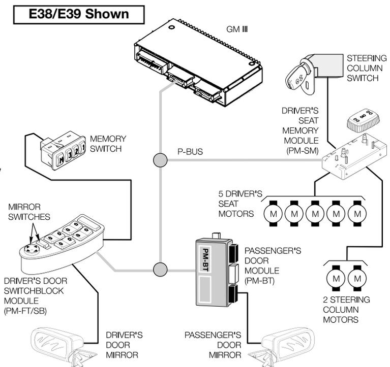
The Seat/Steering Column Memory Module communicates with the DISplus or MoDiC for diagnosis and Vehicle Memory encoding.
