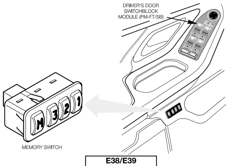
The positions of the mirrors are stored in the respective door modules based on the position of the feedback potentiometers. The positions of the seat and steering column are stored in the seat module, based on the ripple count.
