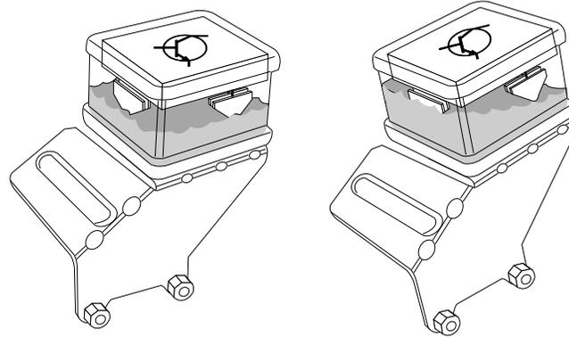
1. DWA ARMED, TILT SENSOR REGISTERS RESISTANCE VALUE THROUGH FLUID. SIGNAL HIGH TO GENERAL MODULE
