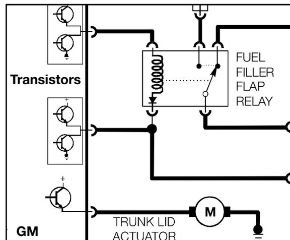
The ZKE III system offers an overall reduction in vehicle wiring particularly in the areas subject to wear from movement such as doors, seats and the steering column. To accomplish this, the “P- Bus” is used to interface (signaling) with peripheral modules over a single wire. The ZKE III modular system consisting of the following components:
