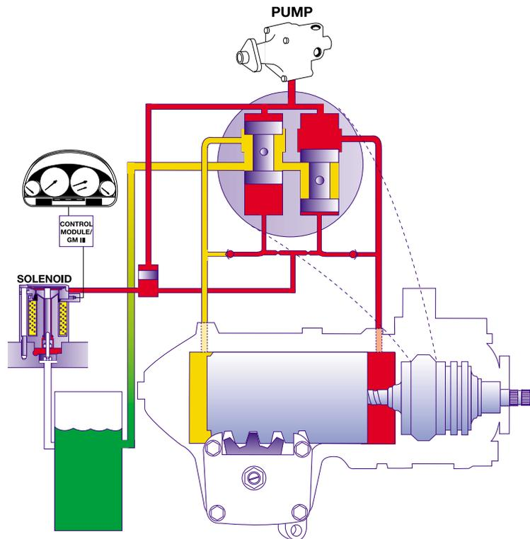
The "Direct Hydraulic Reaction" provided by the system allows the frictional forces between the front wheels and road surface to be transmitted to the driver. This allows the driver to make a better judgment in regard to the driving conditions.
