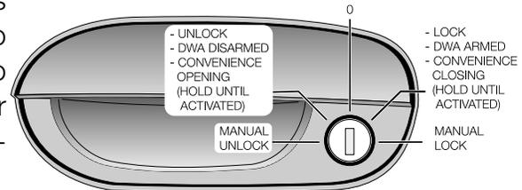
The windows and sunroof can be closed or opened by holding the key in the lock/unlock position (convenience closing/opening feature).
