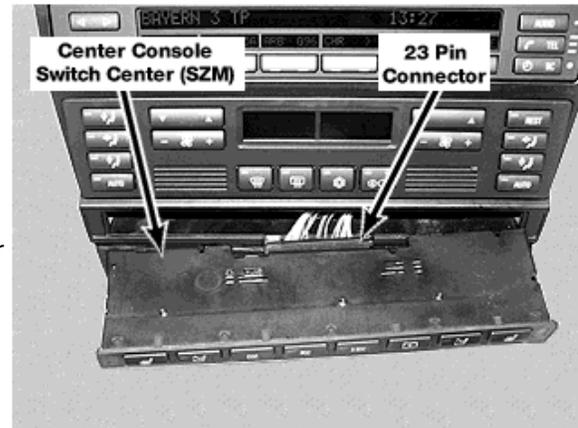
The switch signal output for these systems is a direct output signal. All diagnosis functions are carried out through their respective control systems.
