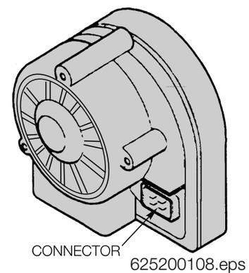
The siren has four wires connecting it to the system; KL 30, KL 31, activate siren signal (SIRENE) and the arm/disarm signal (STDWA).
