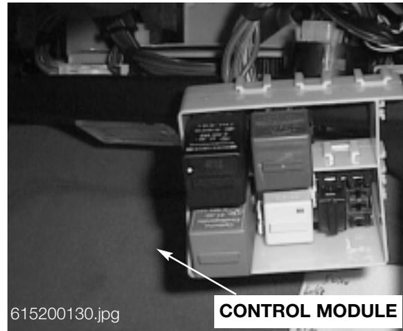
The GM controls the soft on/off feature of the vehicle interior lights by a pulse width modulated control signal. This signal is also an input to the Visual Entry Aid control module which requests simultaneously control (soft on/off) each exterior door light source.
