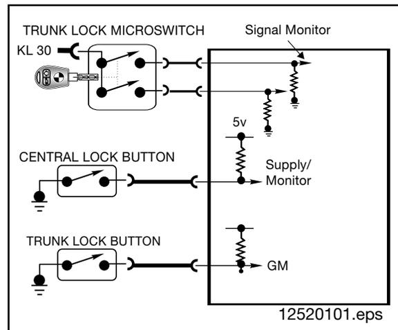
The GM **processes** the input information and contains “coded” instructions that allow a specific output control of functions.
