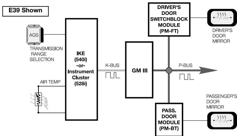
The memory positions are stored in each respective module. The memory position is recognized by the feedback potentiometers located on each mirror motor.
