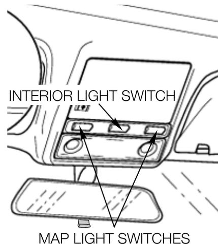
There are two reading/map lights also located in the assembly. Each map light is mechanically controlled by depressing the corresponding on/off switch. The power supply for the map lights is supplied by the GM through the Consumer Cut Off circuit.
