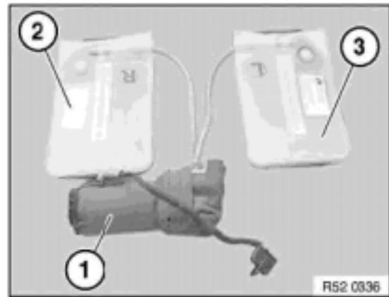
**Note:** *The pump unit and fluid bladders are replaced as a unit.*
