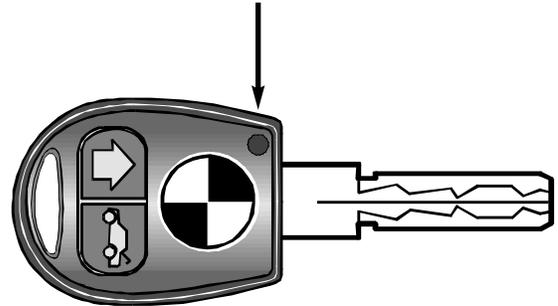
**FZV Key Test:** Pressing the trunk release and lock buttons together activates the key test. If the battery and FZV key EEPROM are “OK”, the LED will come ON for approximately 1 second.
