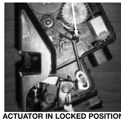
**Door Contact Hall Sensor:** Also included in the drivers door actuator is a third hall effect sensor. This sensor signals the door open/closed status to the GM. This sensor replaces the door jamb mechanical switch of previous systems. The rotary latch plate position activates the door contact hall sensor.
