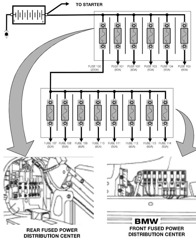
The X5 utilizes a single high amperage fused power distribution center located next to the left side EHC air reservoir beneath the cargo area floor paneling.
