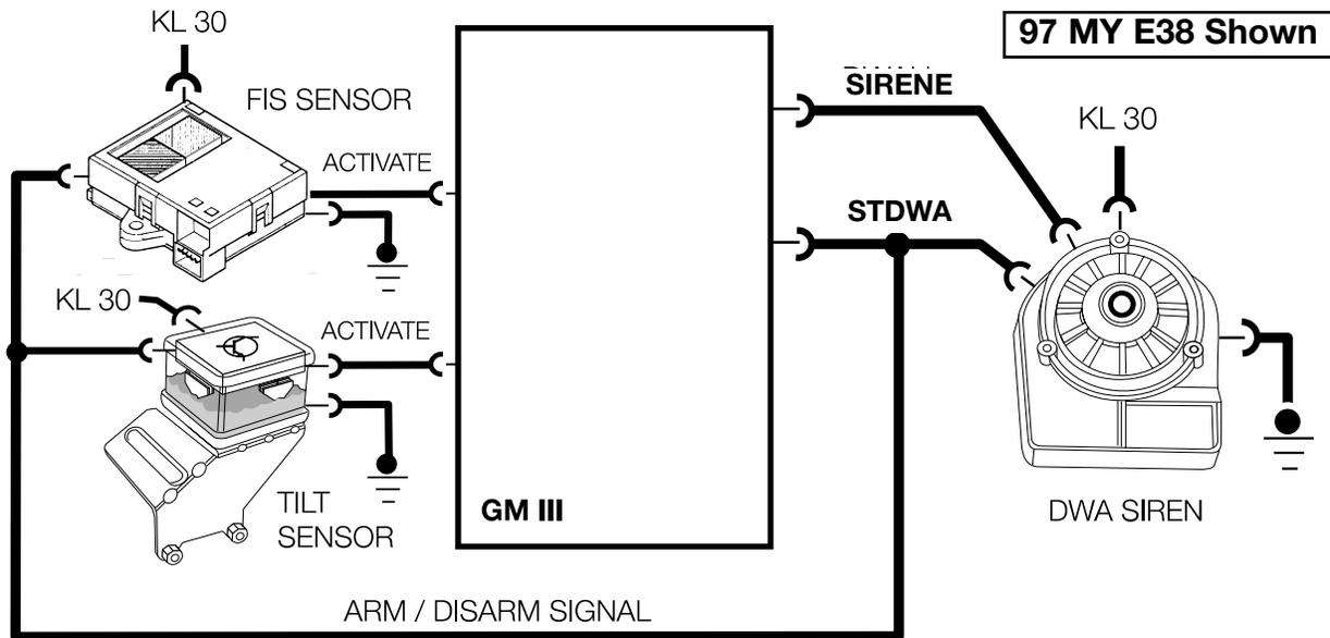
The activate siren signal to the siren is high whether DWA is armed or disarmed. If a monitored input activates the alarm, the high signal to the siren is switched to a 50% duty cycle at the GM. The control circuitry in the siren activates the siren driver.
