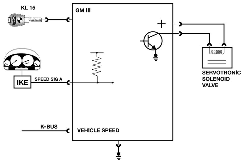
The solenoid is pulse width modulated for control and varies the amount of assist based on the road speed. The maximum assist is available while parking and driving at slow speeds.
