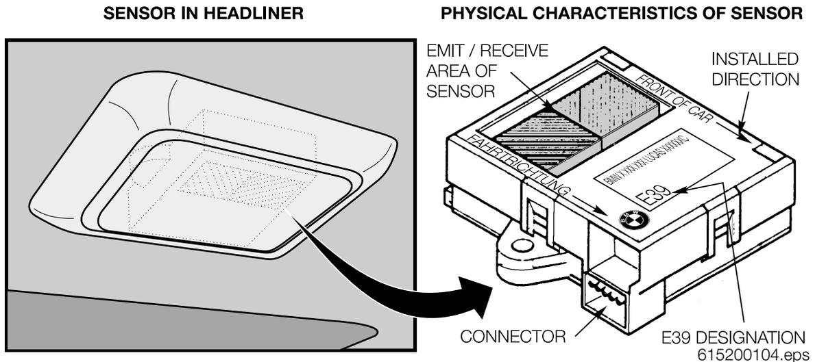
When the alarm system is armed, the sensor emits electromagnetic waves at a frequency of 2.45 GHz. As long as nothing is moving in the vehicle, the waves are bounced back to the sensor at the same frequency. The sensor monitors these bounced back waves as an indication that nothing is disturbed within the vehicle.
