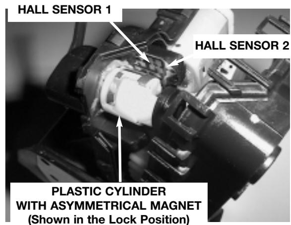
There are two motors incorporated in each actuator that provide two separate functions:
