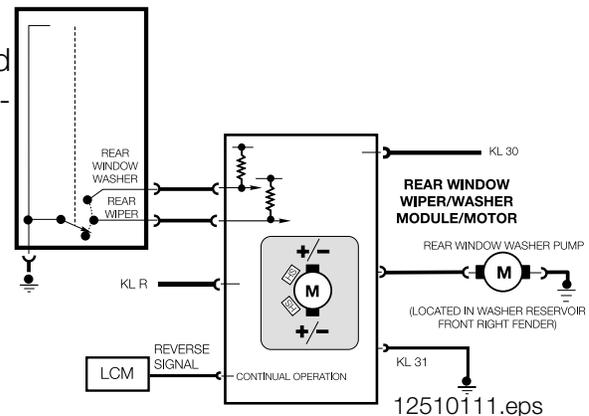
**Pressing the wiper stalk forward to the first detent activates the rear wiper in the intermittent mode.** The timed interval is approximately 7-12 seconds. The full sweep and park positions are recognized by the two hall sensors on the motor gear assembly. If the wiper is switched OFF, the wiper blade will return to the park position.
