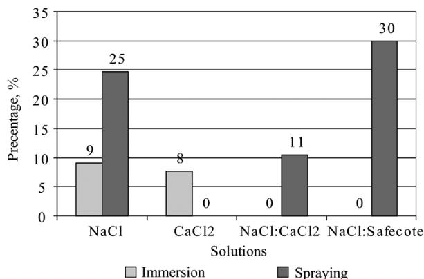
**Fig. 5.** Percentage rate of galvanized steel corrosion product cover by immersion and spraying methods
