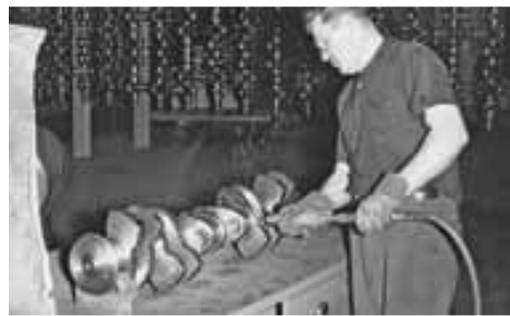
During the 1960s and 1970s, crankshafts were deburred by hand at individual deburr benches.
