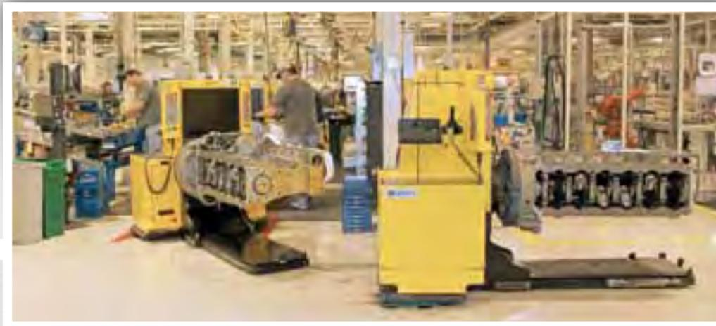
Since 2006, AGV units have replaced slat conveyors, giving assemblers far more freedom to move cylinder blocks into the optimal work position quickly and comfortably.
