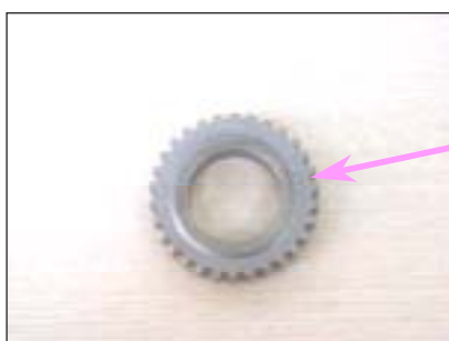
Sensing tone wheel for rear speed (teeth = 30EA) Location : The end of rear propeller shaft
