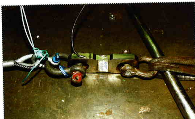
Pulling force is measured within this load cell device...
