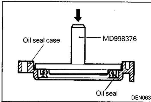
**◆D◆ INSTALLATION OF OIL SEAL**
