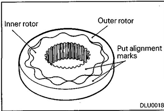
**REMOVAL OF OUTER ROTOR / INNER ROTOR / OUTER GEAR / INNER GEAR**
