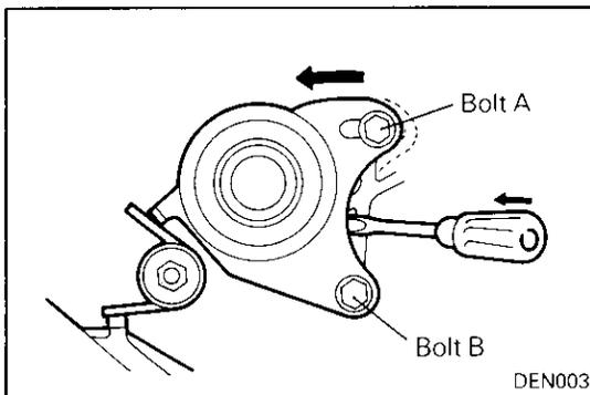
**◆F◆ INSTALLATION OF TIMING BELT TENSIONER**
