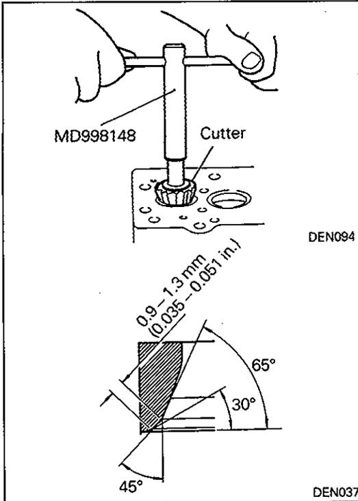
**VALVE SEAT RECONDITIONING PROCEDURE**
