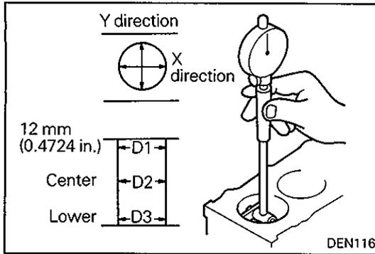
(3) To measure the tightening allowance, measure both the cylinder sleeve O.D. and cylinder block sleeve hole I.D. at the position illustrated.
