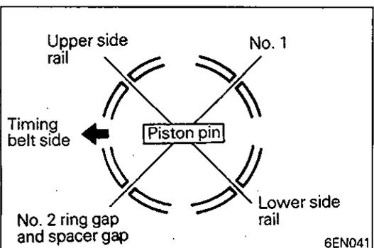
**◆C◆ INSTALLATION OF PISTON AND CONNECTING ROD ASSEMBLY**
