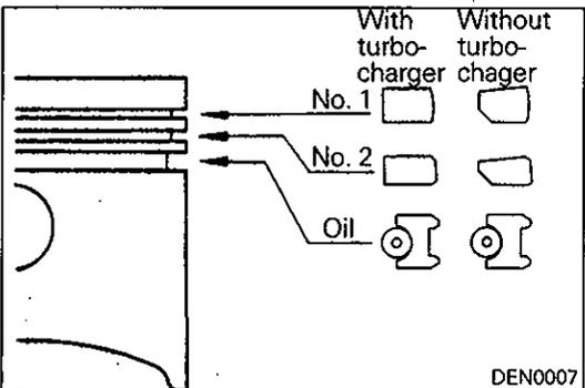
**◆B◆ INSTALLATION OF PISTON RING NO. 1 / PISTON RING NO. 2 / OIL RING**
