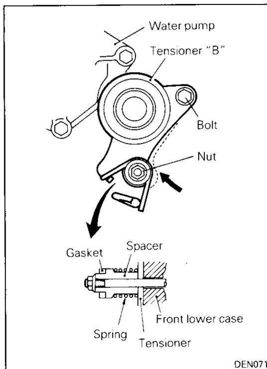
**◆D◆ INSTALLATION OF TIMING BELT TENSIONER "B"**
