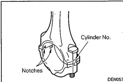
**◆D◆ INSTALLATION OF CONNECTING ROD CAP**
