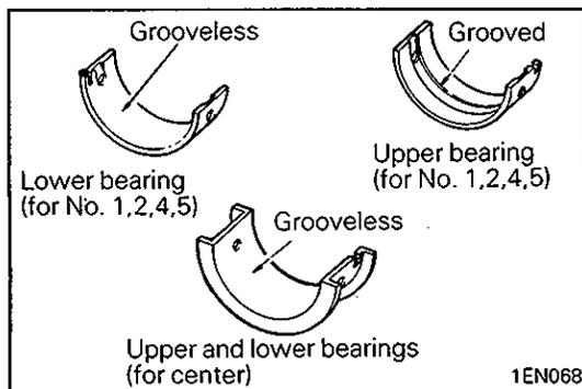
**SERVICE POINTS OF INSTALLATION****◆A◆ INSTALLATION OF CRANKSHAFT BEARING (UPPER)**
