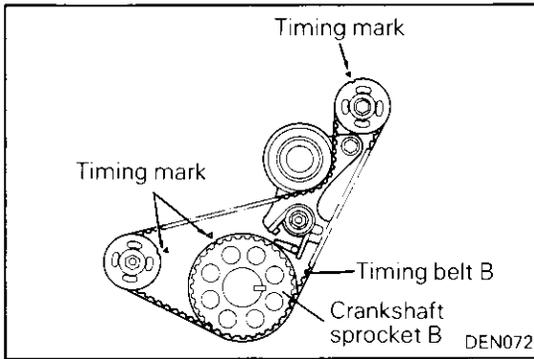
**◆E◆ INSTALLATION OF TIMING BELT "B"**
