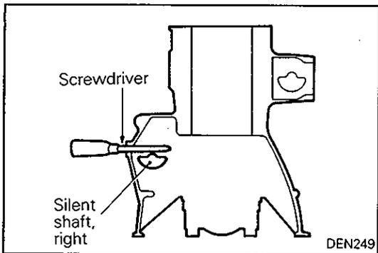
**◊C◊ REMOVAL OF SILENT SHAFT BEARING**
