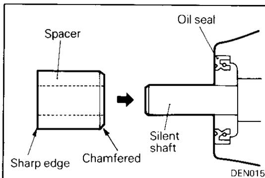
**◆B◆ INSTALLATION OF SPACER**
