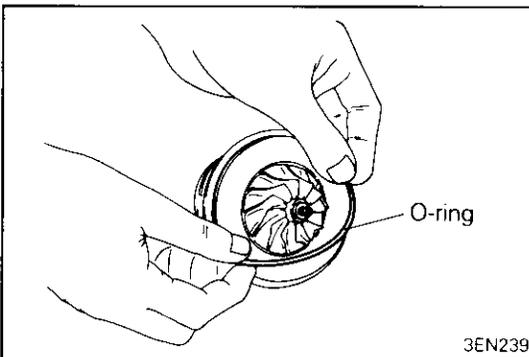
**◆B◆ INSTALLATION OF TURBINE WHEEL ASSEMBLY**
