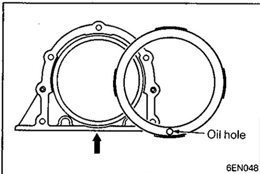
**◆E◆ INSTALLATION OF OIL SEPARATOR**
