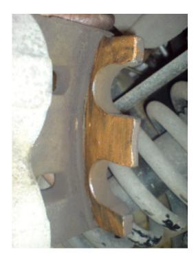
Put also a some grease on the other side of the caliper.
