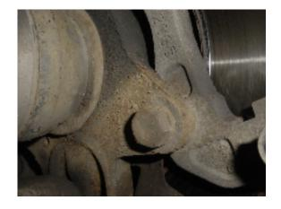
Then remove the bolts of the brackets.
