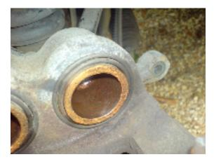
Then put a small amount of cupper grease in the caliper edge.
