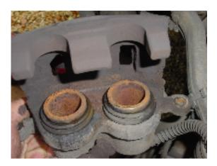
There is some rust inside the pistons. I removed it with a cupper brush.
