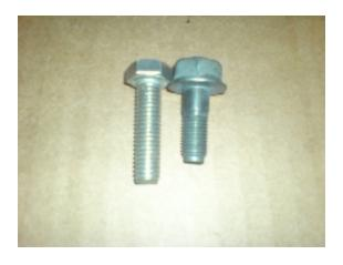
Here you see to the right one of the bolts that holds the caliper. You can see it has a finer treat so don't use a regular bolt when you lose one.
