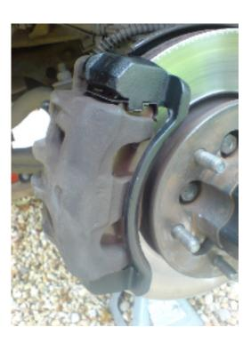
Put the caliper in place and tight the two 8 mm bolts with the right torque.
