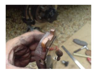
Put on a small amount of cupper grease on both ends of the pads.
