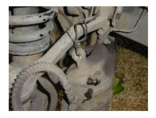
Then hang up the caliper on the wishbone.
