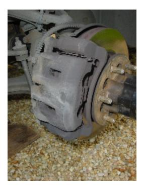
Here you see the front brake before I started. By the models 2004> a 2 pistons system is mounted.
