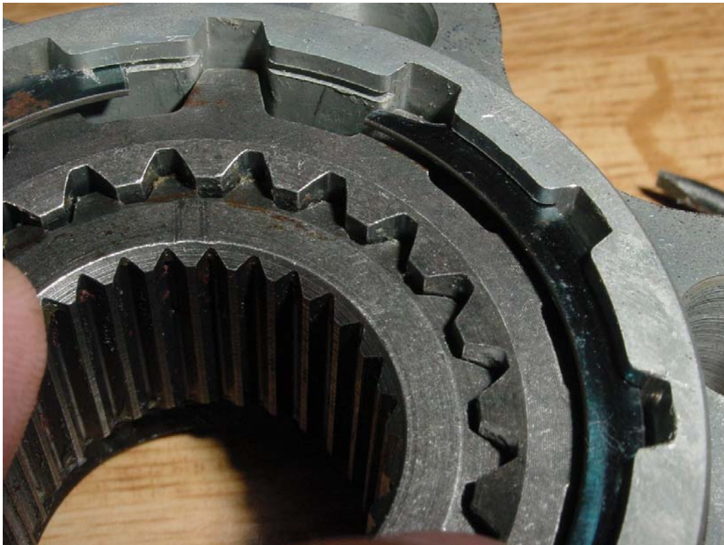
Retainer ring in place.
