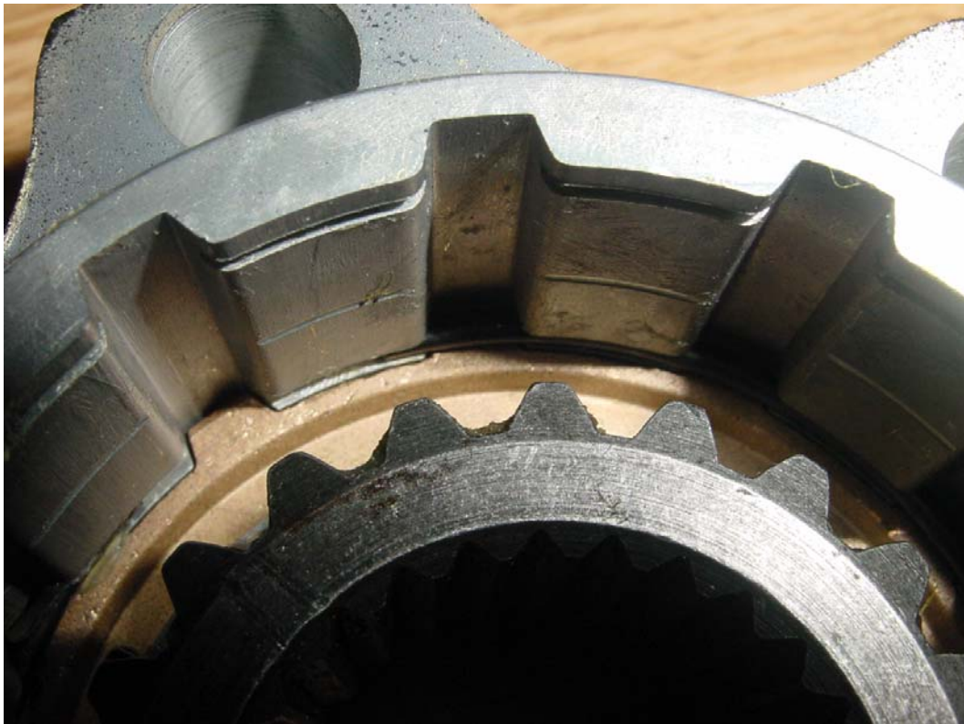
Retainer ring in place.
