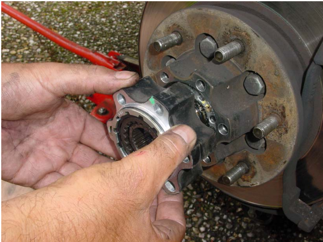
Pull vacuum hub body from axle hub.
