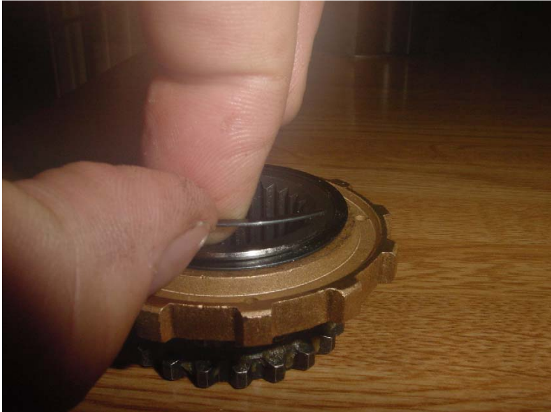
Inner Drive Gear and bearing locked by retainer ring.
