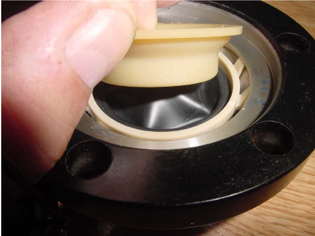
Under the Diaphragm Retainer sits the vacuum Diaphragm.
