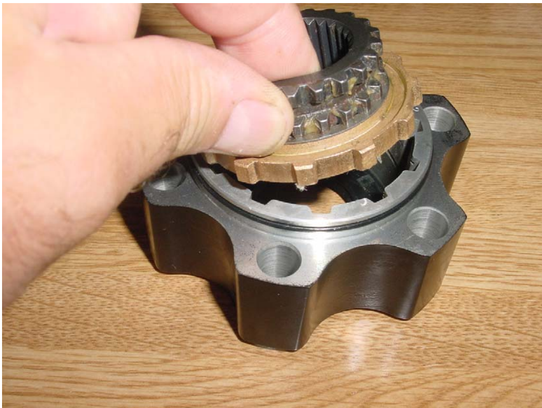
Place Inner Drive Gear and bearing in body.
