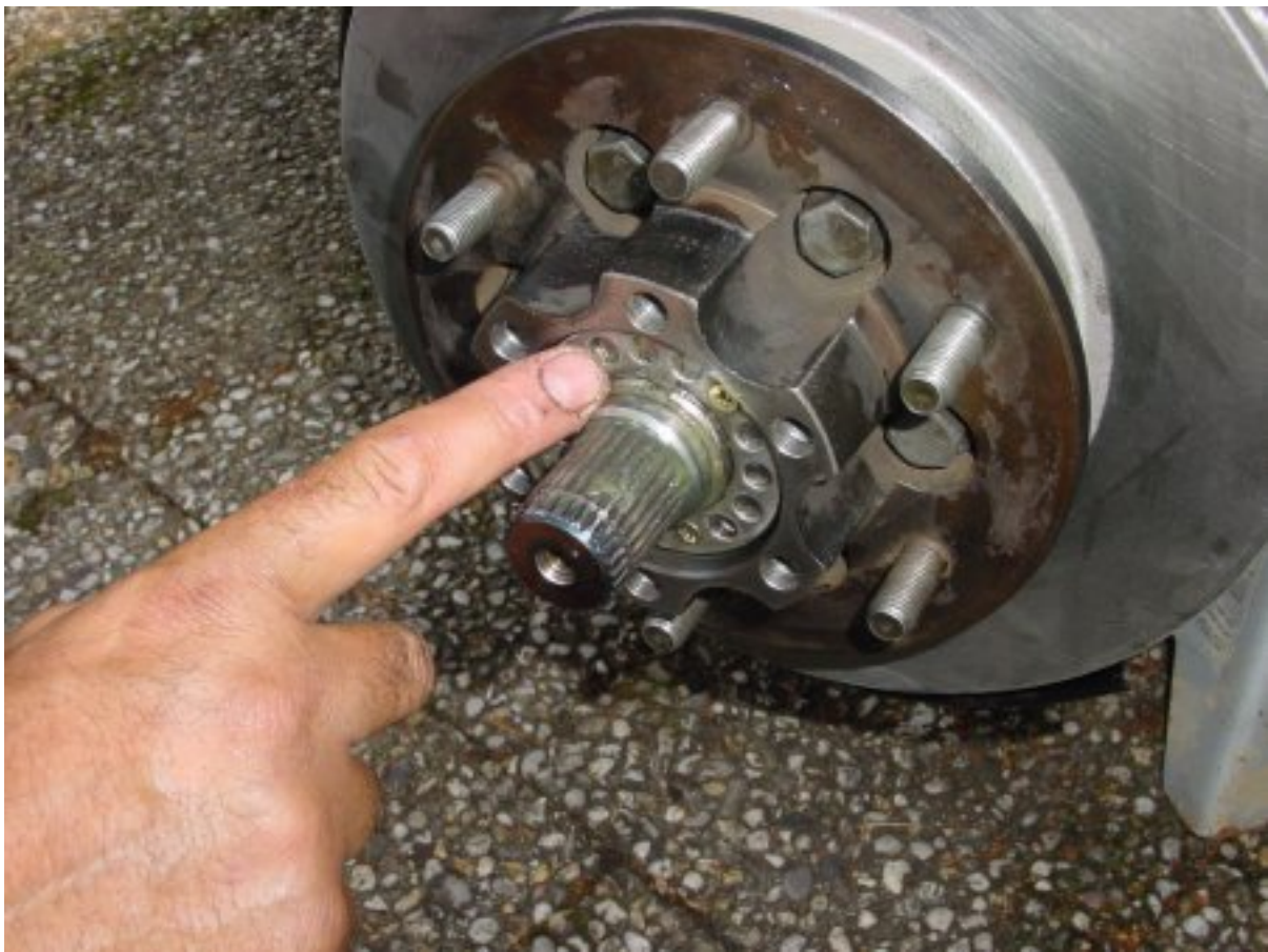
Replace the hub on the axle. Put the outer bearing in. Screw the nut on till the mark of the centre point is on his place. Check the hub on play. If yes tighten the nut a bit till the play is out. Replace the locking plate with the three screws. Torques see manual.
