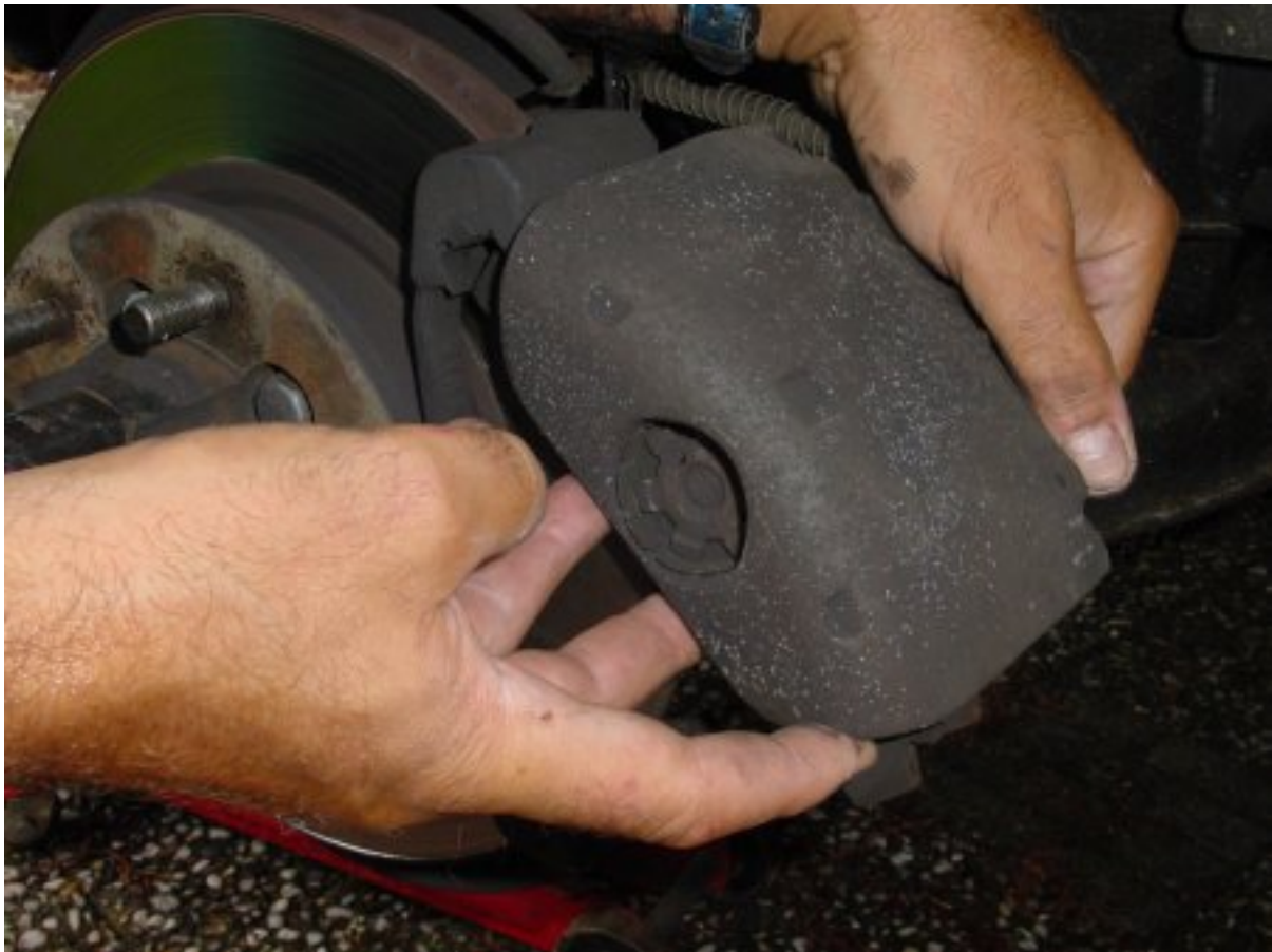
Rotate the calliper housing whit pads of.
