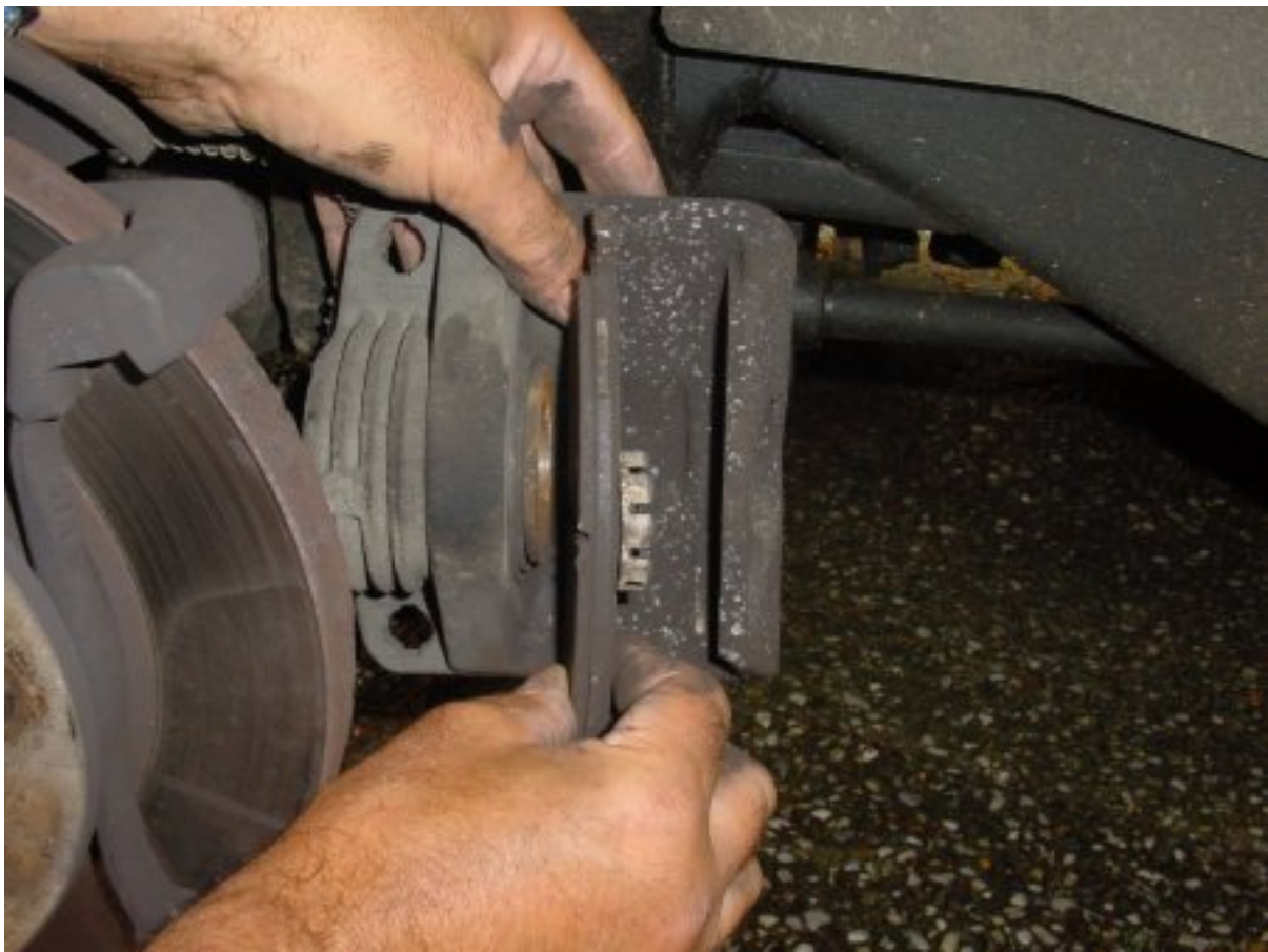
Remove the outer pad of the calliper.
