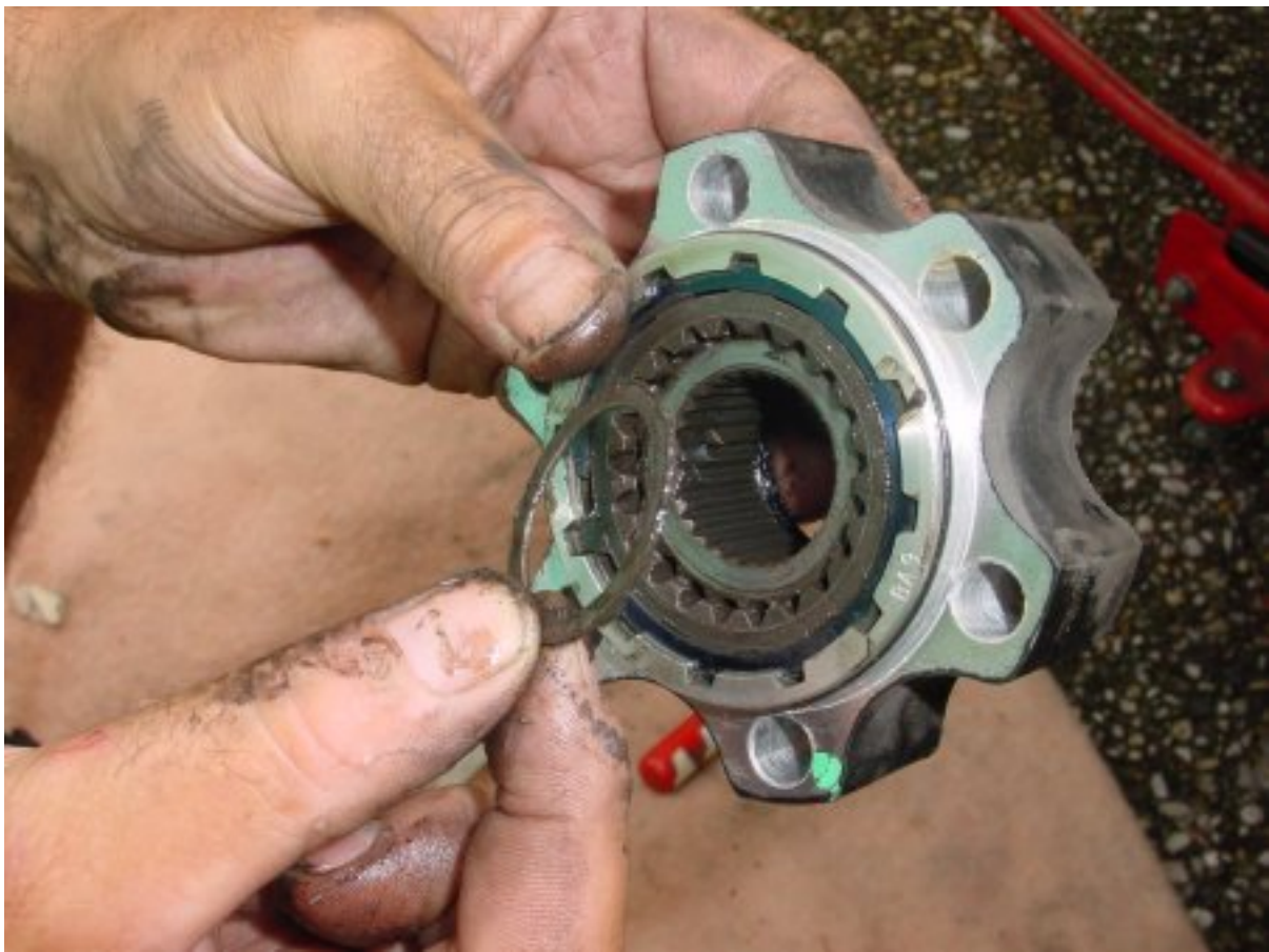
Between the retainer ring and the hub inner part sits one or more shims.
