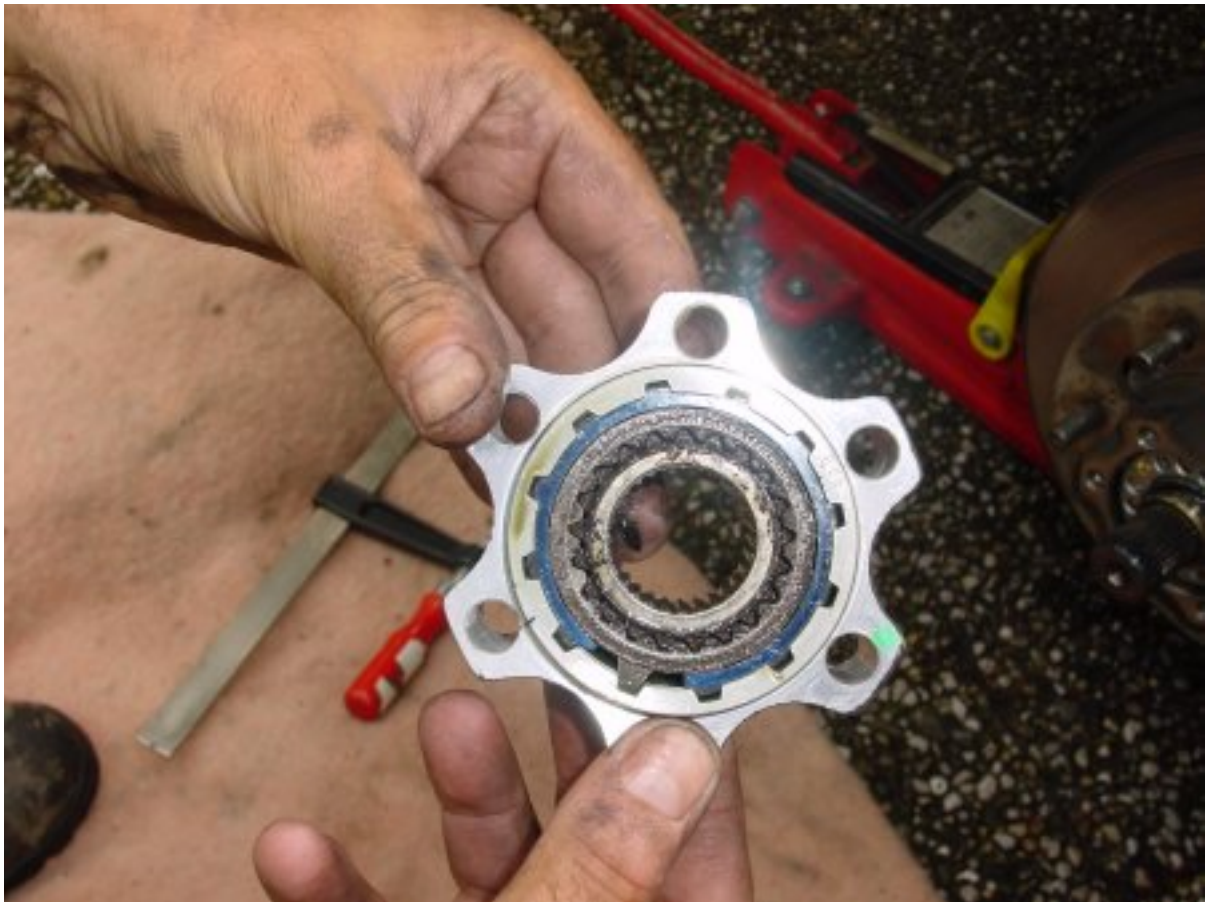
View on the front side of the hub. The bleu part is a locking spring.
